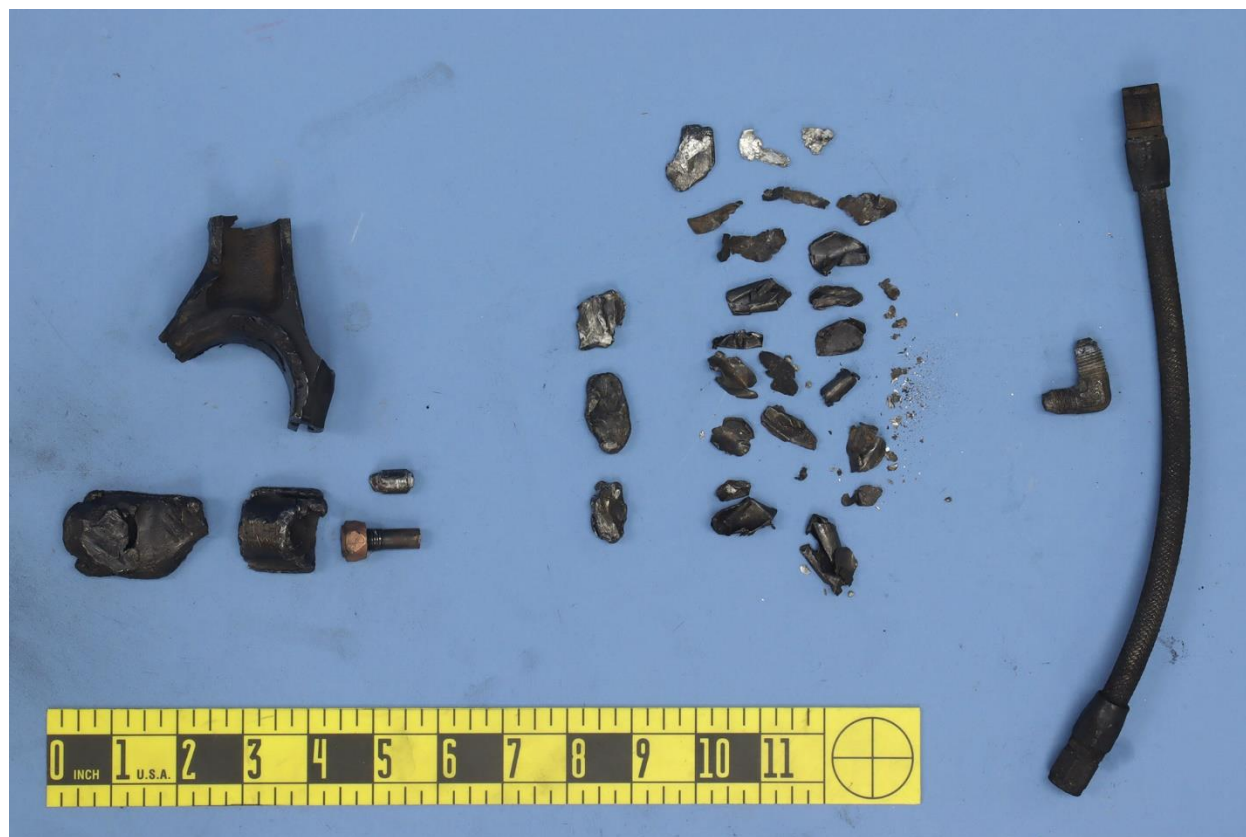
Figure 1: Connecting rod assembly pieces, fragments from sump, oil line, and elbow fitting, as received.
