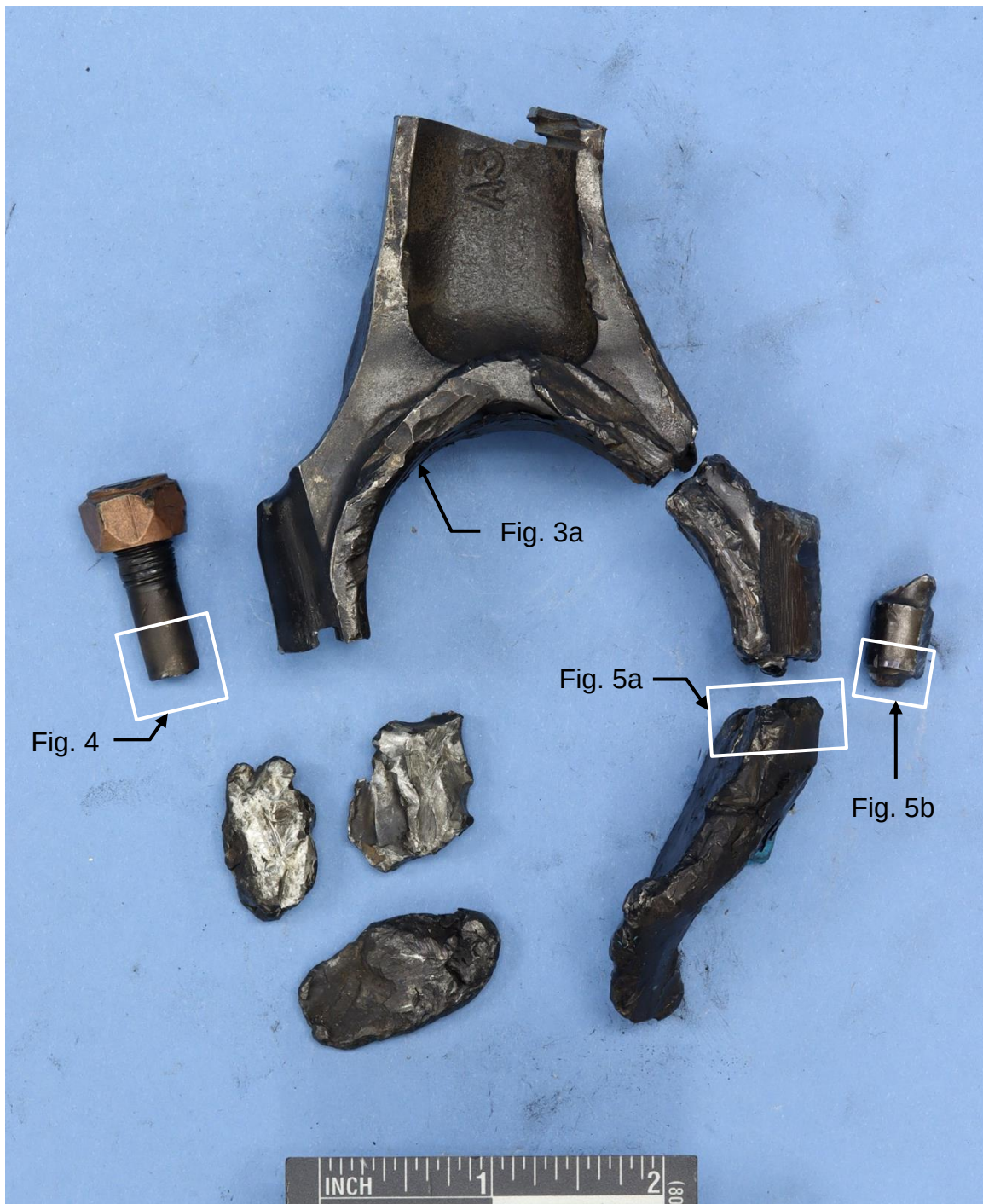
Figure 2: Connecting rod assembly pieces placed in their relative positions using fracture and interlocking surface features. Three fragments found in the sump were battered and their position could not be identified.
