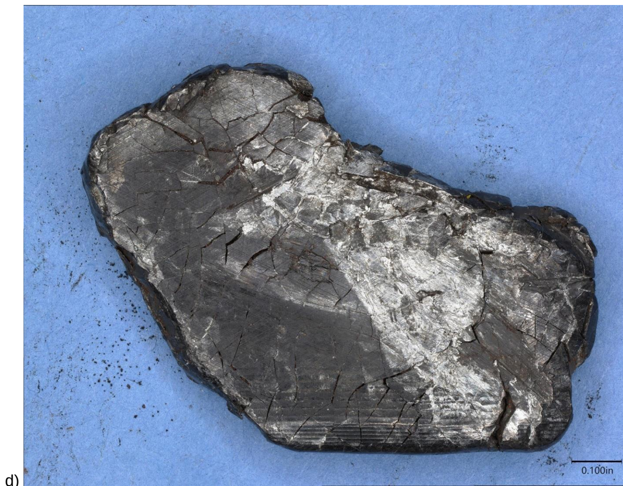
Figure 6 (cont.): c) EDS spectrum from one of the silver-metallic chips showing the presence of aluminum (Al) and silicon (Si); and d) thicker metal chip exhibiting mud cracking and smeared silver-metallic material.
