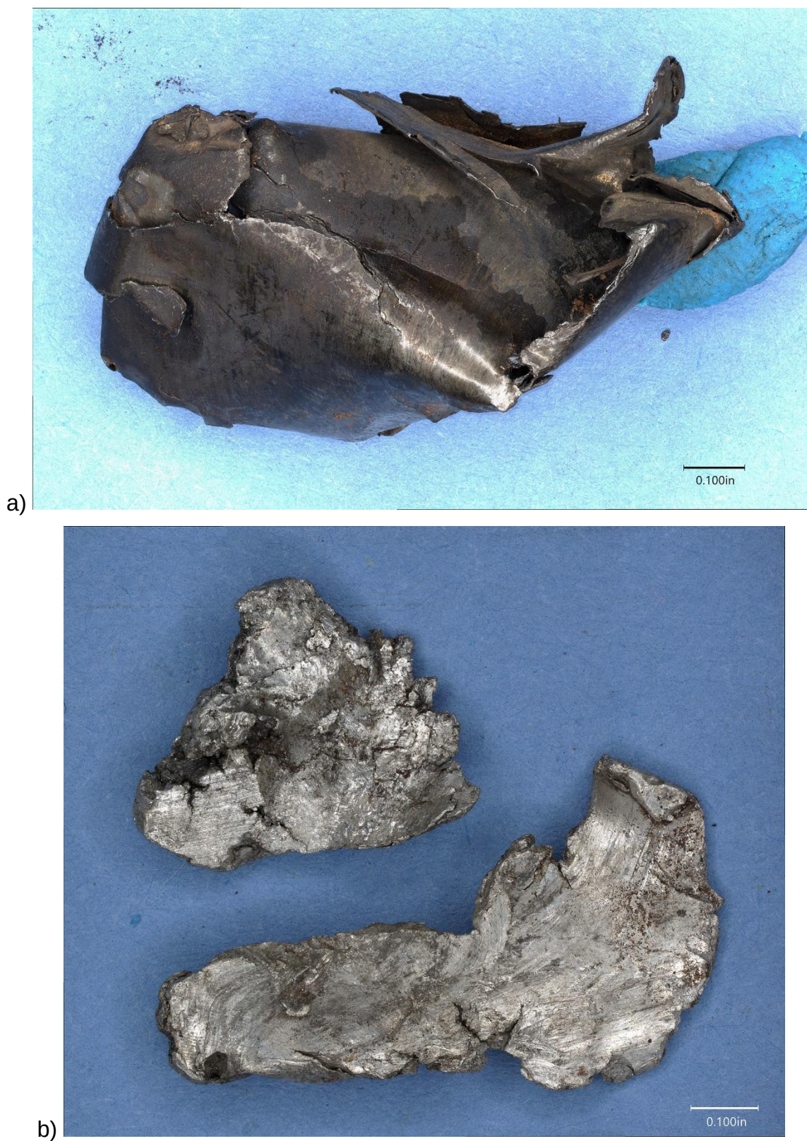
Figure 6: a) Image of a typical chip from the sump; b) two silver-metallic chips found in sump;
