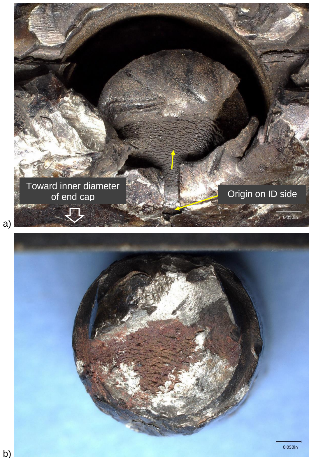
Figure 5: Images of mating fracture faces from the bolt on the right side of the connecting rod in figure 2: a) fracture face on a piece of bolt trapped in the end cap and b) mating fracture face on a free-standing bolt fragment.
