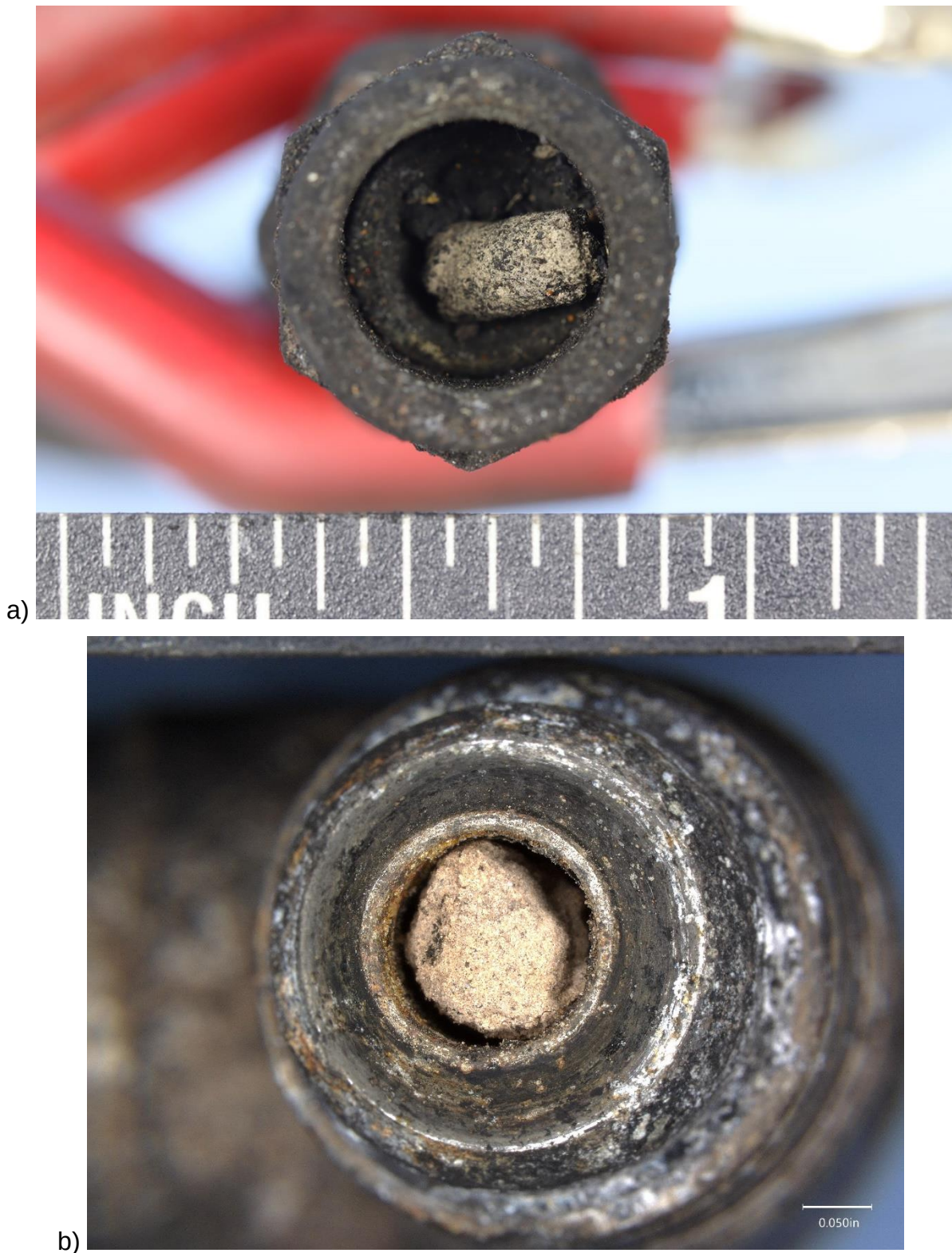
Figure 8: a) One end of the oil line showing an obstruction and b) the elbow fitting showing a piece of the obstruction at the entrance to the internal passage after it had been dislodged.
