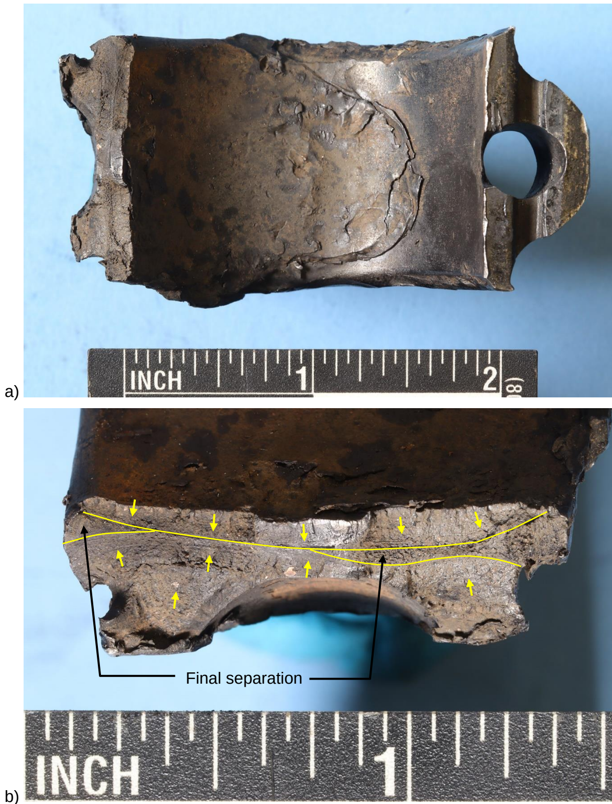
Figure 3: a) Image of the bearing saddle and fractured yoke on the connecting rod fragment; b) annotated view of the yoke fracture; and
