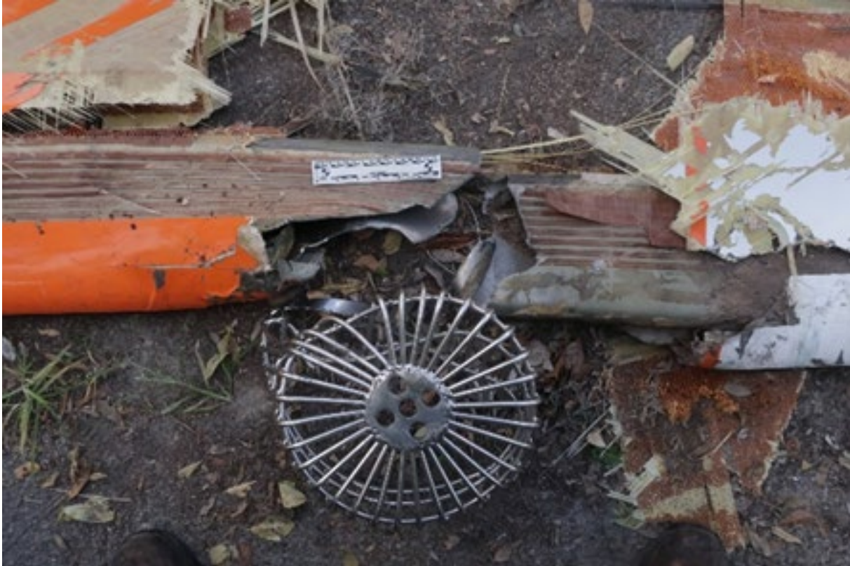
Figure 9. Yellow blade exhibiting semicircular shaped leading-edge separation and the snorkel pump basket deformed in the shape of the blade leading edge.
