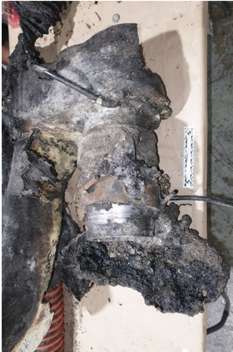
Figure 13. Forward side of the fire tank nozzle support and the snorkel hose connection.
