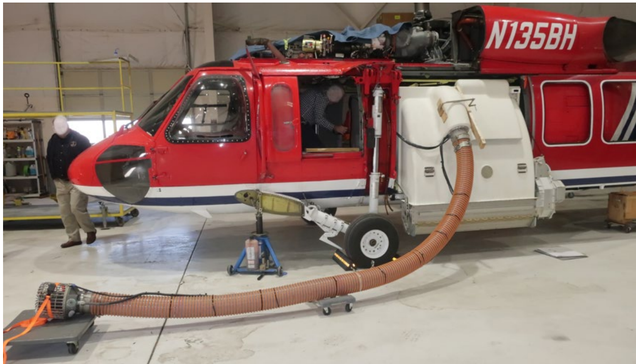
Figure 15. Exemplar fire tank installed for examination purposes.
