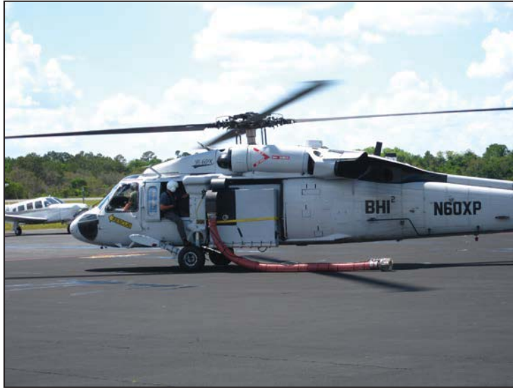
Fig. 10 – UH-60A test aircraft N60XP with prototype internal water tank . BME has completed over 59 hours of company flight testing with prototype water tank.
