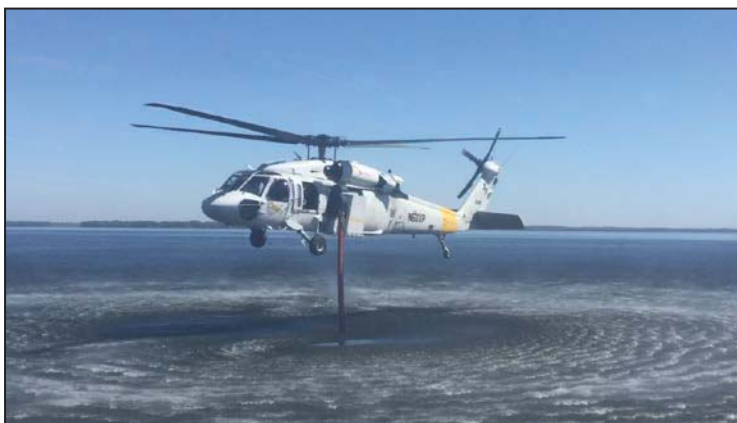
Fig. 13 – Test aircraft with prototype water tank in a hover collecting water
