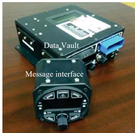
Fig. 6 – Data vault and message interface are installed in cockpit center console. The message interface display provides water quantity to the pilots in the cockpit at all times.
