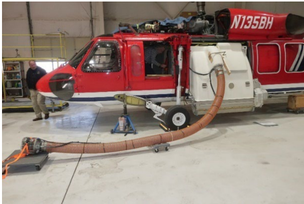
Figure 1. Left side of the helicopter showing the water tank installation and snorkel configuration.
