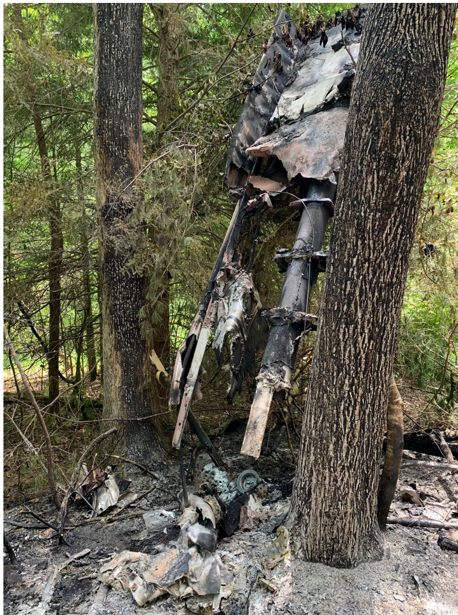
Photo 2 – View of Left Wing and Main Landing Gear Leg
