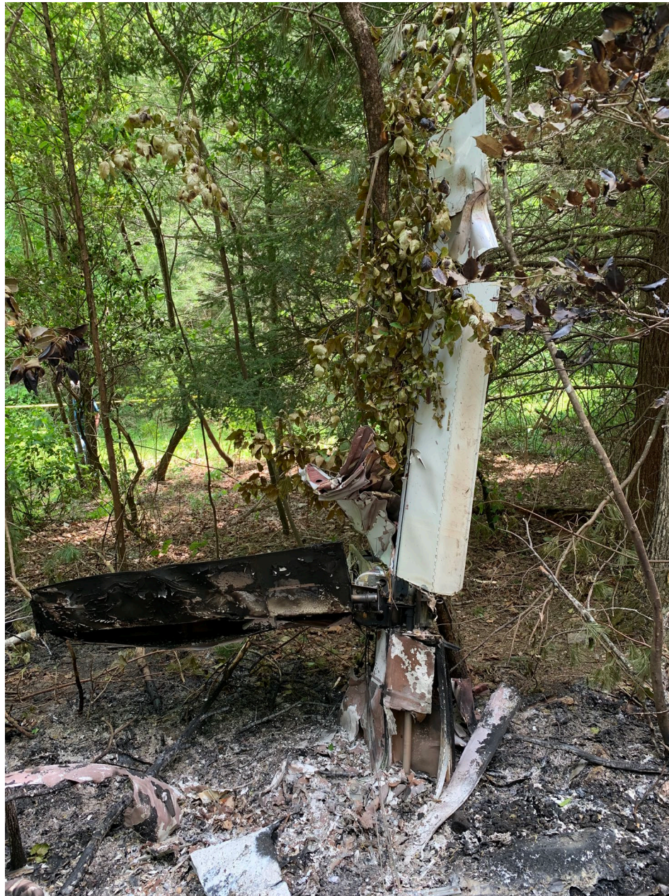
Photo 3 – Remains of Impact and Fire-Damaged Tail Section
