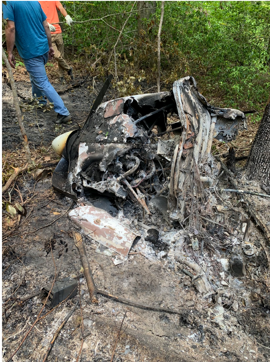
Photo 4 – View of Engine, Firewall, and Remains of Instrument Panel
