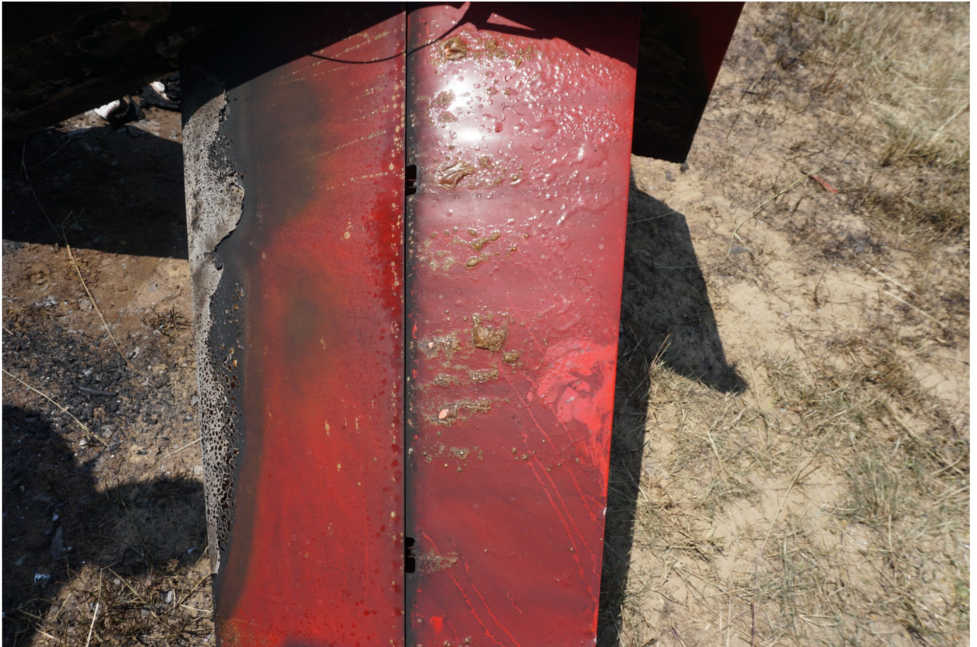
Photo 5 – View of under right horizontal stabilizer and elevator showing burnt oil streaks.
