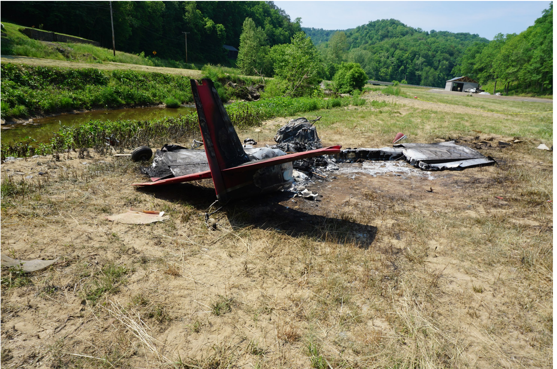
Photo 2 – View of fire damaged airplane aft.
