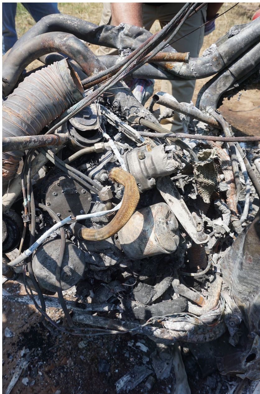
Photo 6 – View of fire damaged oil and fuel lines on accessory section.
