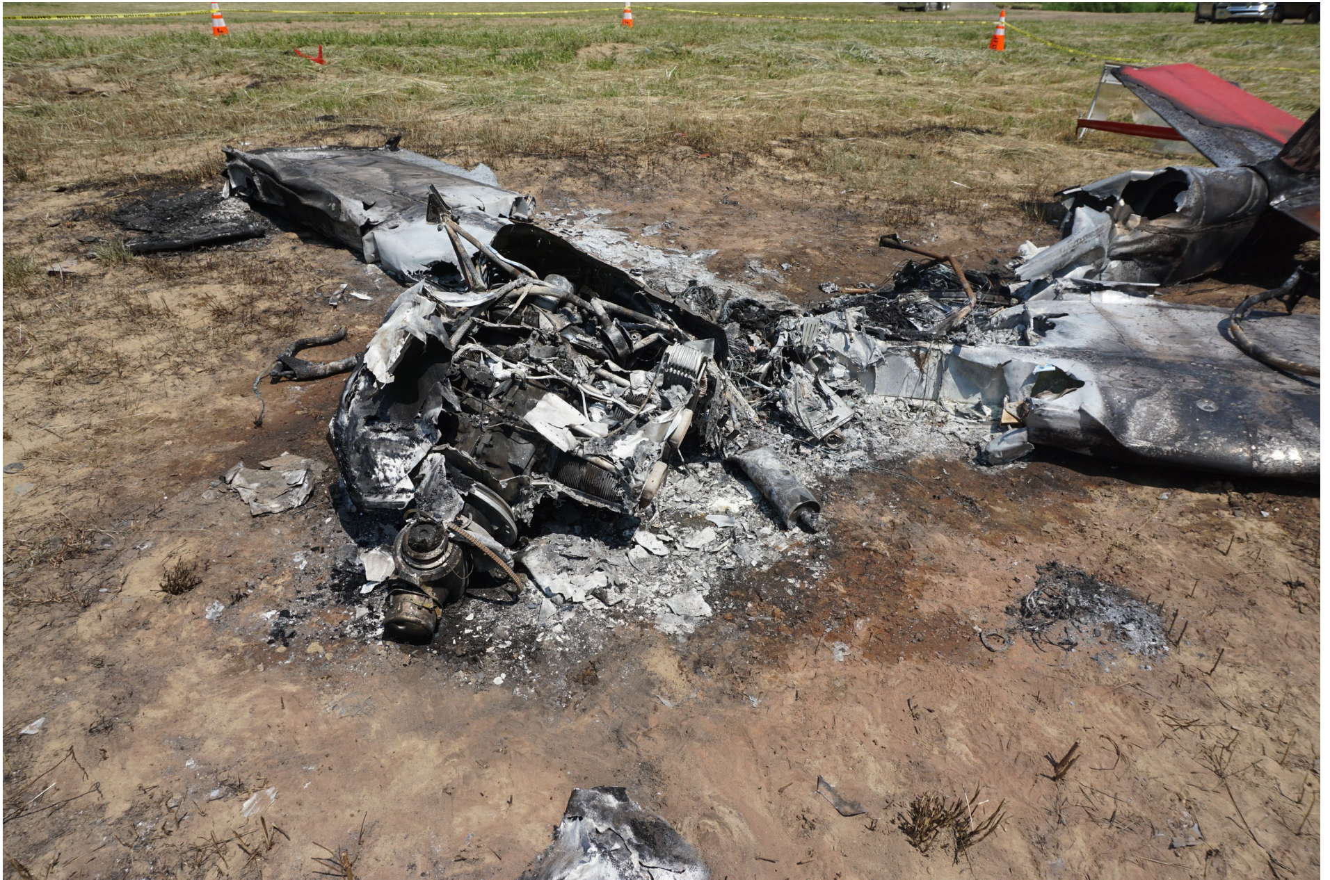
Photo 4 – View of fire damaged airplane froward showing engine, and cockpit.
