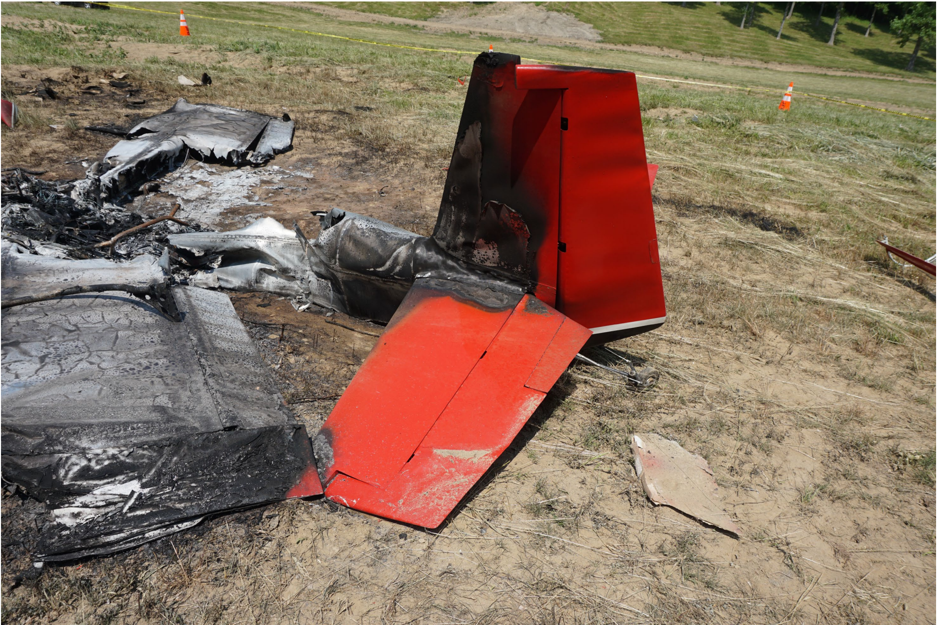
Photo 3 – View of left side of airplane showing fire damaged fuselage and empennage.
