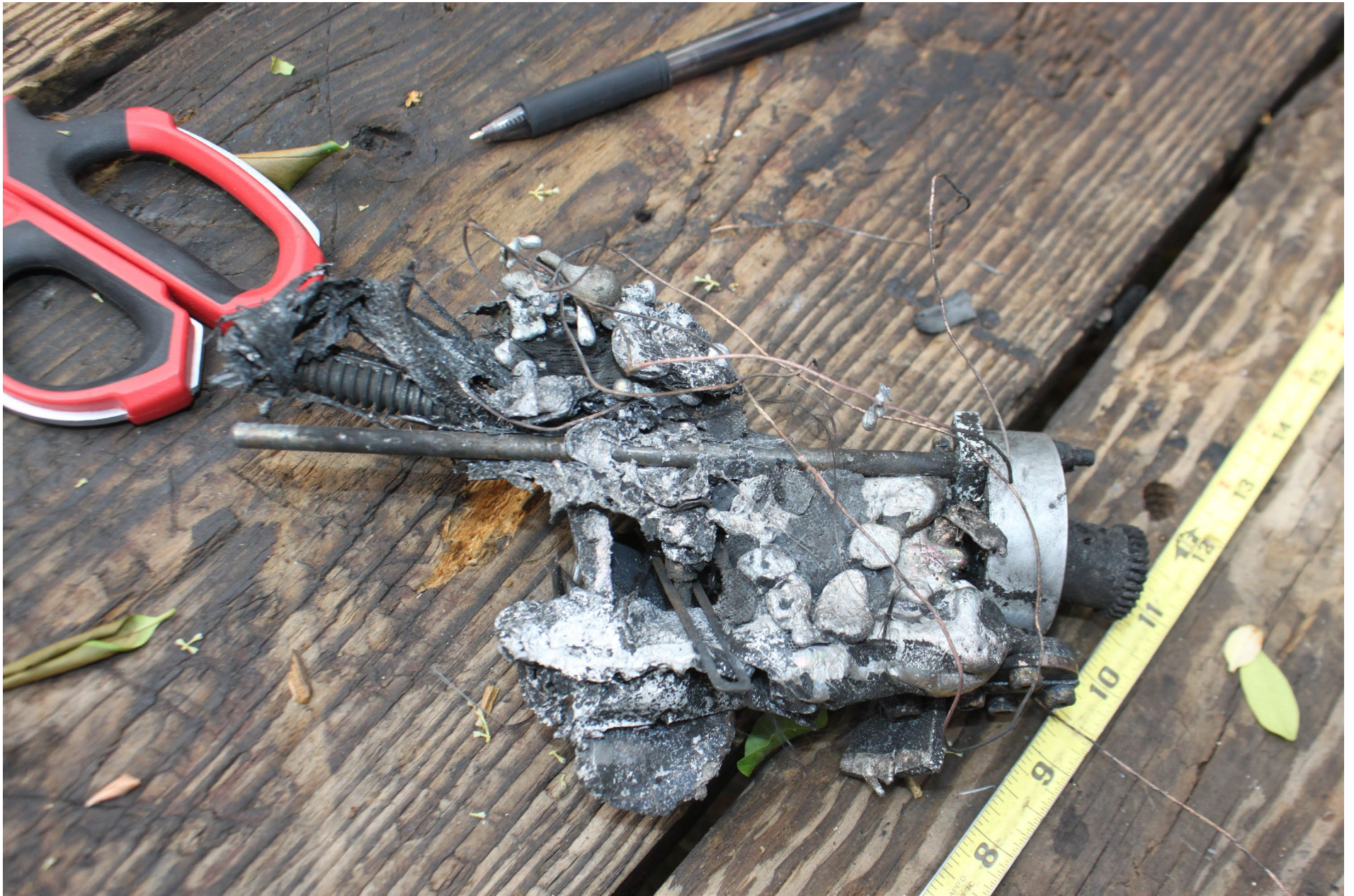
Photo 3 - NTSB Digital Photograph. View of the Extensively Heat Damaged Flap Motor/Actuator Assembly.
