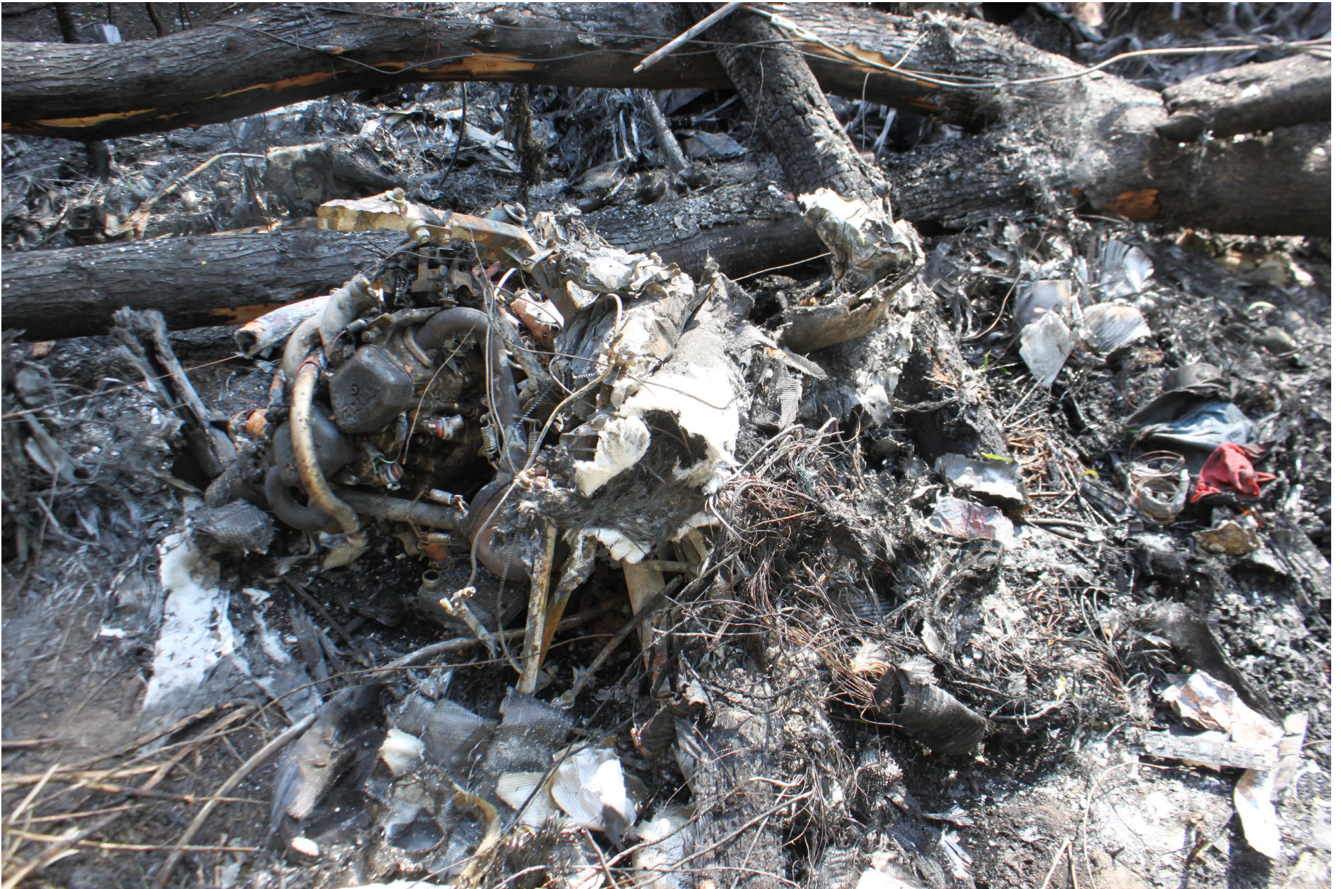
Photo 2 - NTSB Digital Photograph. View of the Extensively Heat Damaged Engine Assembly At the Accident Site.
