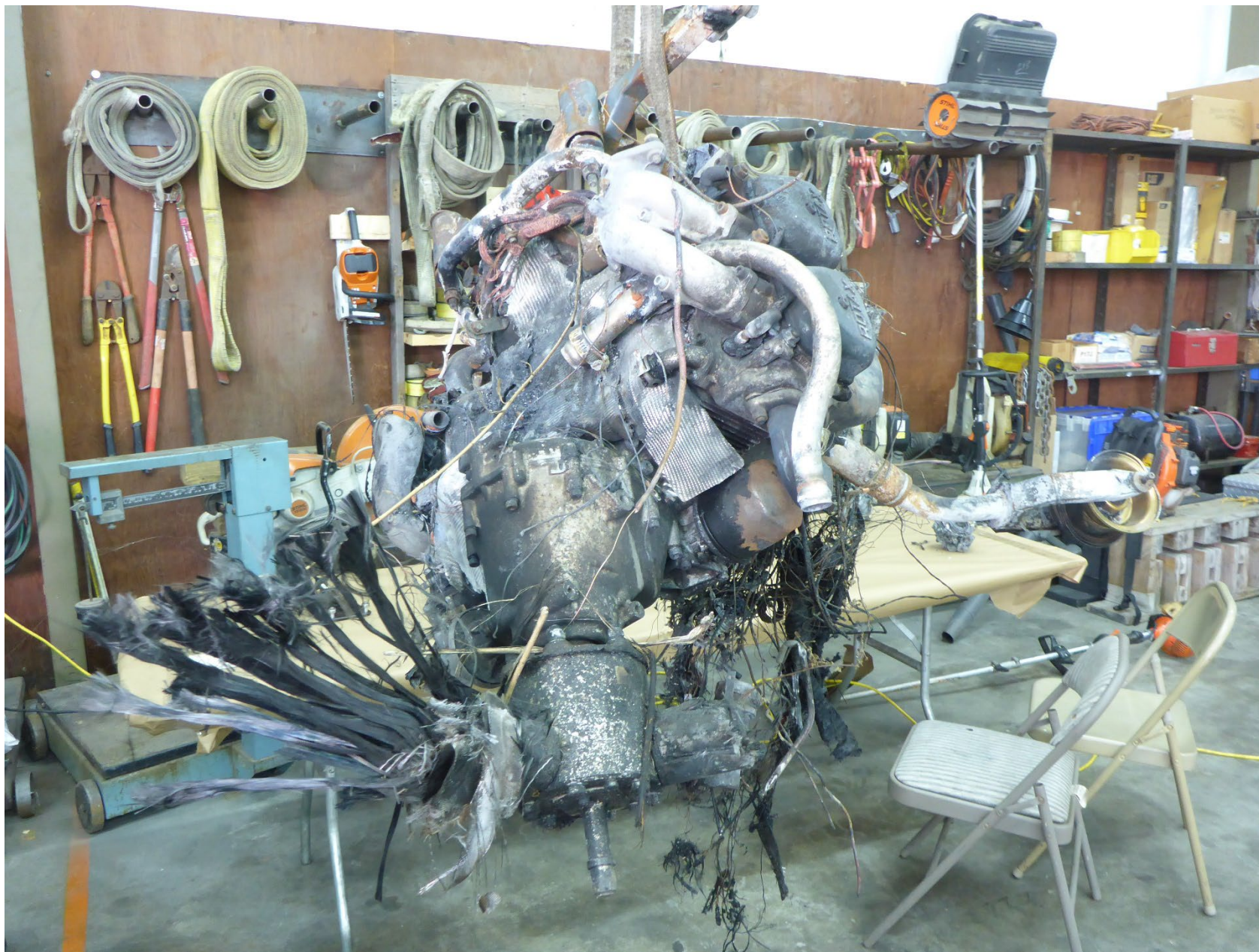
Photo 5 – Rotech Flight Safety Digital Photograph. Front and Top Views of the Extensively Heat Damaged Engine and Propeller Assembly Following Recovery.
