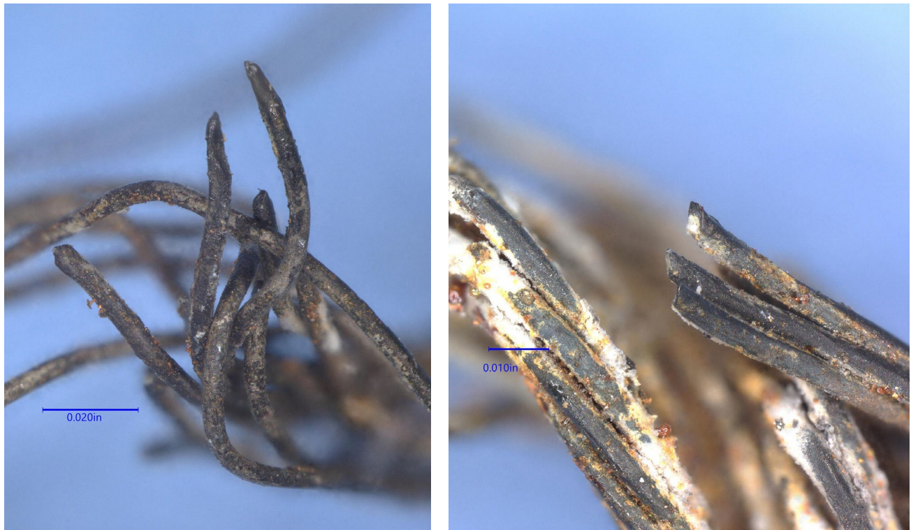
Figure 7: Wires from cable 1/3 1-B exhibiting necking, cup, and slant fractures.
