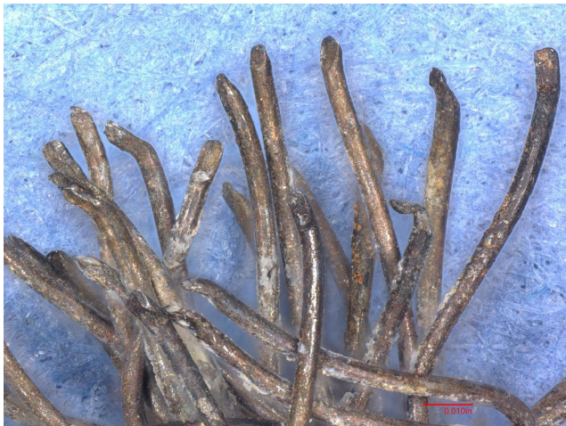
Figure 13: Wires from 2/4 2-A exhibiting chisel point fractures on the ends.
