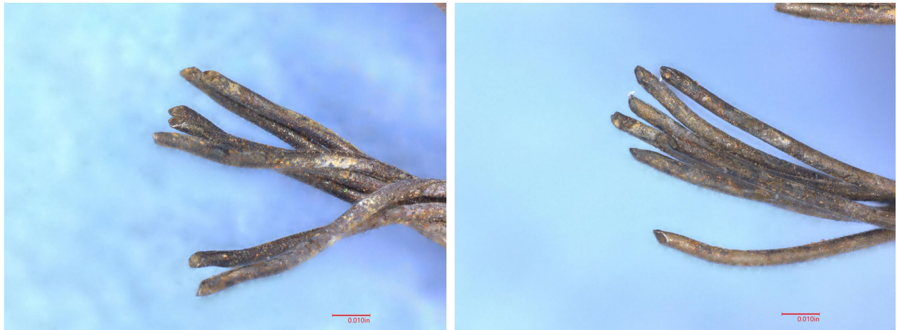
Figure 15: Wires from 2/4 2-B exhibiting necking and slant fractures.
