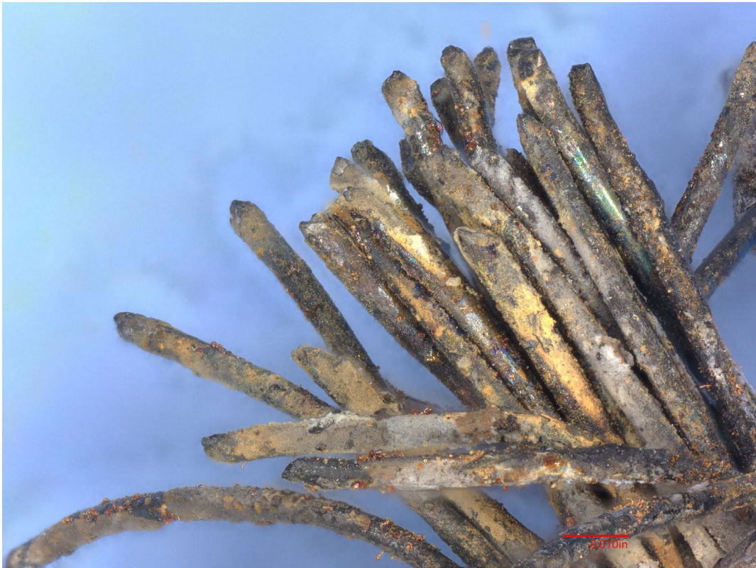
Figure 5: Wires from cable 1/3 1-A exhibiting chisel point fractures.
