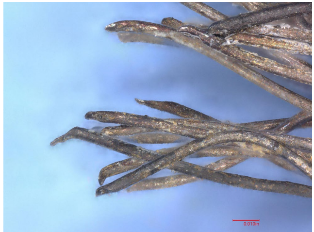
Figure 13: Wires from 2/4 2-A exhibiting chisel point fractures on the ends.
