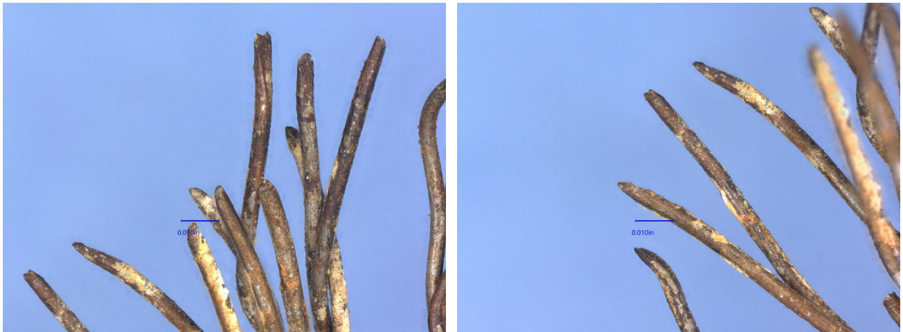
Figure 9: Wires from 2/4 1-A exhibiting necking, cup, and slant fractures.
