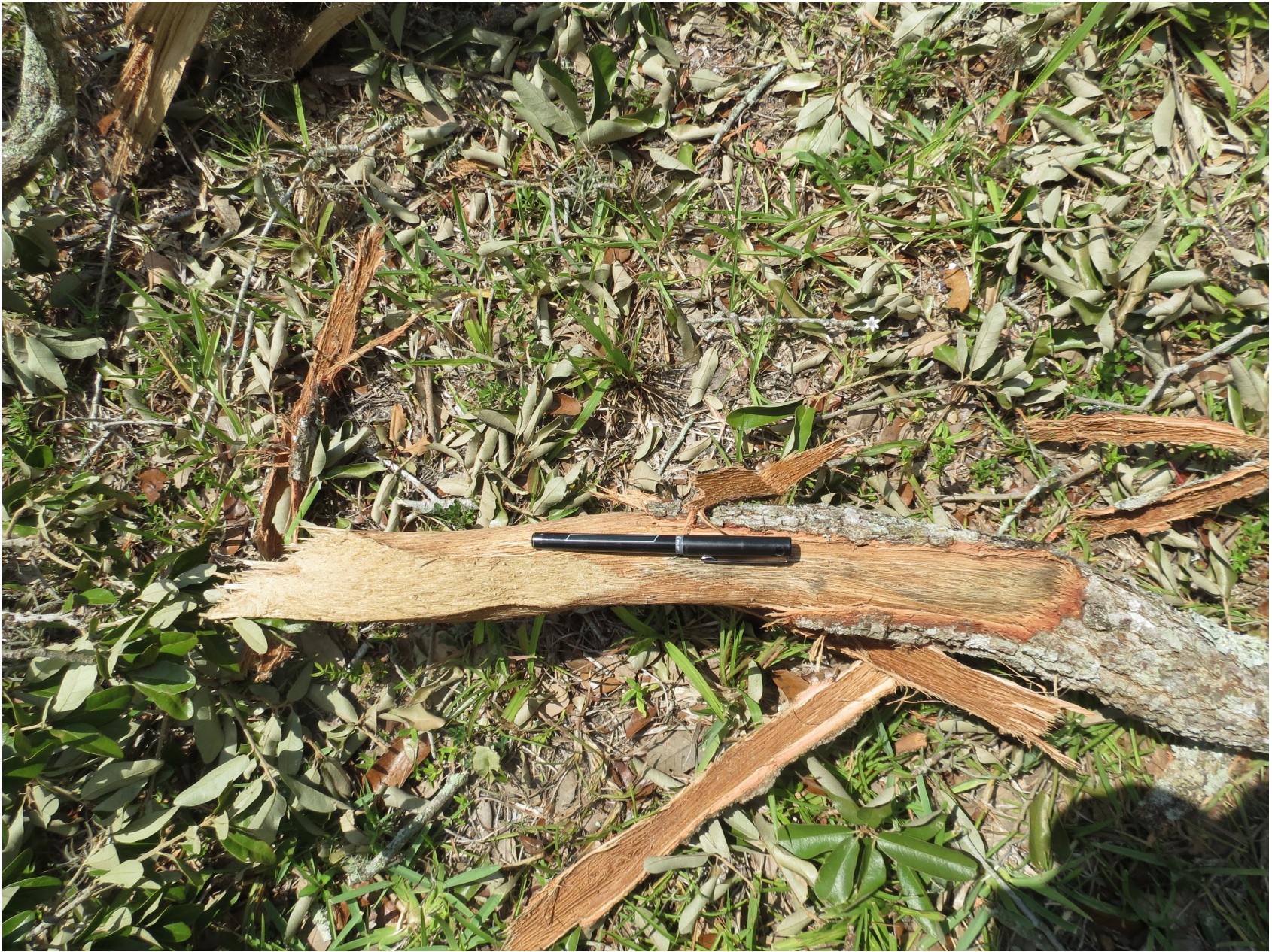
Photo 3 – Angularly Cut Wood with Paint Transfer (Lycoming)
