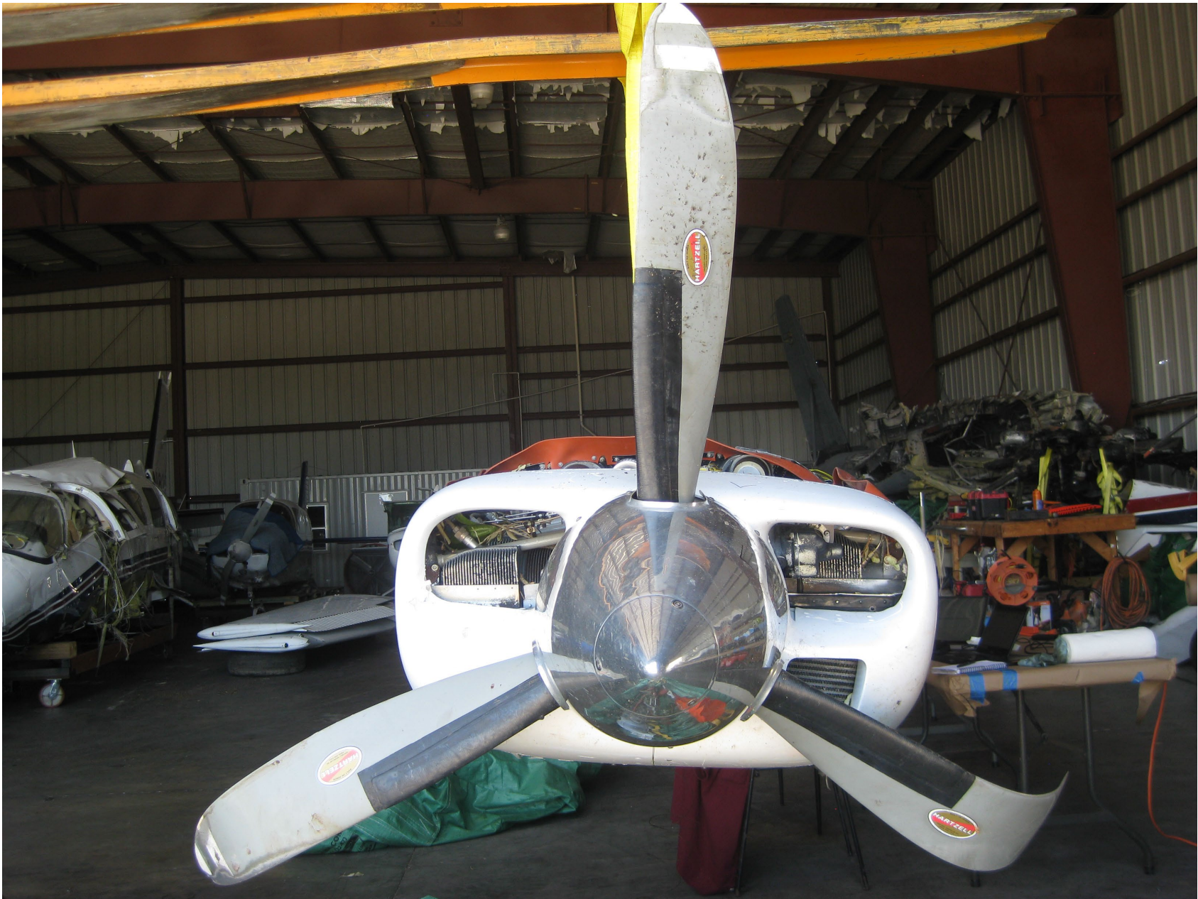
Photo 7 – View of Left Propeller Tip Curl and Blade Polishing (Lycoming)
