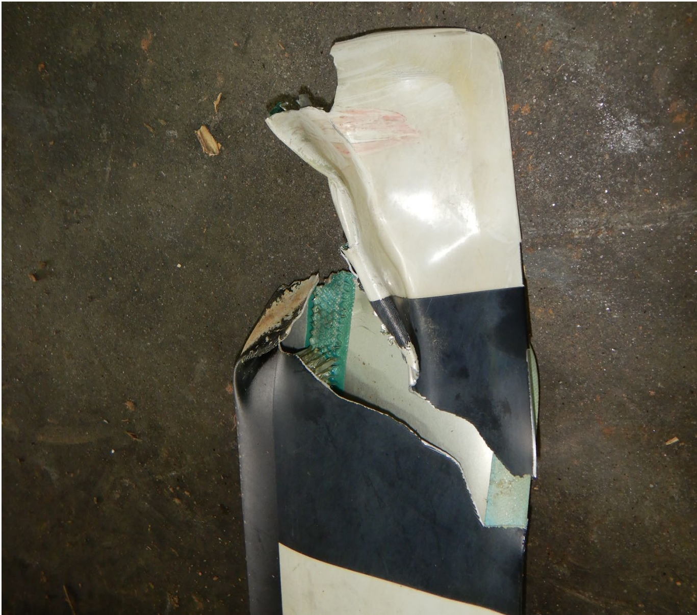
Photo 5 – View of rotor blade tip with evidence of impact with the tail rotor guard
