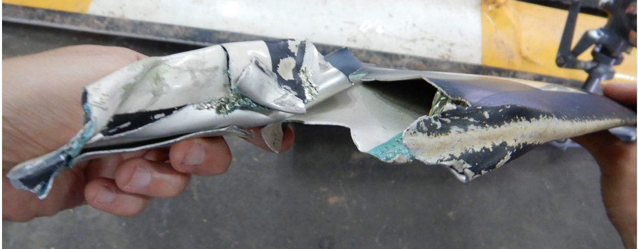
Figure 5: Fractured tail rotor blade
