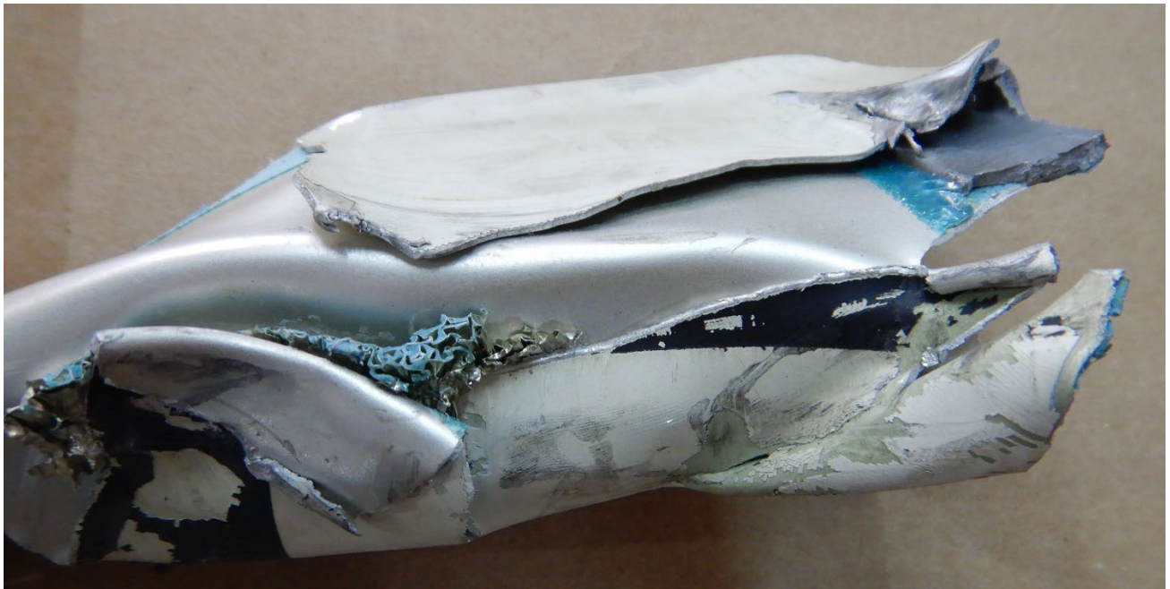
Figure 6: Close up view of wire strike impact signatures
