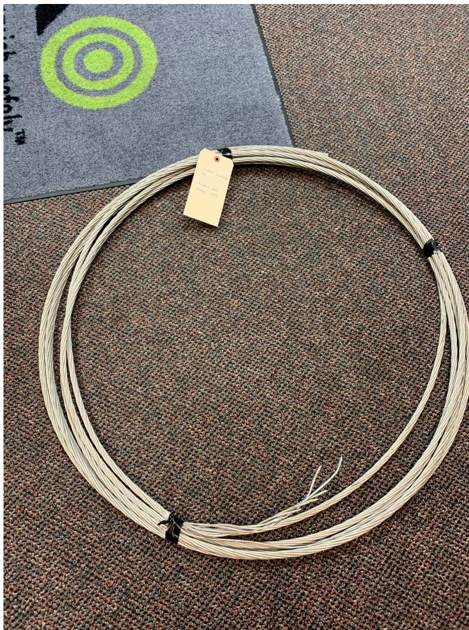
Photo 6 – Piece of the broken cable (powerline)
