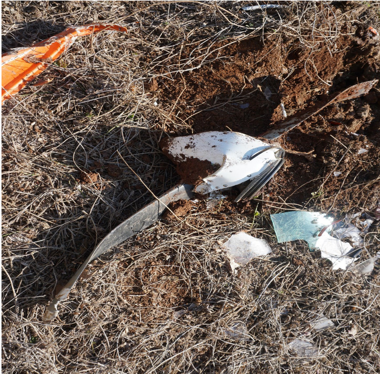
Photo 2 – View of propeller at wreckage site, showing gouges in blade and twist.
