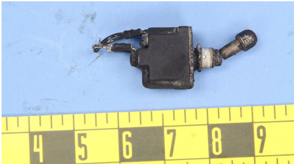
Figure 1. Overall photograph of accident switch.
