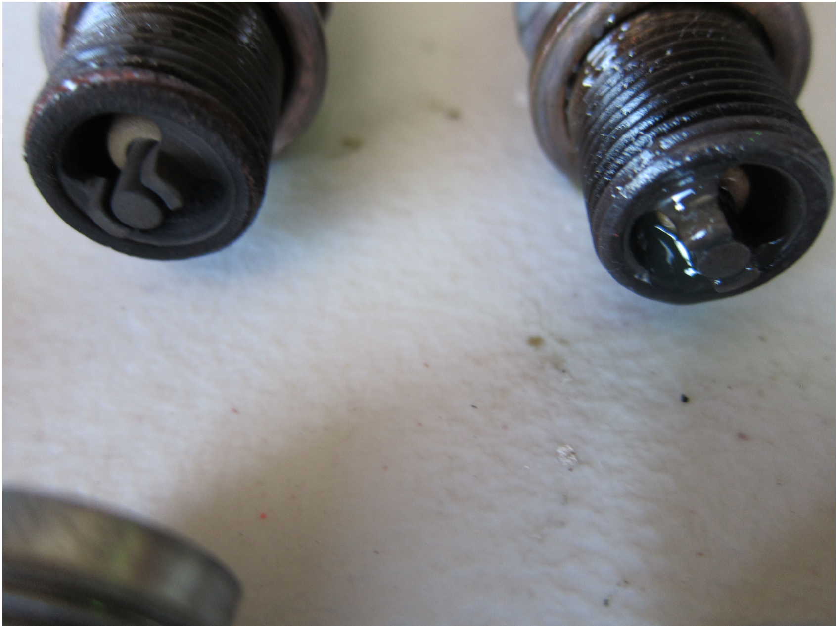
Photo 15 - Continental Aerospace Technologies Digital Photograph. View of the Cylinder Portions of the Nos. 4 and 6 Bottom Spark Plugs. No. 4 is on the Left. Note the soot color.
