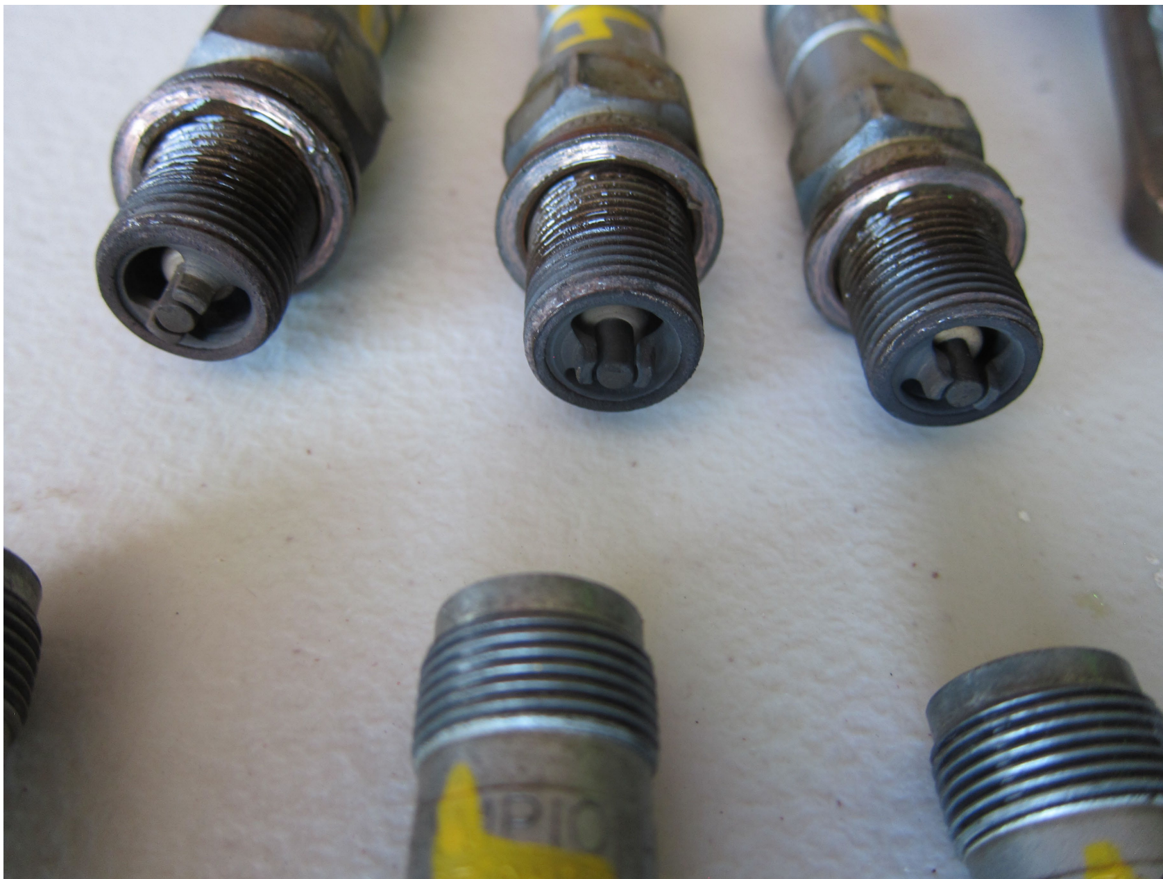
Photo 13 - Continental Aerospace Technologies Digital Photograph. View of the Cylinder Portions of the Nos. 2, 4, and 6 Top Spark Plugs. No. 2 is on the Left. Note the soot color.
