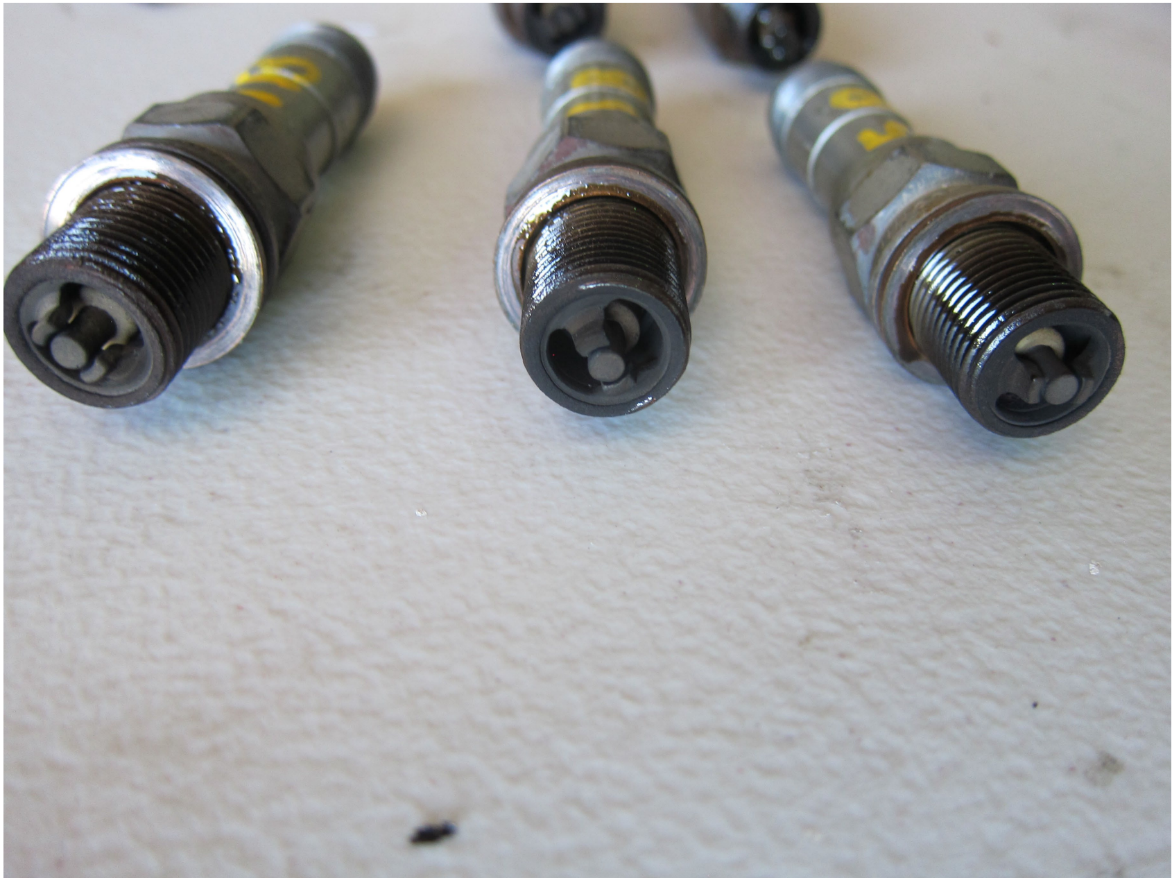
Photo 14 - Continental Aerospace Technologies Digital Photograph. View of the Cylinder Portions of the Nos. 1, 3, and 5 Bottom Spark Plugs. No. 1 is on the Left. Note the soot color for Nos. 3 and 5.
