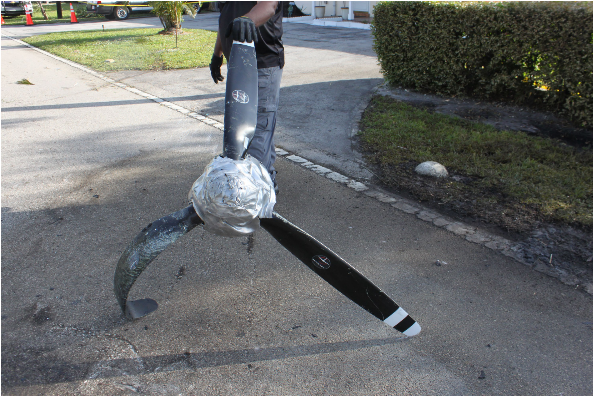
Photo 10 - NTSB Digital Photograph. Frontal View of the Separated Propeller.
