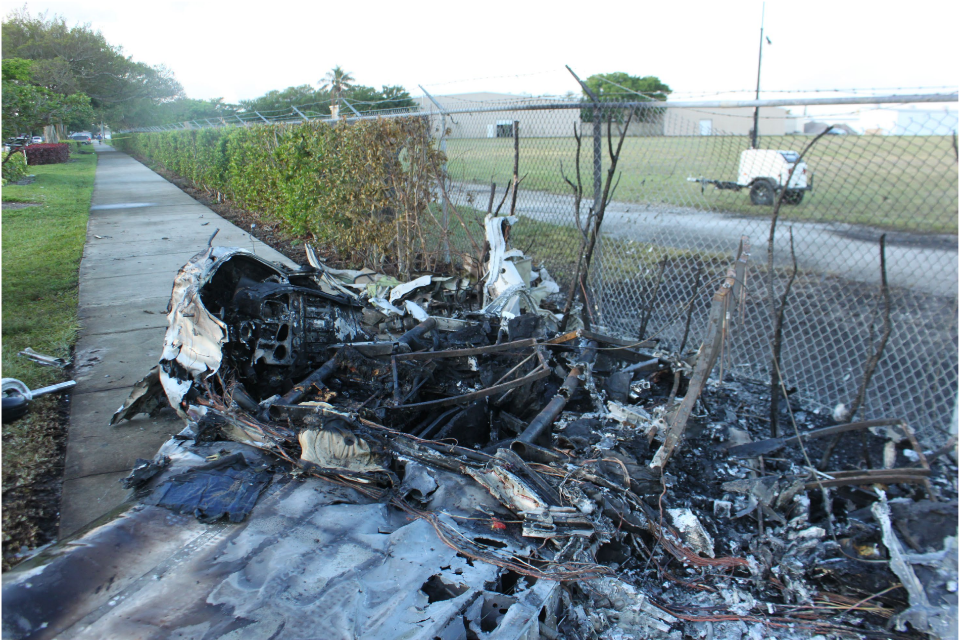
Photo 7 - NTSB Digital Photograph. Left Side View Showing the Inboard Portion of the Left Wing, and Heat Damaged Cockpit and Cabin.
