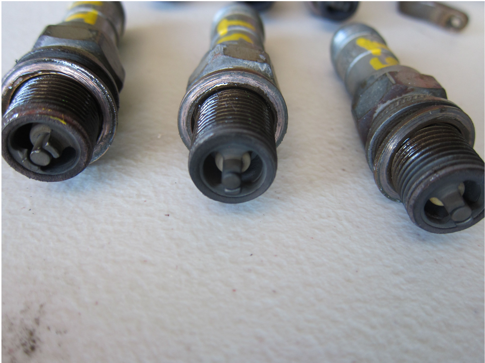
Photo 12 – Continental Aerospace Technologies Digital Photograph. View of the Nos. 1, 3, and 5 Top Spark plugs. No. 1 is on the Left. Note the soot color.
