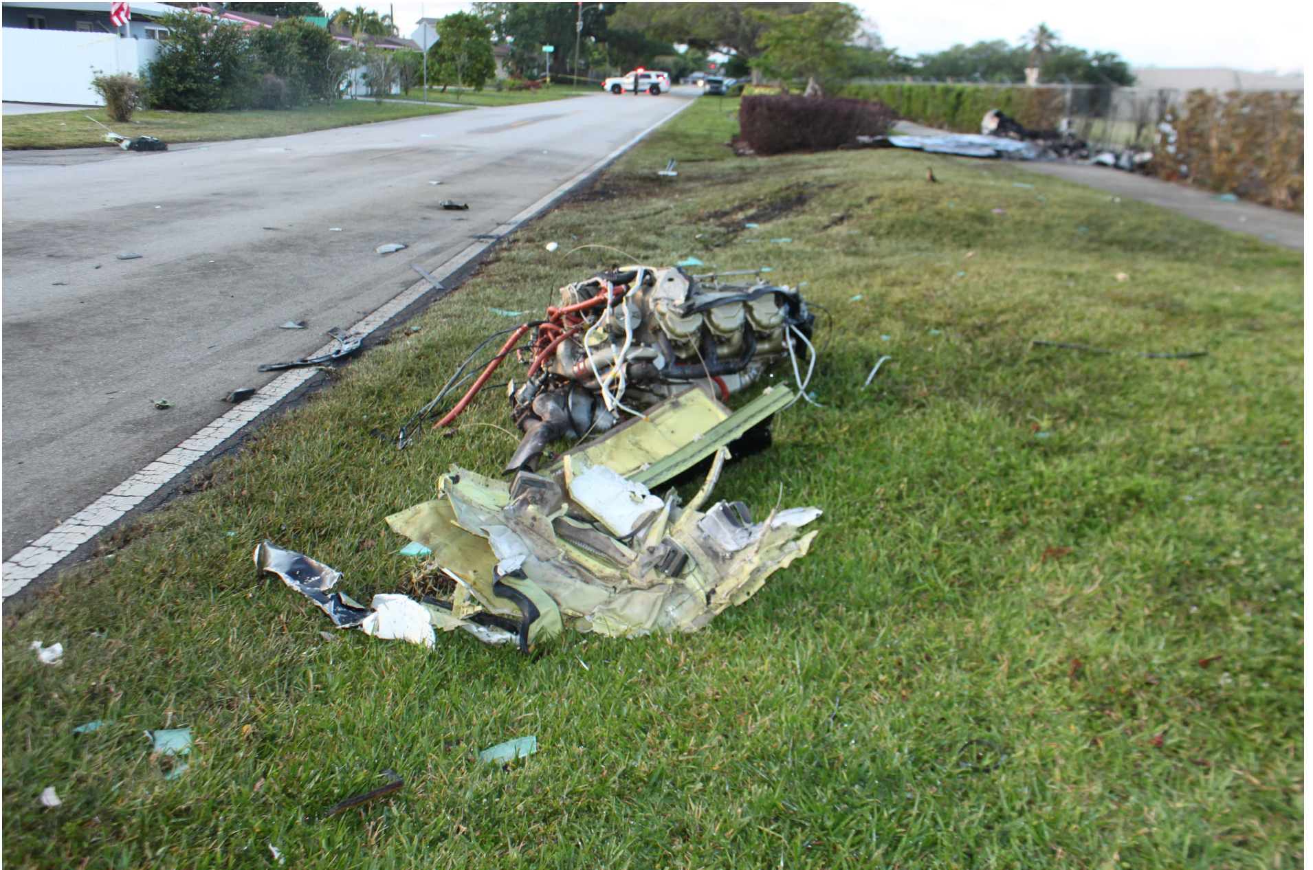
Photo 3 - NTSB Digital Photograph. View of the Separated Engine. Note the Wreckage in the Background.
