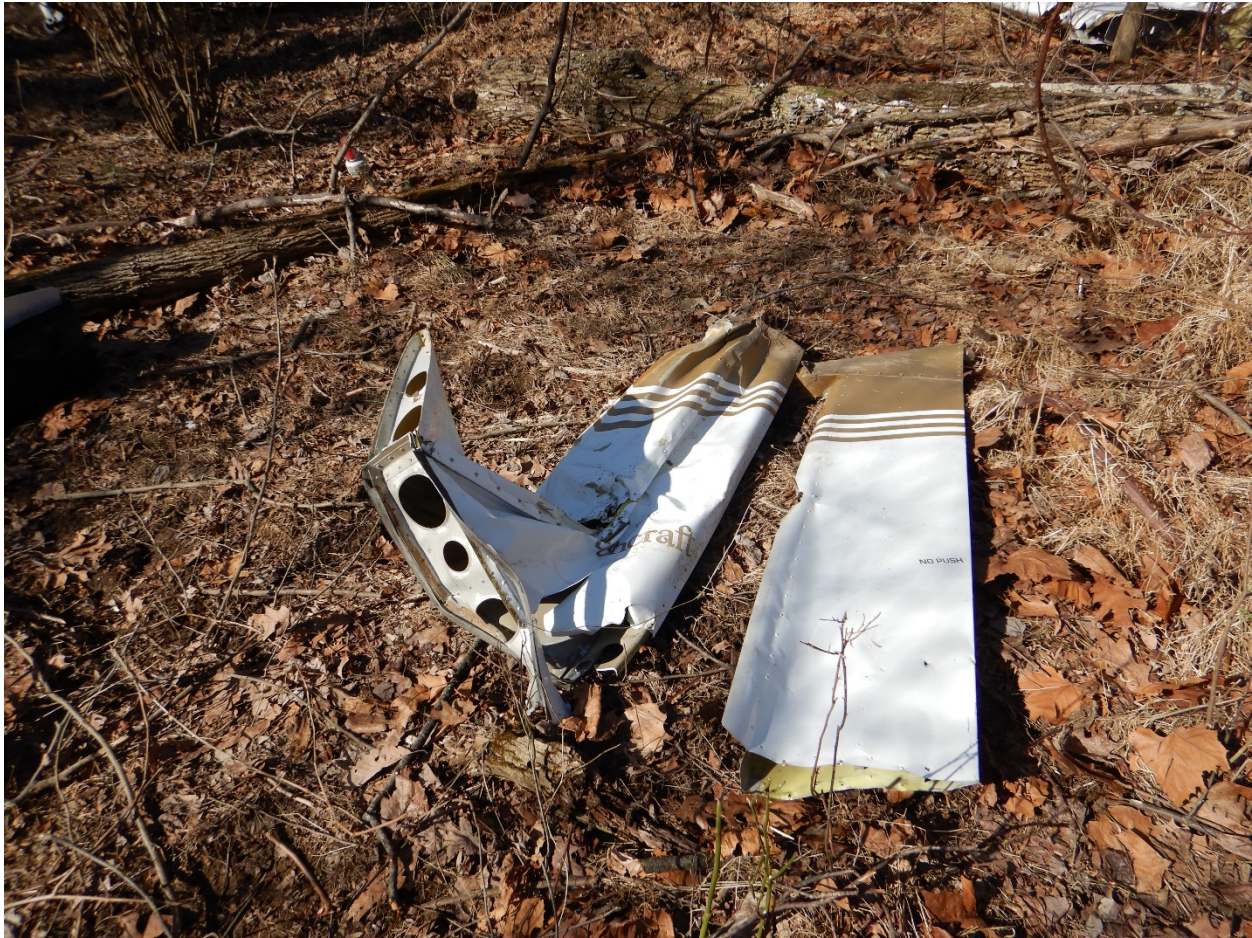
Figure 3. Rudder and Vertical Stabilizer
