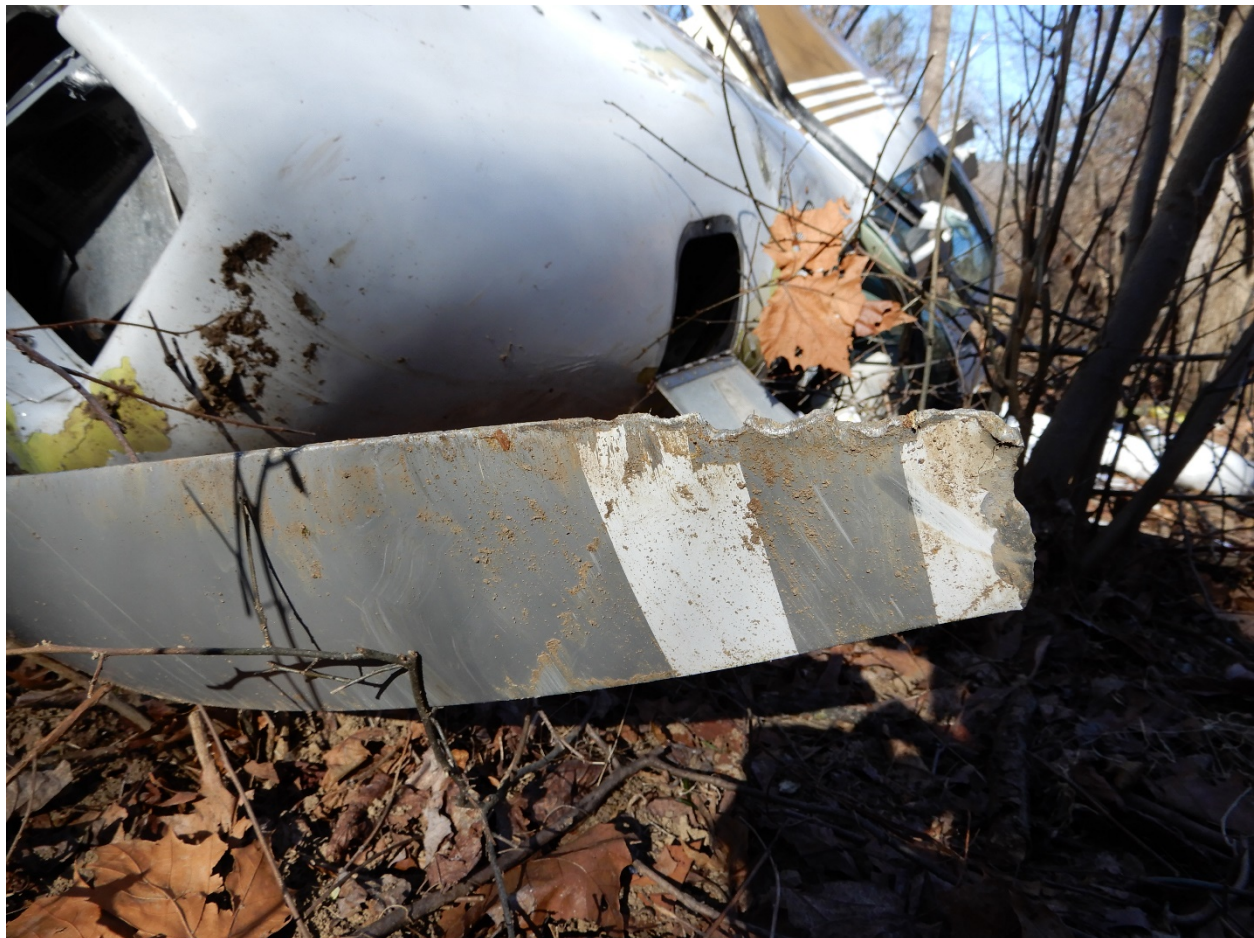
Figure 7. View of leading edge gouging, chordwise scratching, and tip tearing on one propeller blade.
