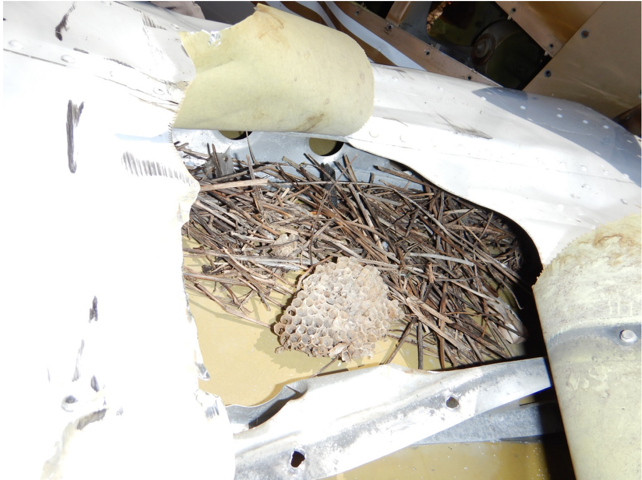
Figure 4. Nest inside right side of horizontal stabilator.
