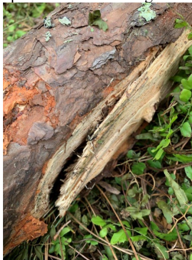
Figure 6 Propeller signatures on tree
