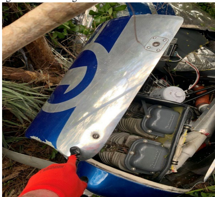
Figure 8 Damaged engine cowl showing fasteners
