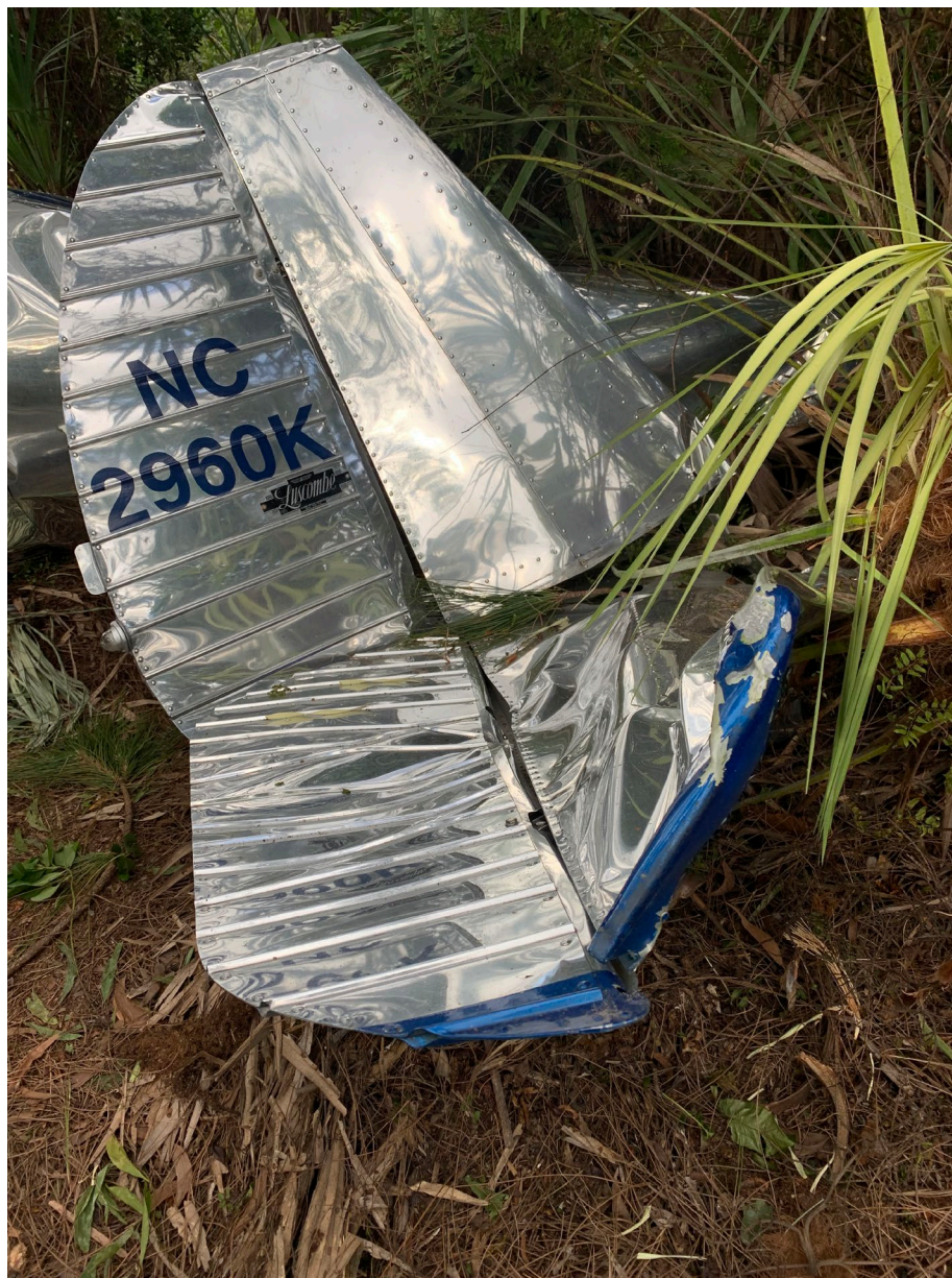
Photo 3 – View of right side of rudder, elevator and stabilizer damage.
