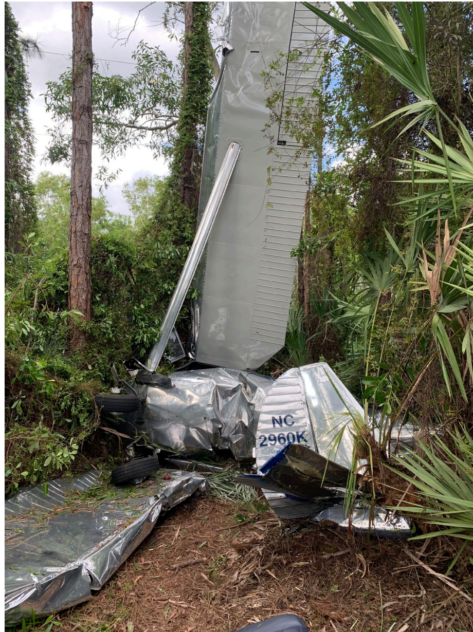
Photo 1 –View of airplane wreckage as discovered. Left wing nearly vertical and right wing detached and resting beside wreckage on ground.
