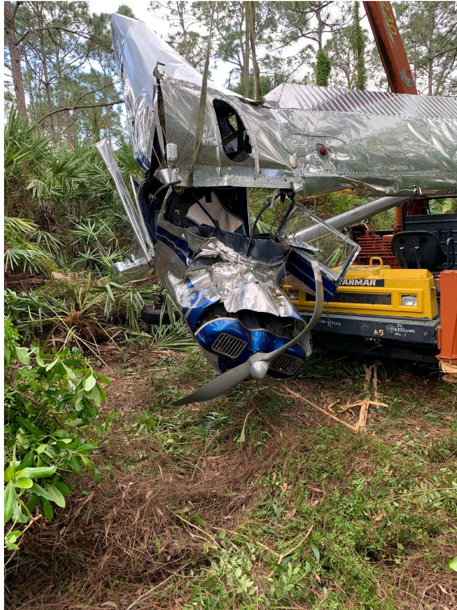
Photo 9 – Overall forward view of wreckage during recovery. Note damage to cockpit, propeller and left wing.
