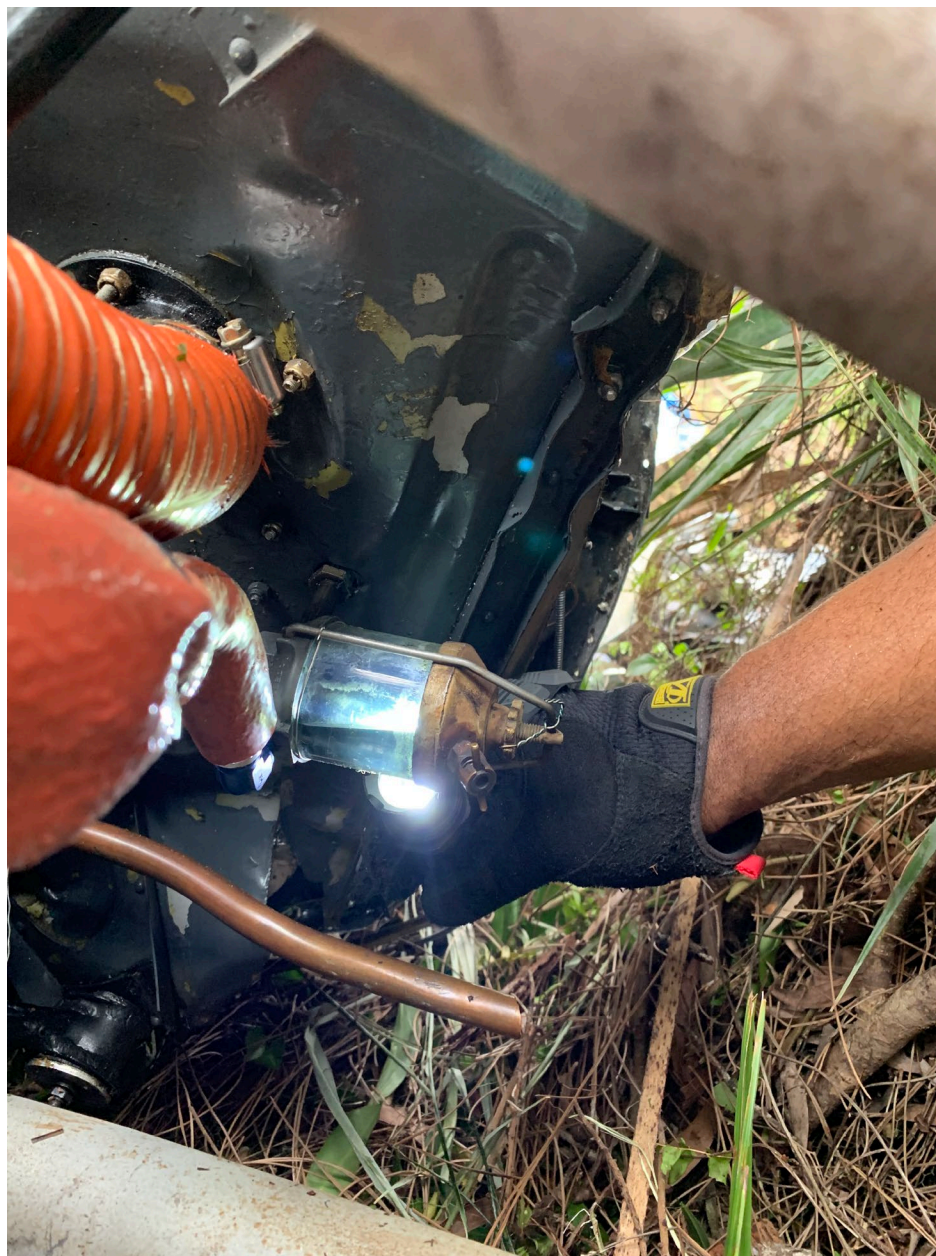
Photo 7 – View of fuel gascolator in wreckage. Note: contained fuel.
