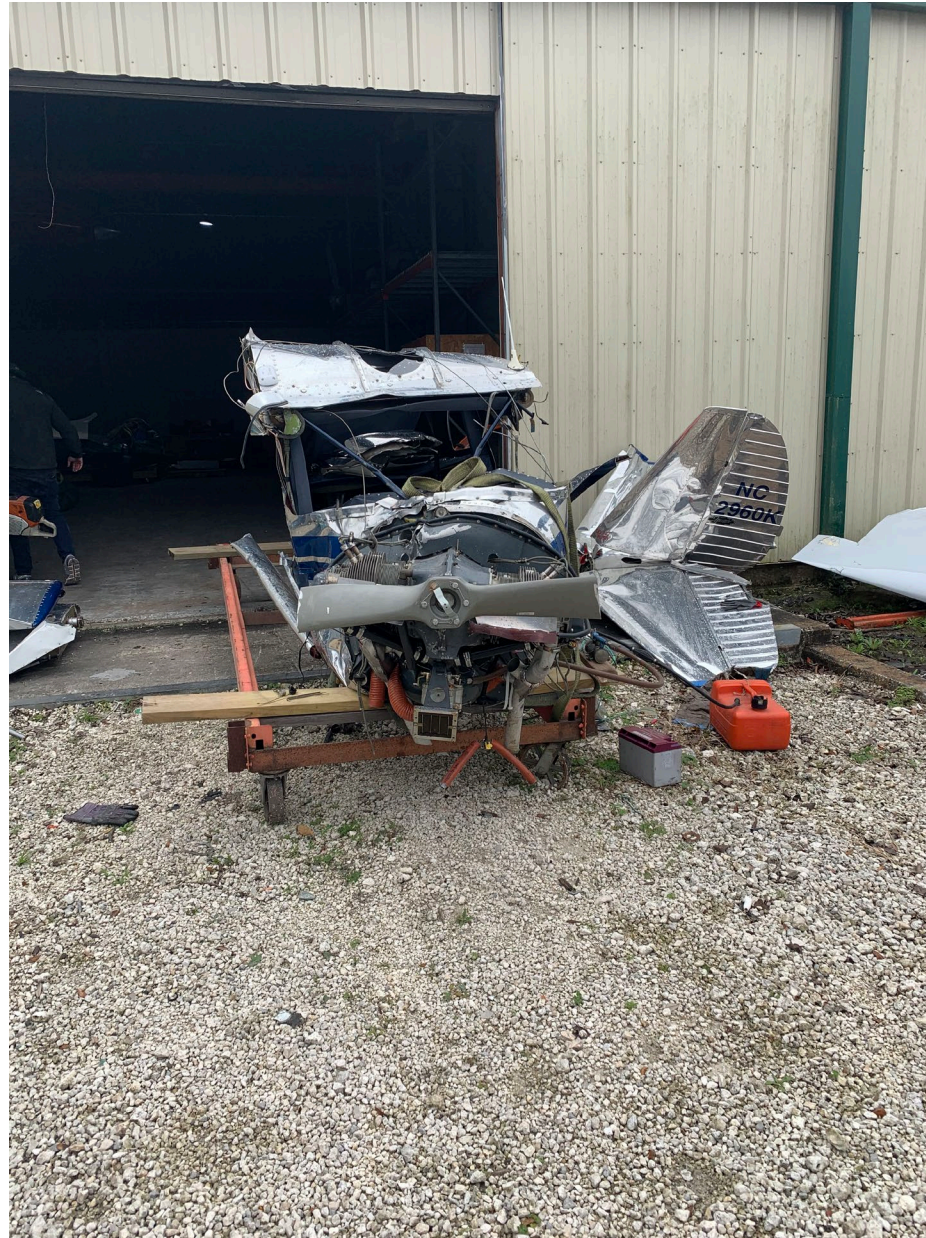
Photo 10 – View of engine and fuselage on test stand after successful engine run.
