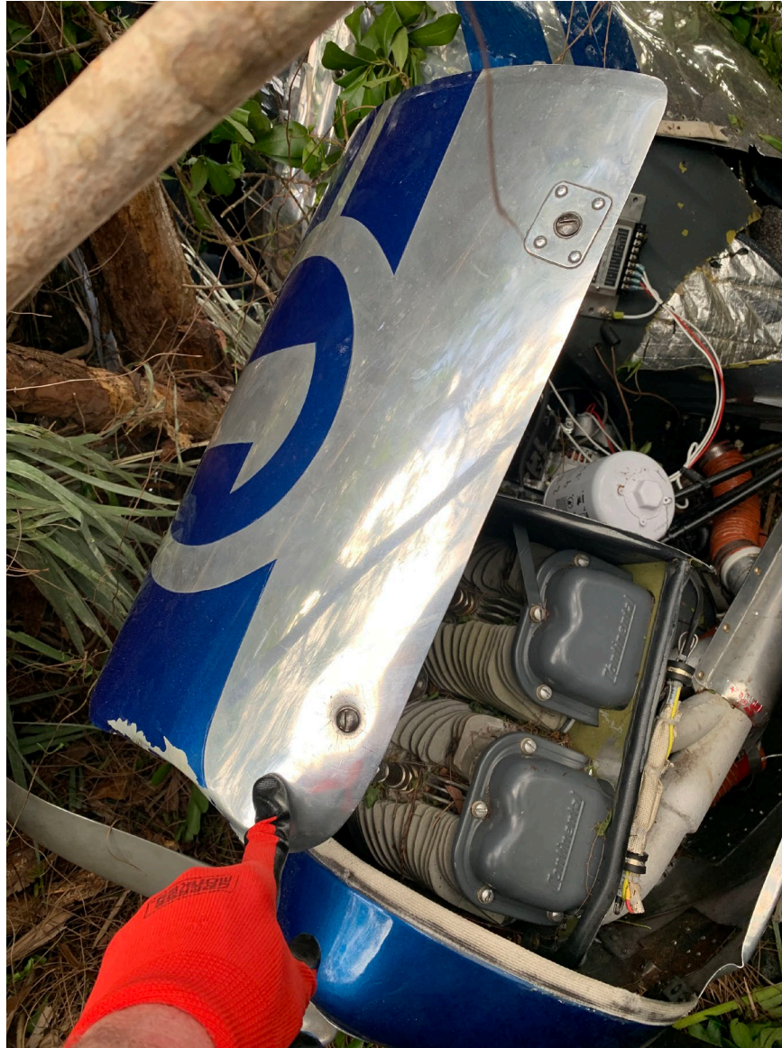
Photo 6 – View of left cowl that opened during takeoff.
