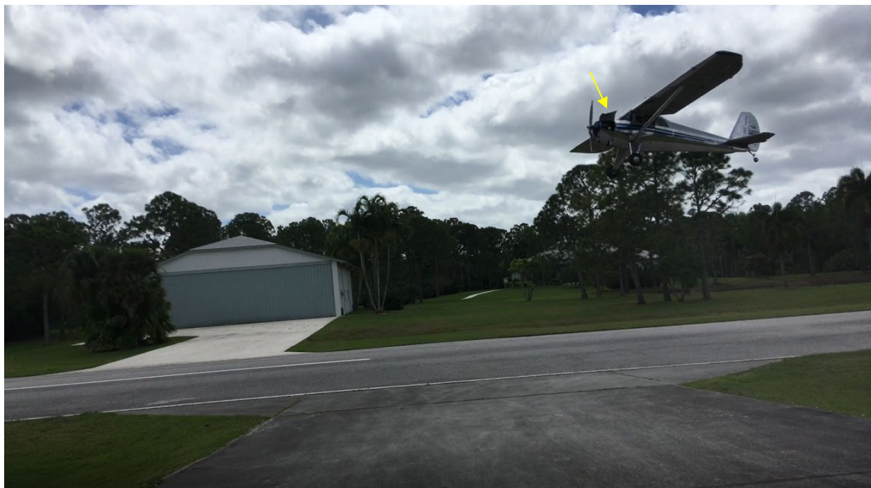
Figure 2. Still from second 14 of video. The engine cowling (yellow arrow) is open and flapping.
