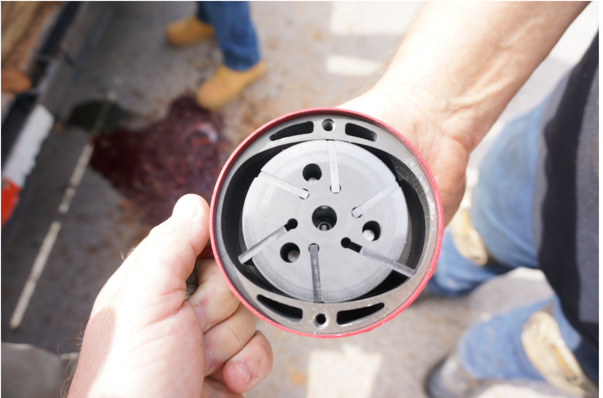
Photo 17 – Interior of Vacuum Pump
