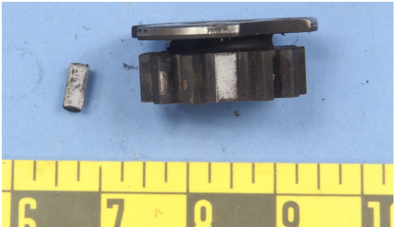
Figure 5 – View of the mating fracture surfaces of the drive gear and liberated tooth.
