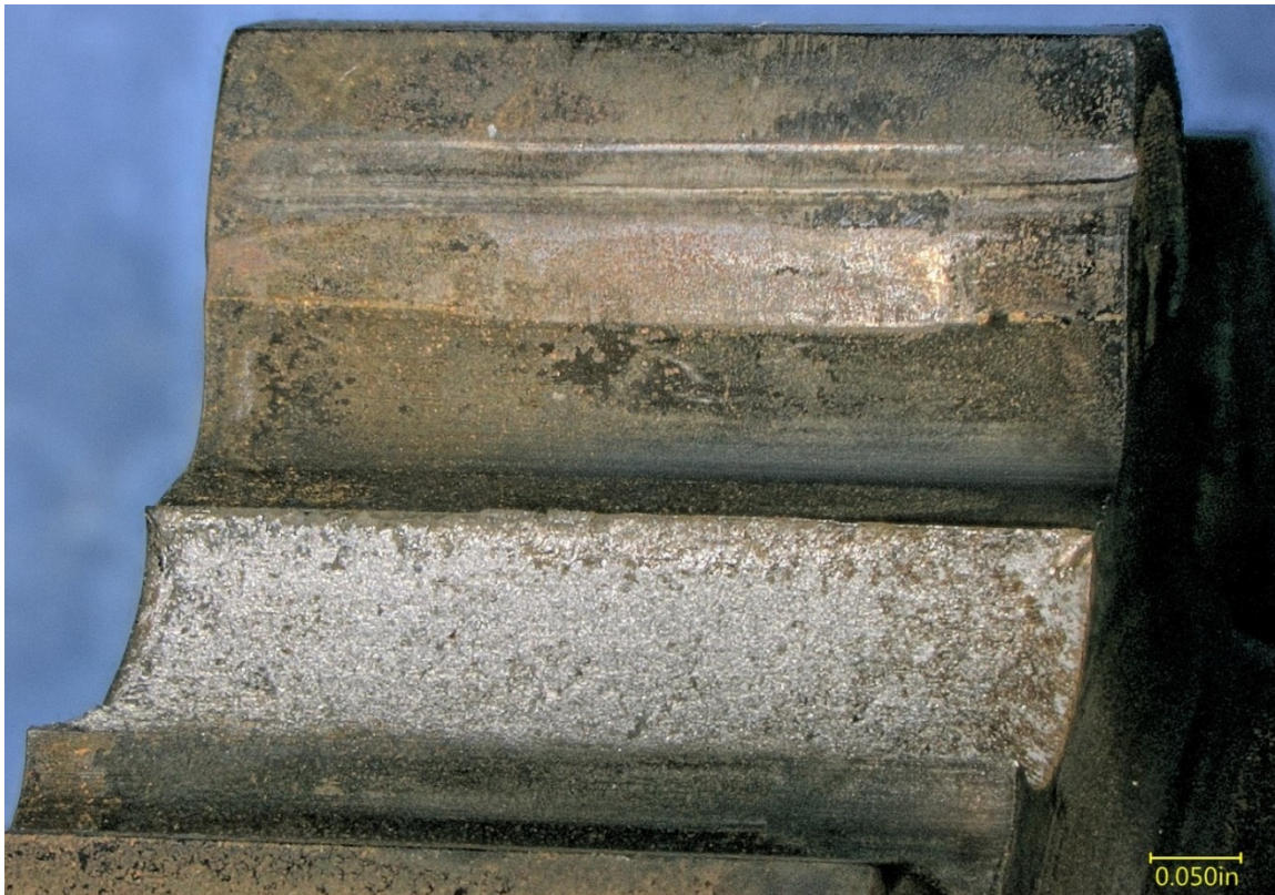
Figure 7 – Angled view of the gear fracture surface, showing the adjacent tooth.
