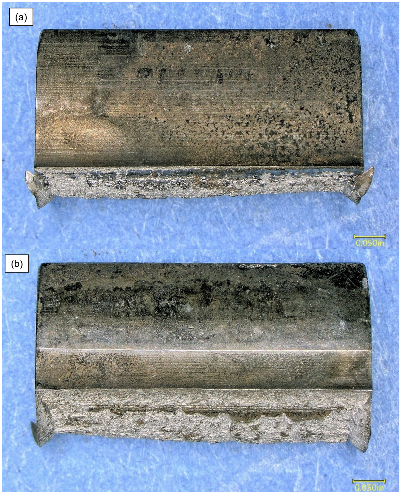
Figure 12 – View of the fractured tooth from (a) the lagging face and (b) driven face.
