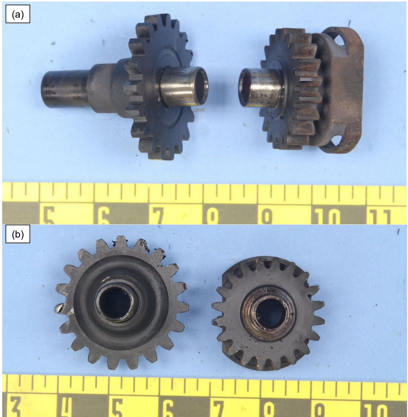
Figure 3 – The pair of accessory gears, as received; viewed from (a) the sides and (b) the gear faces.
