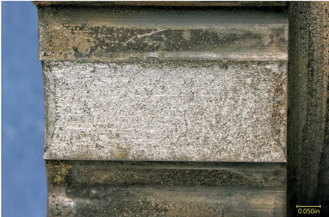
Figure 6 – The fractured tooth surface of the drive gear.
