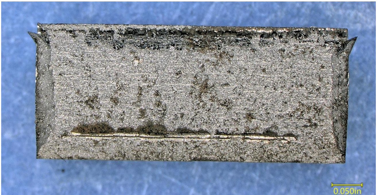
Figure 11 – View of the fracture surface of the fractured drive gear tooth.
