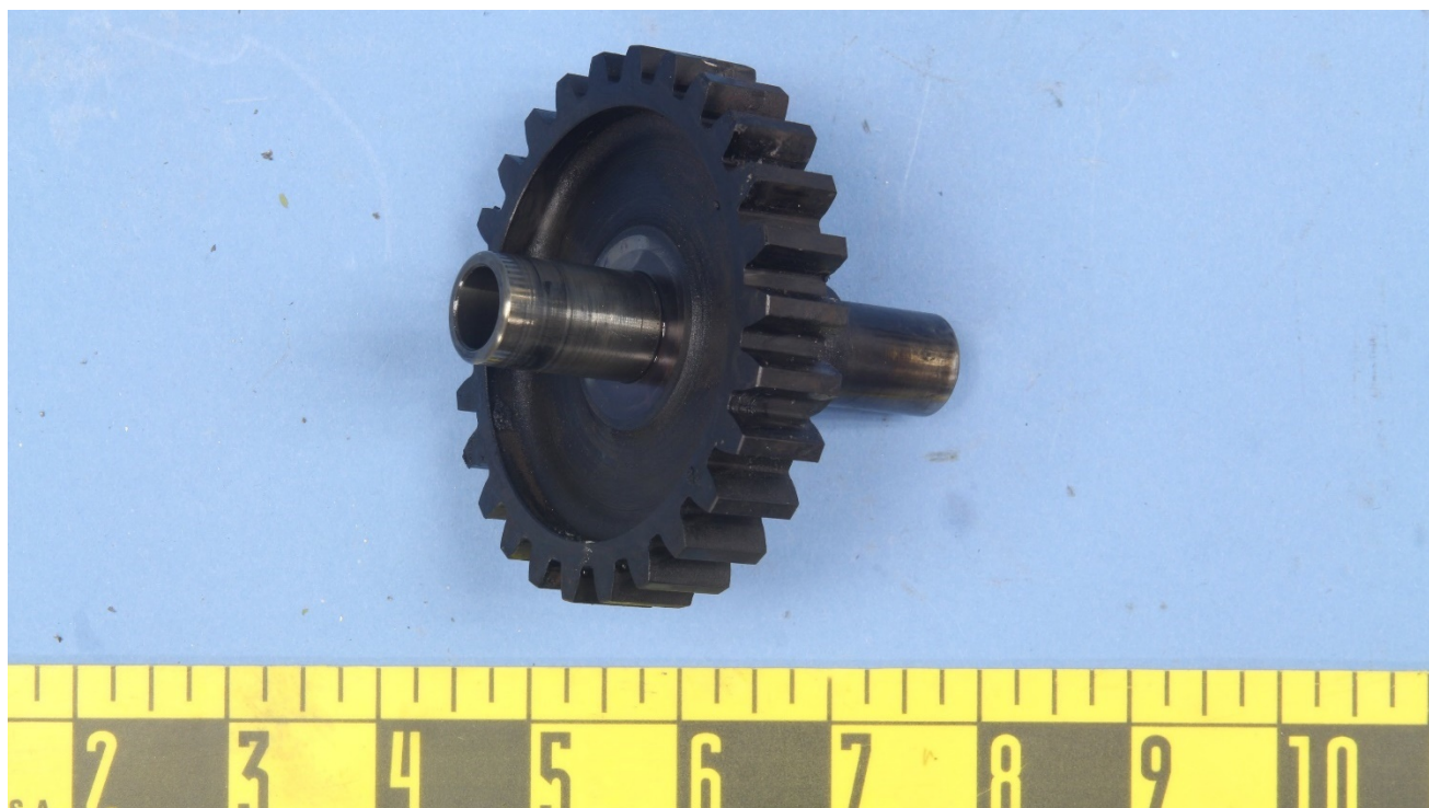
Figure 1 – The bottom right hand assembly gear, as received.
