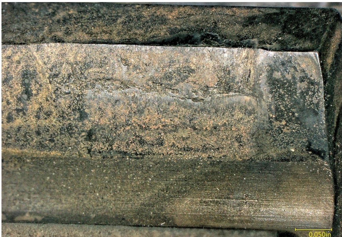
Figure 9 – Closer view of the imprint on a gear tooth flank in Figure 8.
