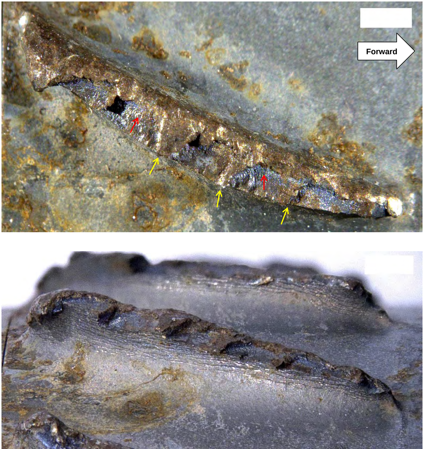
Figure 71. Detailed views of the fracture surface (top) and suction side surface (bottom) of stage 6 compressor blade 8 (see Figures 62 and 63). The red arrows indicate the local direction of fatigue progression. The yellow arrows indicate ratchet marks consistent with fatigue initiation on the suction side surface.
