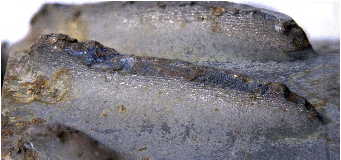
Figure 82. Detailed views of the fracture surface (top) and suction side surface (bottom) of stage 6 compressor blade 19 (see Figures 62 and 63). The red arrows indicate the local direction of fatigue progression. The yellow arrows indicate ratchet marks consistent with fatigue initiation on the suction side surface.
