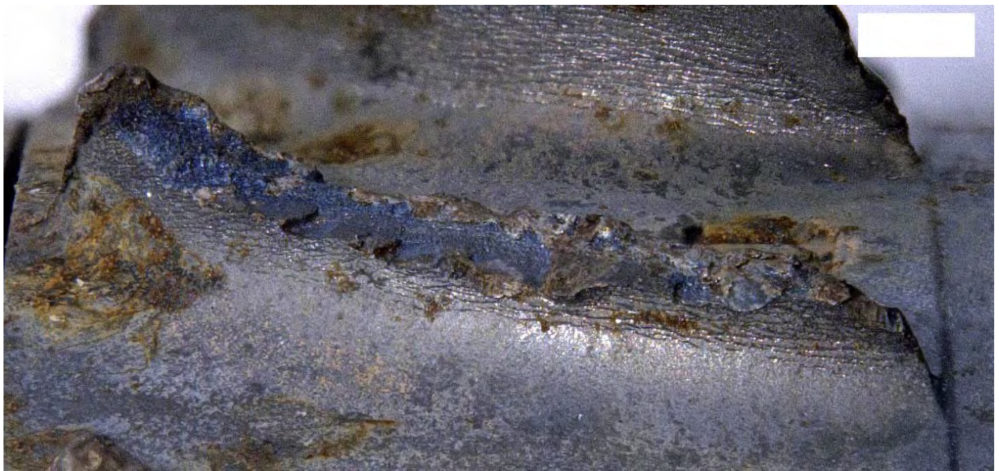
Figure 86. Detailed views of the fracture surface (top) and suction side surface (bottom) of stage 6 compressor blade 23 (see Figures 62 and 63). The red arrows indicate the local direction of fatigue progression. The yellow arrows indicate ratchet marks consistent with fatigue initiation on the suction side surface.
