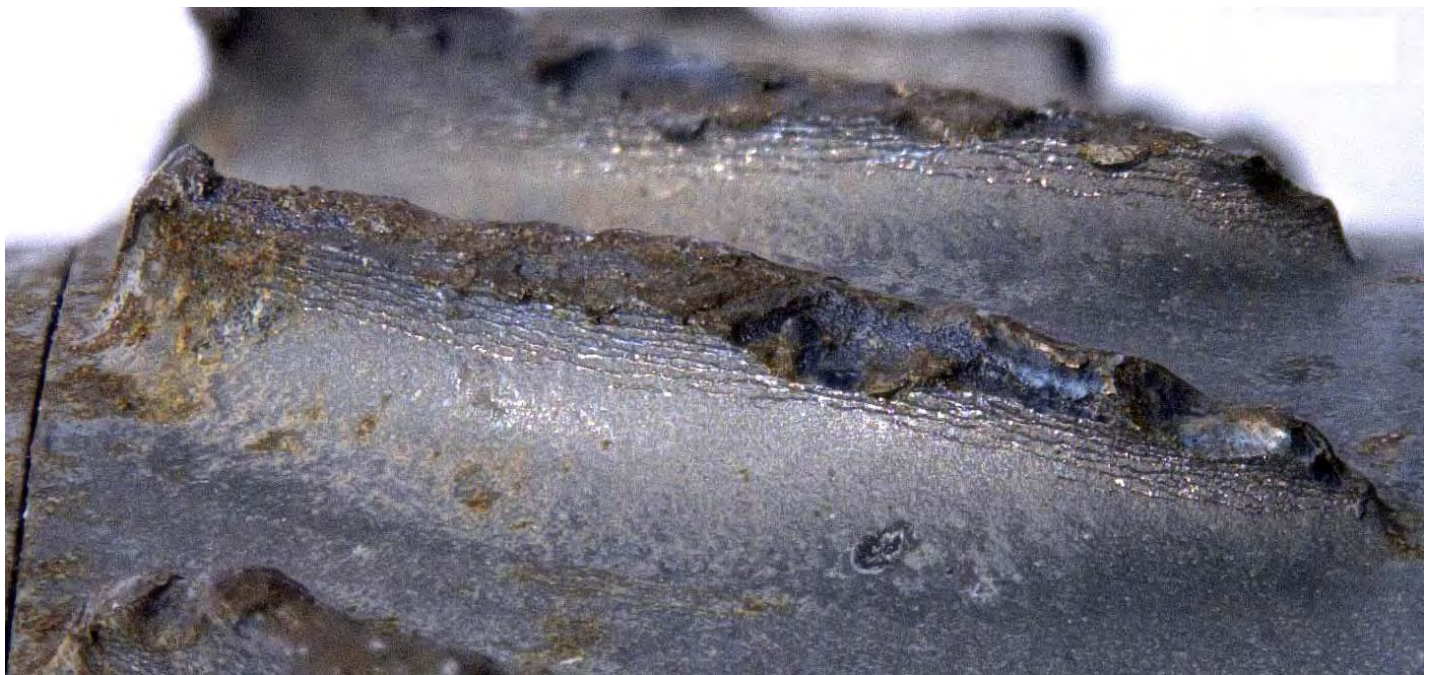
Figure 73. Detailed views of the fracture surface (top) and suction side surface (bottom) of stage 6 compressor blade 10 (see Figures 62 and 63). The red arrows indicate the direction of fatigue progression. The yellow arrow indicates a ratchet mark consistent with fatigue initiation on the suction side surface.
