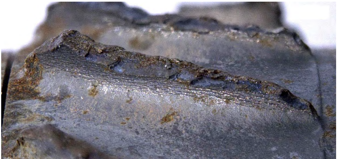
Figure 77. Detailed views of the fracture surface (top) and suction side surface (bottom) of stage 6 compressor blade 14 (see Figures 62 and 63). The red arrows indicate the local direction of fatigue progression. The yellow arrows indicate ratchet marks consistent with fatigue initiation on the suction side surface.
