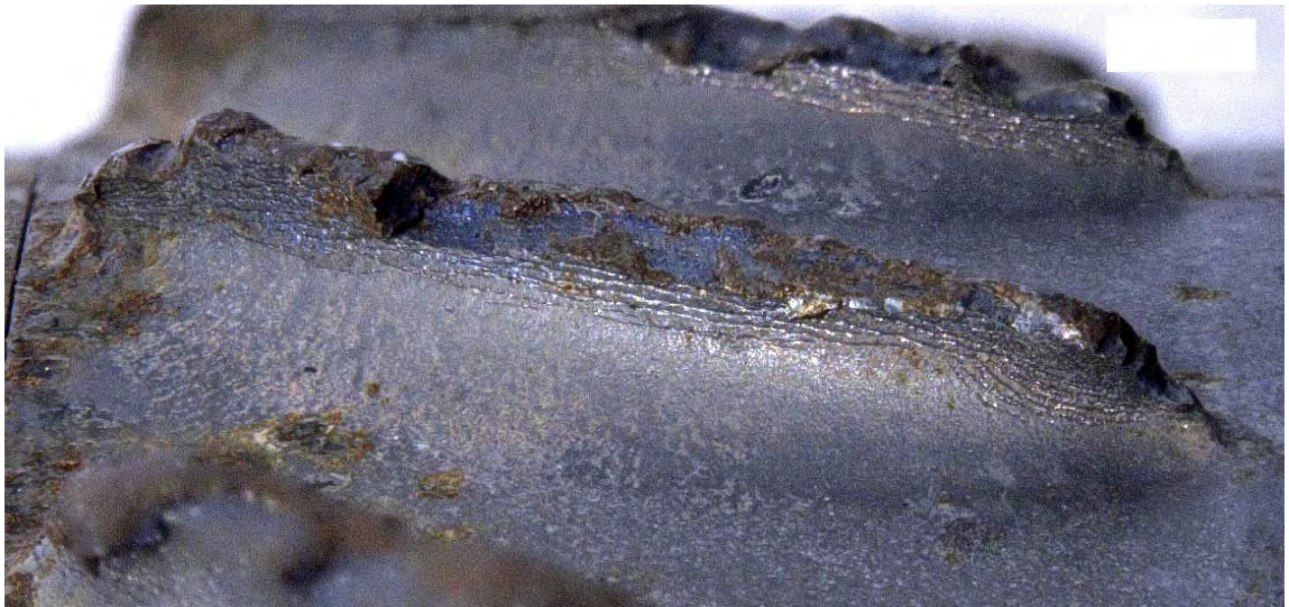
Figure 72. Detailed views of the fracture surface (top) and suction side surface (bottom) of stage 6 compressor blade 9 (see Figures 62 and 63). The red arrows indicate the direction of fatigue progression. The yellow arrows indicate ratchet marks consistent with fatigue initiation on the suction side surface.
