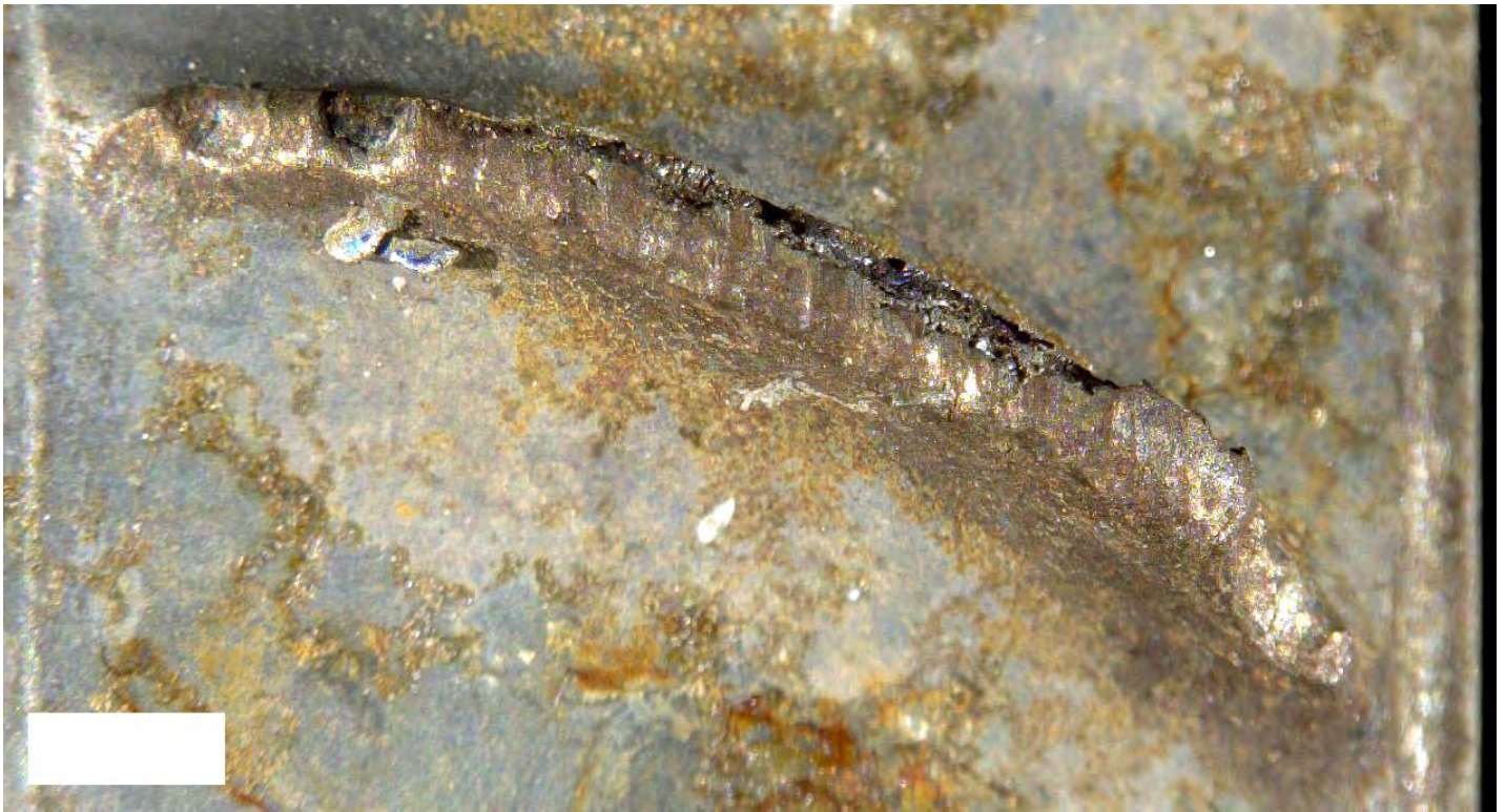
Figure 61. Detailed views of two stage 5 blade fracture surfaces. No fatigue fracture features were present on either of the fracture surfaces.
