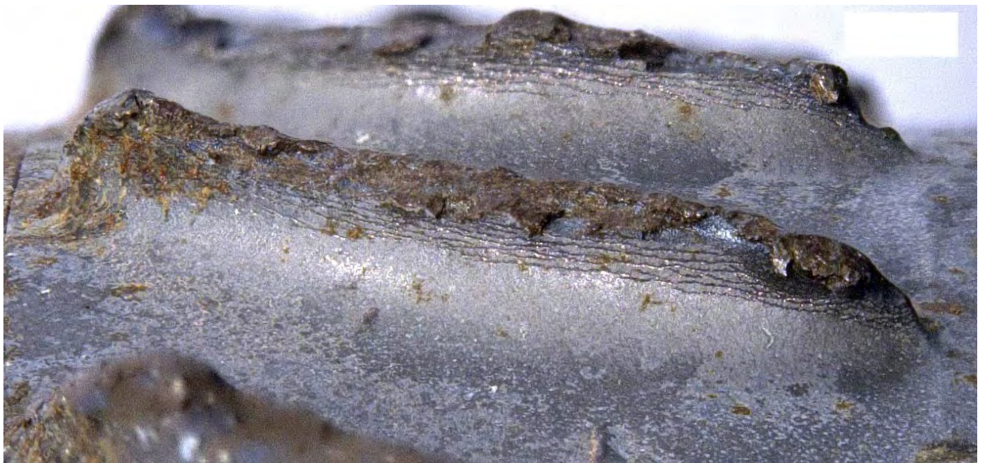
Figure 69. Detailed views of the fracture surface (top) and suction side surface (bottom) of stage 6 compressor blade 6 (see Figures 62 and 63). The red arrow indicates the local direction of fatigue progression. The yellow arrows indicate ratchet marks consistent with fatigue initiation on the suction side surface.
