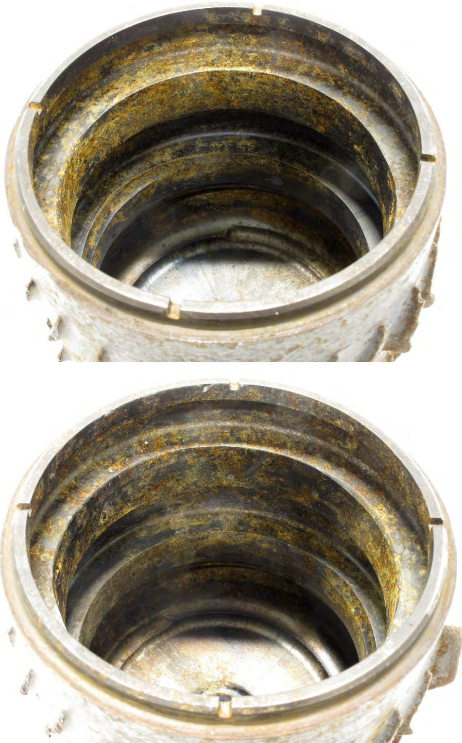
Figure 34. Inner diameter of the stage 4 through 6 compressor wheels after separation from the stage 1 through 3 compressor wheels. Each image shows the component rotated approximately 180° from the previous. Generalized corrosion was present on the majority of the inner diameter.
