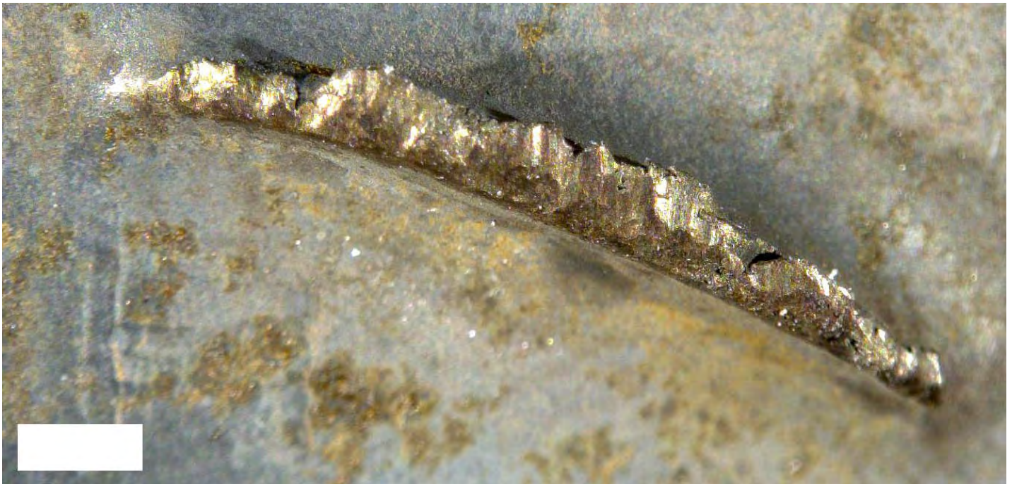
Figure 41. Detailed views of two stage 4 blade fracture surfaces. No fatigue fracture features were present on either of the fracture surfaces.
