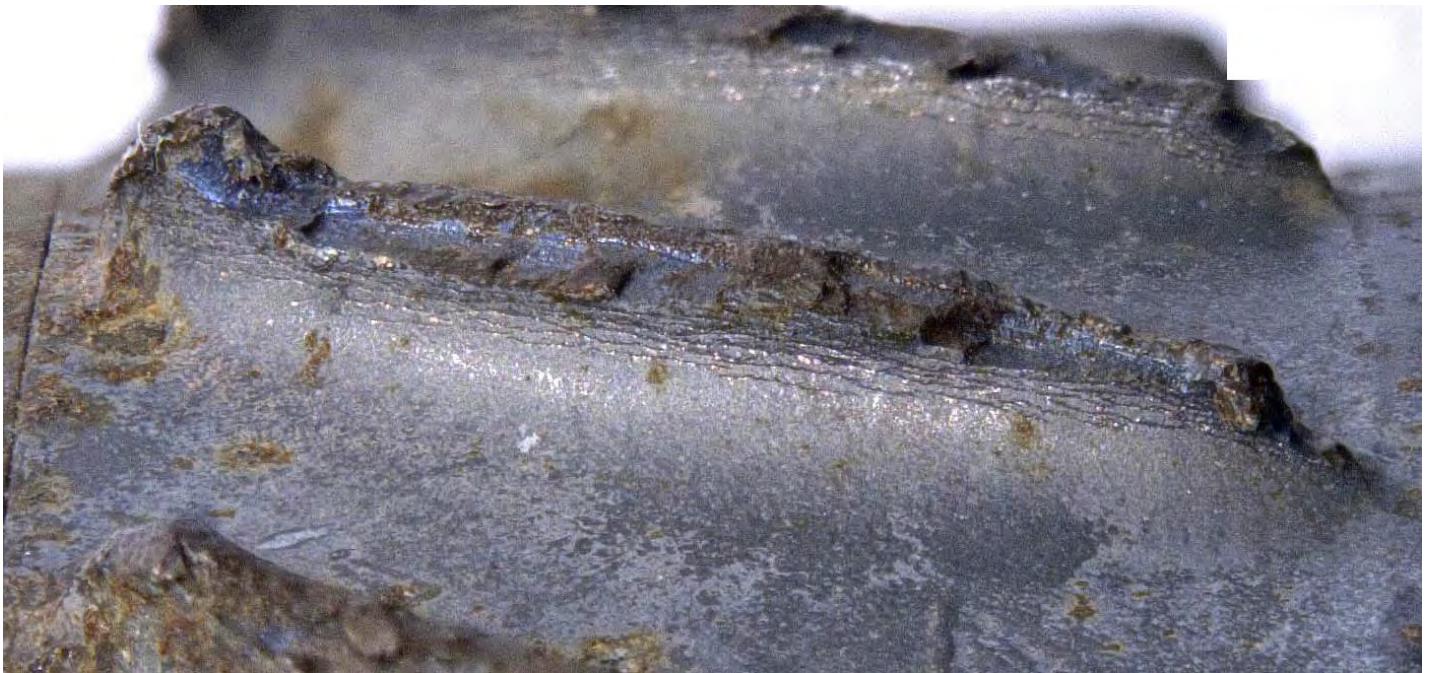
Figure 70. Detailed views of the fracture surface (top) and suction side surface (bottom) of stage 6 compressor blade 7 (see Figures 62 and 63). The red arrows indicate the local direction of fatigue progression. The yellow arrows indicate ratchet marks consistent with fatigue initiation on the suction side surface.
