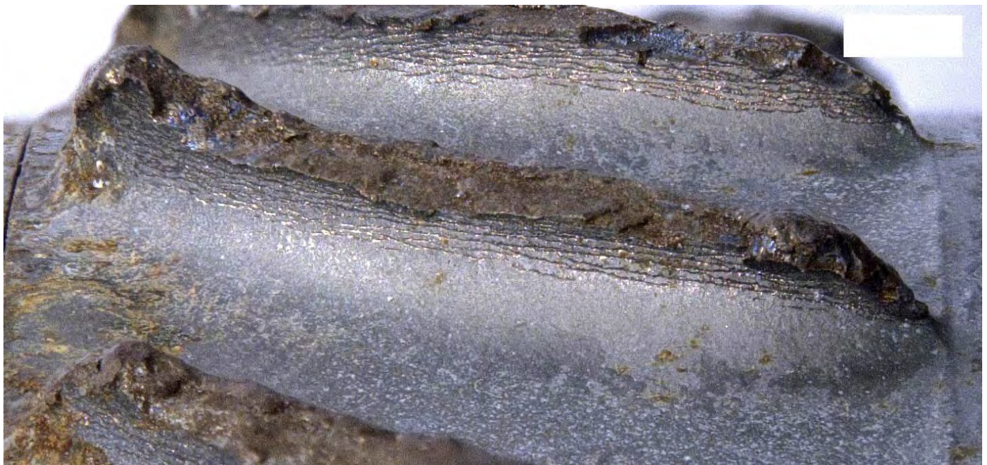
Figure 67. Detailed views of the fracture surface (top) and suction side surface (bottom) of stage 6 compressor blade 4 (see Figures 62 and 63). The red arrow indicates the local direction of fatigue progression. The yellow arrows indicate ratchet marks consistent with fatigue initiation on the suction side surface.
