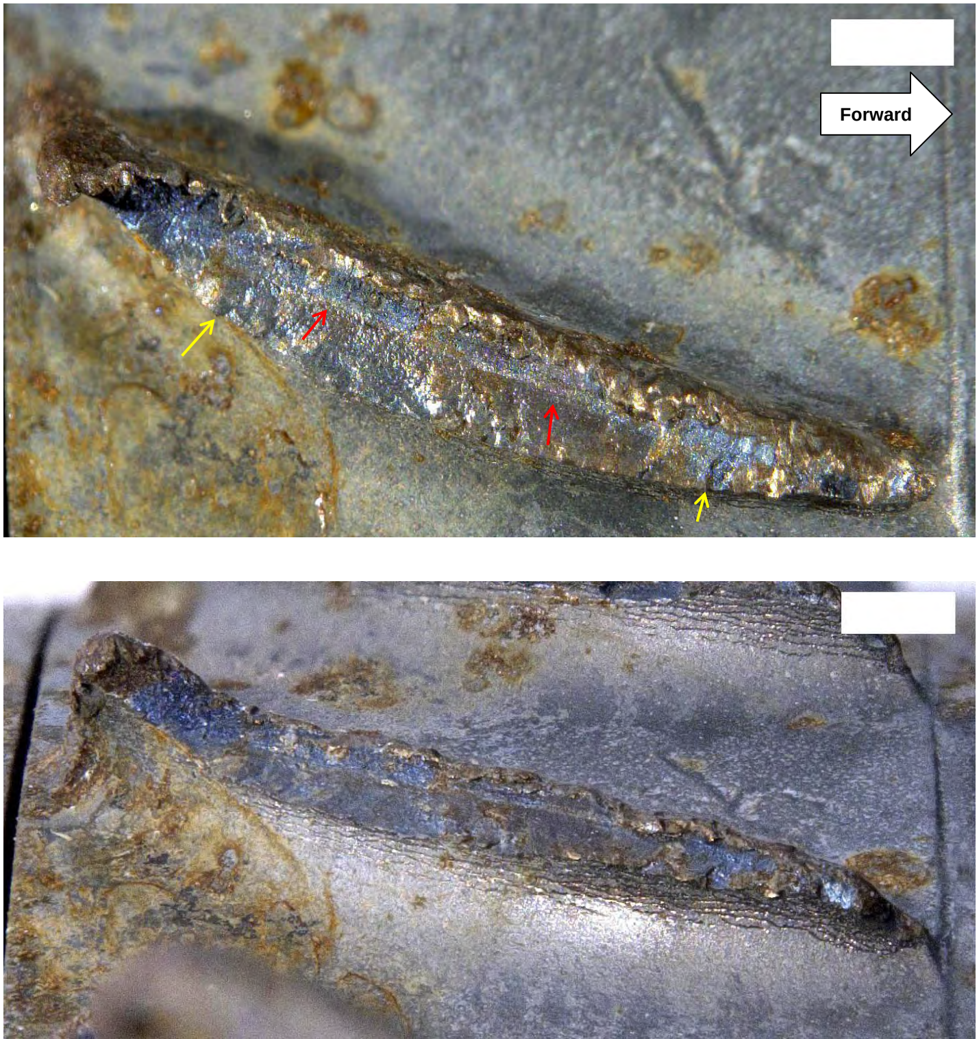
Figure 88. Detailed views of the fracture surface (top) and suction side surface (bottom) of stage 6 compressor blade 25 (see Figures 62 and 63). The red arrows indicate the local direction of fatigue progression. The yellow arrows indicate ratchet marks consistent with fatigue initiation on the suction side surface.
