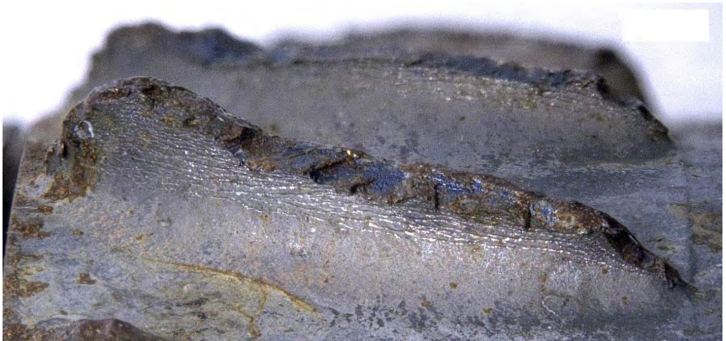
Figure 81. Detailed views of the fracture surface (top) and suction side surface (bottom) of stage 6 compressor blade 18 (see Figures 62 and 63). The red arrows indicate the local direction of fatigue progression. The yellow arrows indicate ratchet marks consistent with fatigue initiation on the suction side surface.
