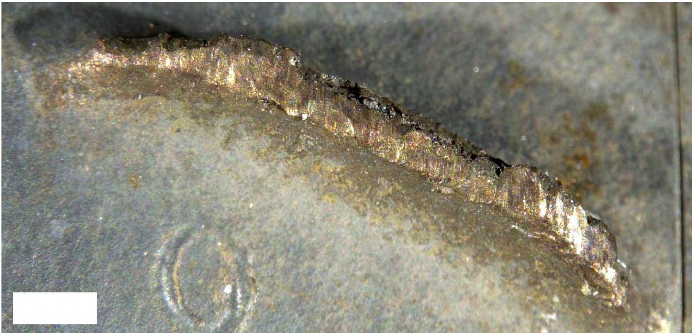
Figure 45. Detailed views of two stage 4 blade fracture surfaces. No fatigue fracture features were present on either of the fracture surfaces.
