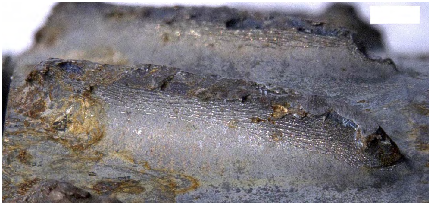
Figure 83. Detailed views of the fracture surface (top) and suction side surface (bottom) of stage 6 compressor blade 20 (see Figures 62 and 63). The red arrows indicate the local direction of fatigue progression. The yellow arrows indicate ratchet marks consistent with fatigue initiation on the suction side surface.
