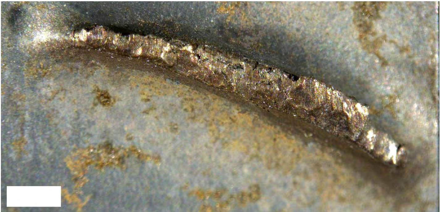
Figure 37. Detailed views of two stage 4 blade fracture surfaces. No fatigue fracture features were present on either of the fracture surfaces.
