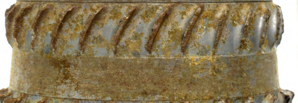
Figure 31. Detailed radial views of the stage 4 and 5 compressor wheels, while still in the rotor stack. Each image shows the rotor rotated approximately 90° from the previous.
