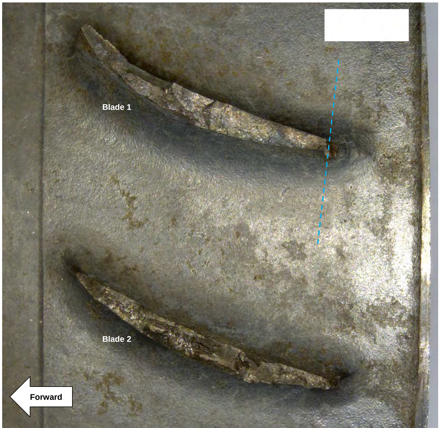
Figure 13. Detailed radial views of the fracture surfaces of the two liberated stage 3 compressor blades. The blue dashed line shows the approximate plane of metallographic cross section shown in Figure 23.
