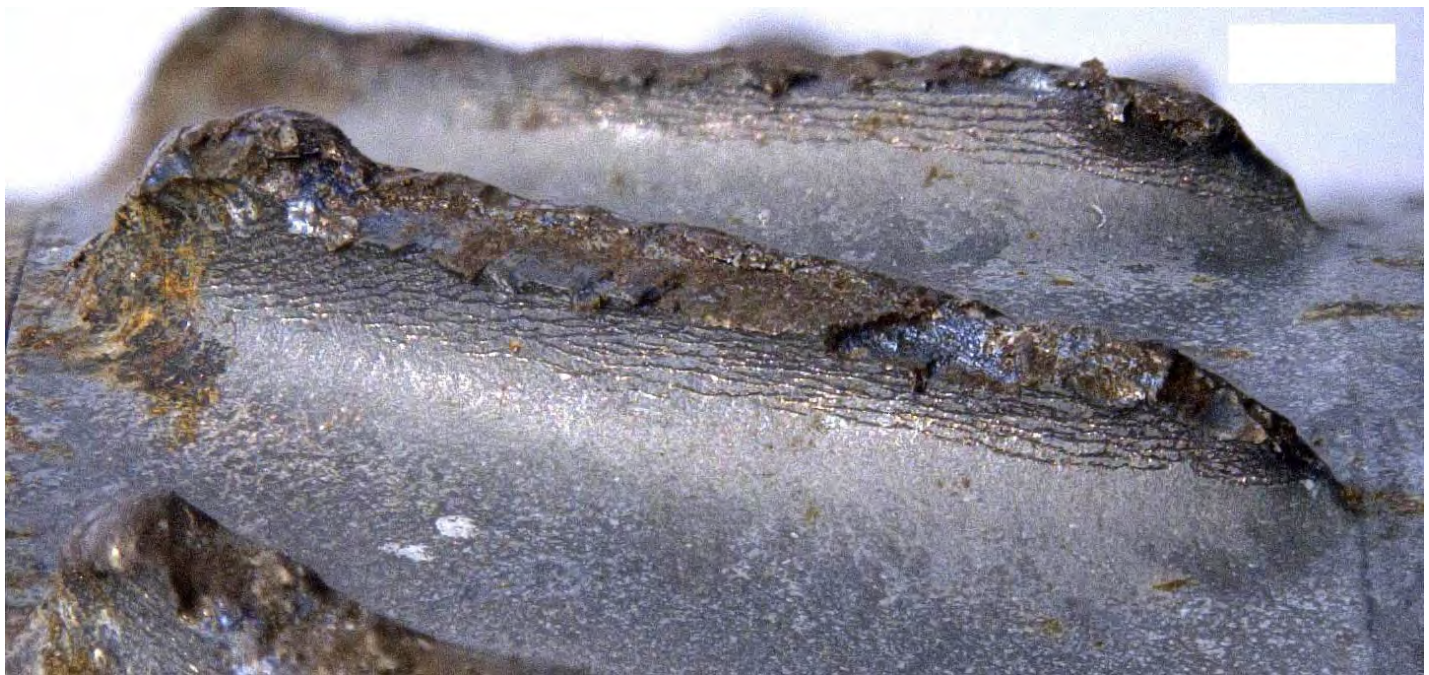
Figure 68. Detailed views of the fracture surface (top) and suction side surface (bottom) of stage 6 compressor blade 5 (see Figures 62 and 63). The red arrows indicate the direction of fatigue progression.
