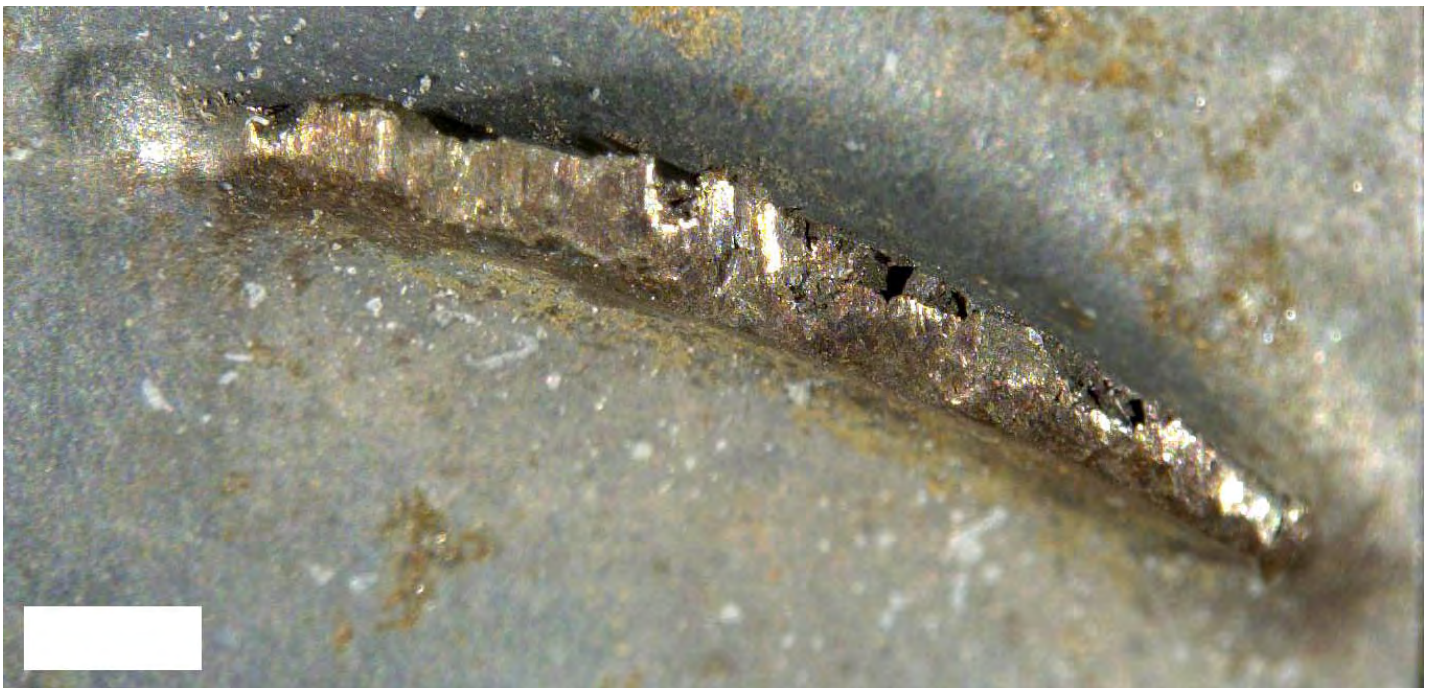
Figure 46. Detailed views of two stage 4 blade fracture surfaces. No fatigue fracture features were present on either of the fracture surfaces.
