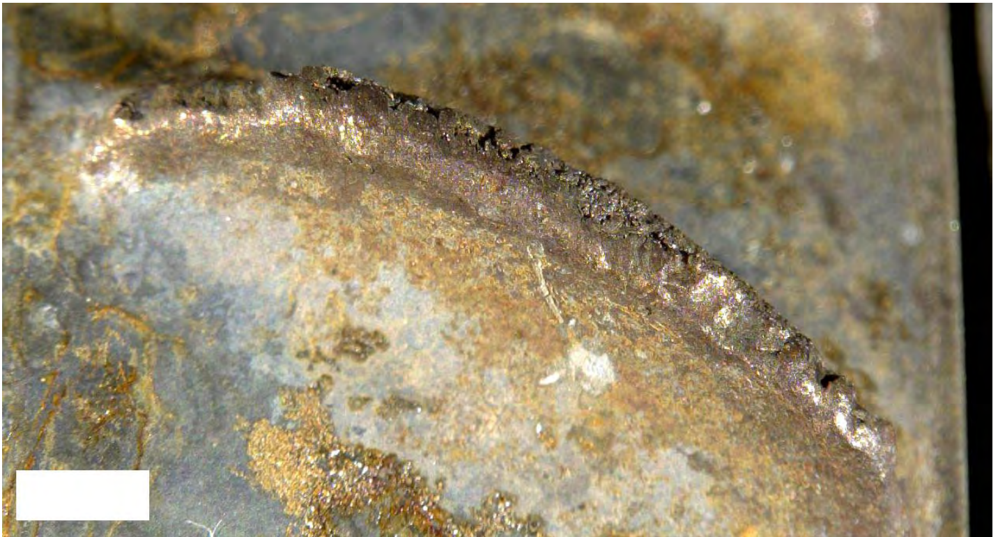
Figure 60. Detailed views of two stage 5 blade fracture surfaces. No fatigue fracture features were present on either of the fracture surfaces.
