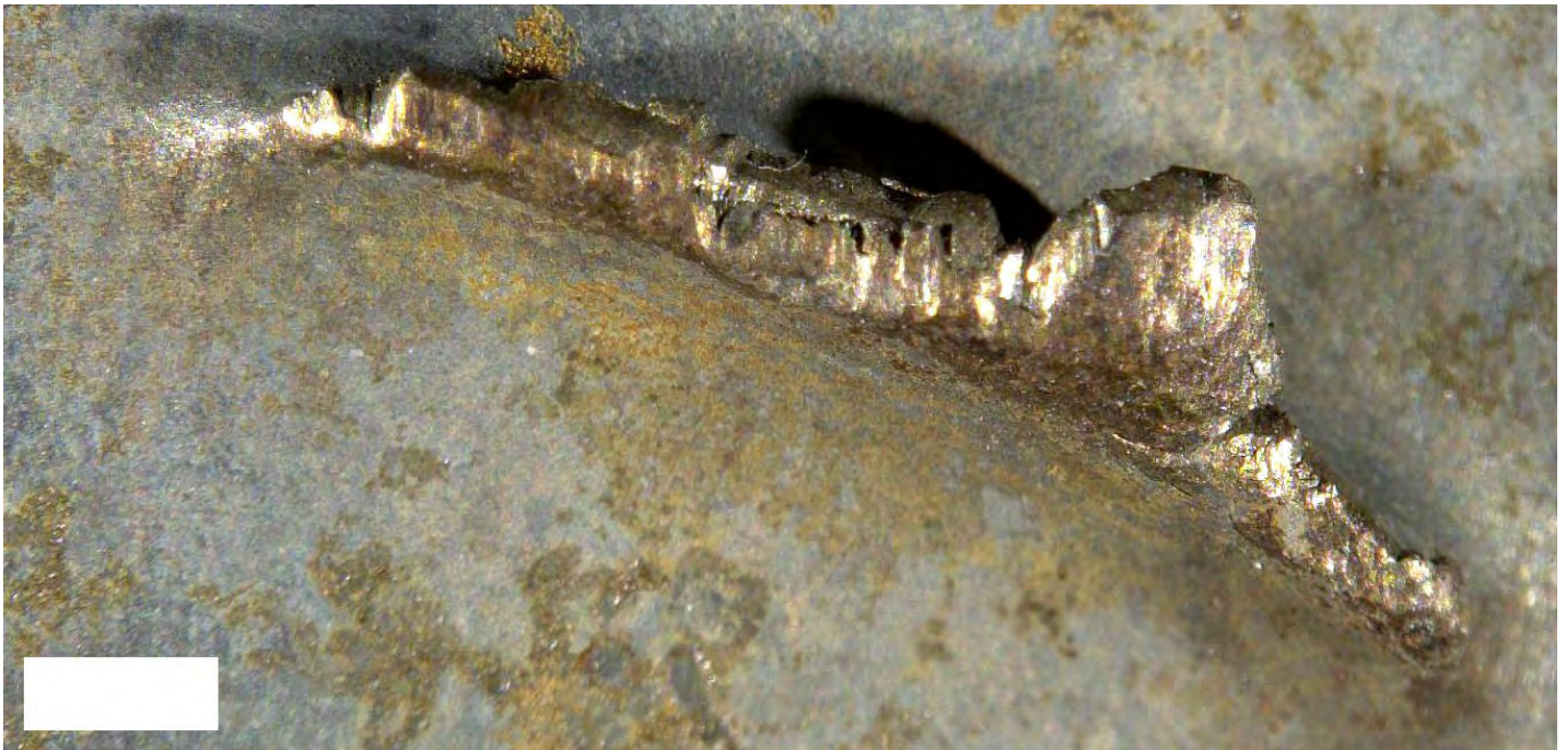
Figure 42. Detailed views of two stage 4 blade fracture surfaces. No fatigue fracture features were present on either of the fracture surfaces.
