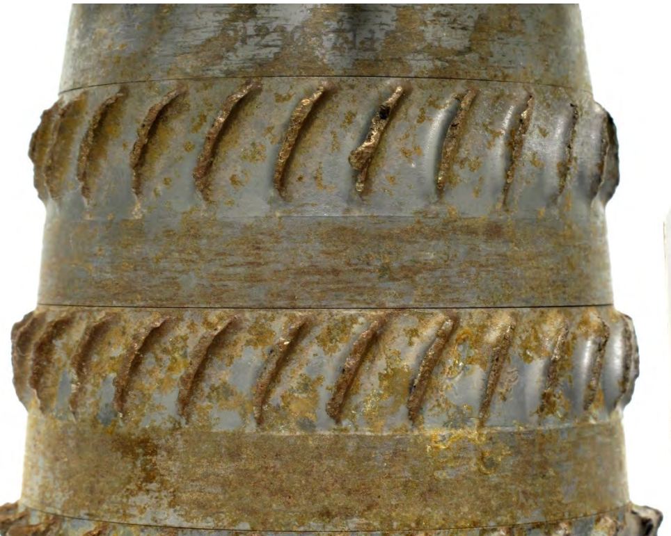
Figure 31. Detailed radial views of the stage 4 and 5 compressor wheels, while still in the rotor stack. Each image shows the rotor rotated approximately 90° from the previous.
