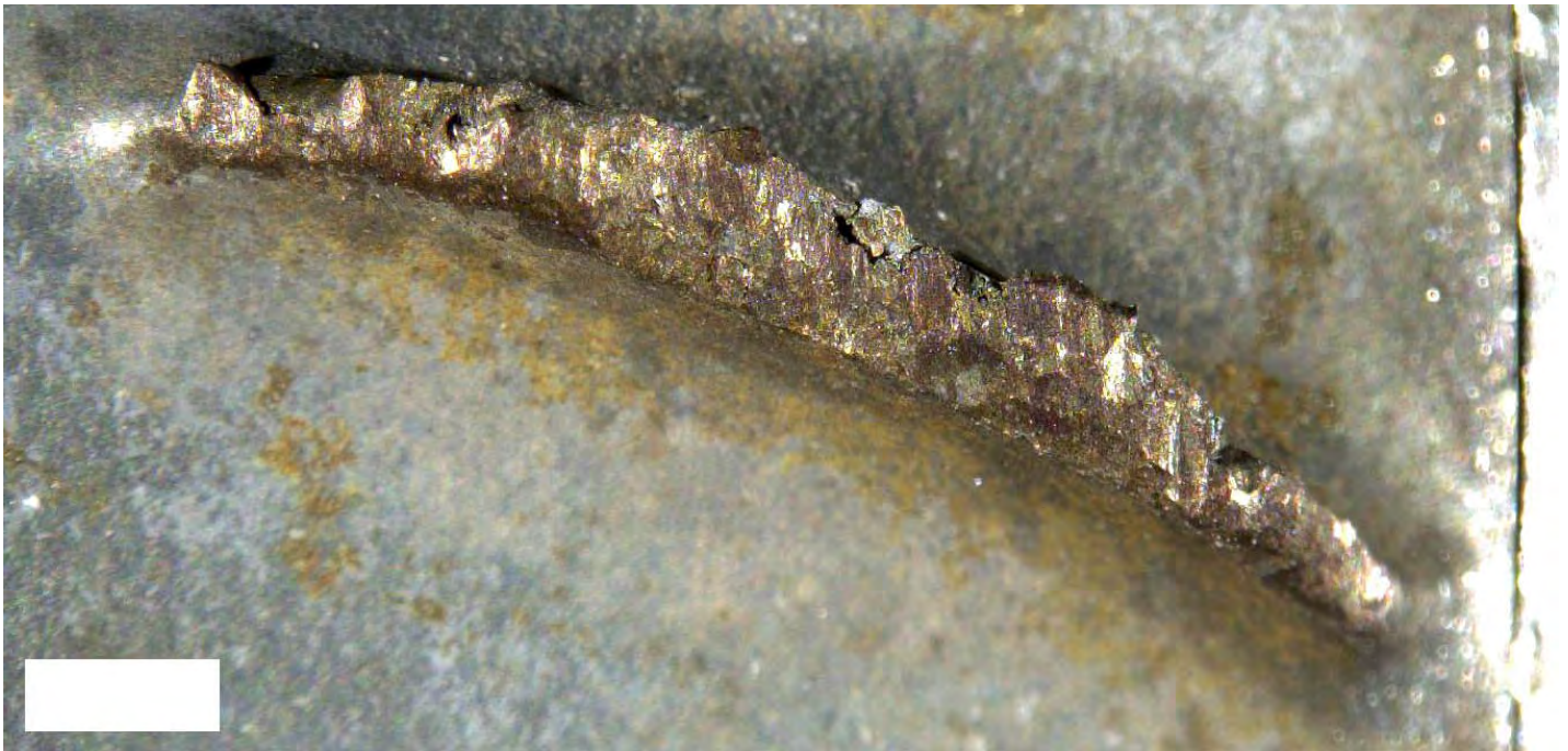
Figure 35. Detailed views of two stage 4 blade fracture surfaces. No fatigue fracture features were present on either of the fracture surfaces.
