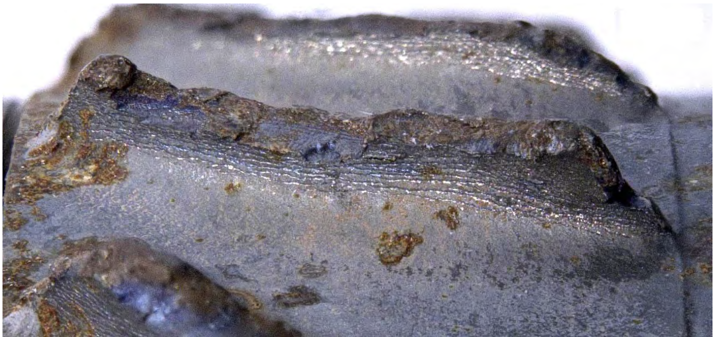
Figure 79. Detailed views of the fracture surface (top) and suction side surface (bottom) of stage 6 compressor blade 16 (see Figures 62 and 63). The red arrows indicate the local direction of fatigue progression. The yellow arrows indicate ratchet marks consistent with fatigue initiation on the suction side surface.
