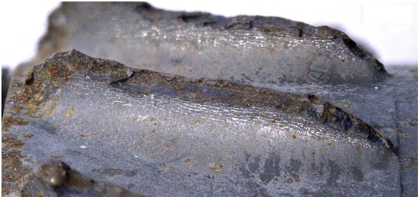
Figure 80. Detailed views of the fracture surface (top) and suction side surface (bottom) of stage 6 compressor blade 17 (see Figures 62 and 63). The red arrows indicate the local direction of fatigue progression. The yellow arrows indicate ratchet marks consistent with fatigue initiation on the suction side surface.
