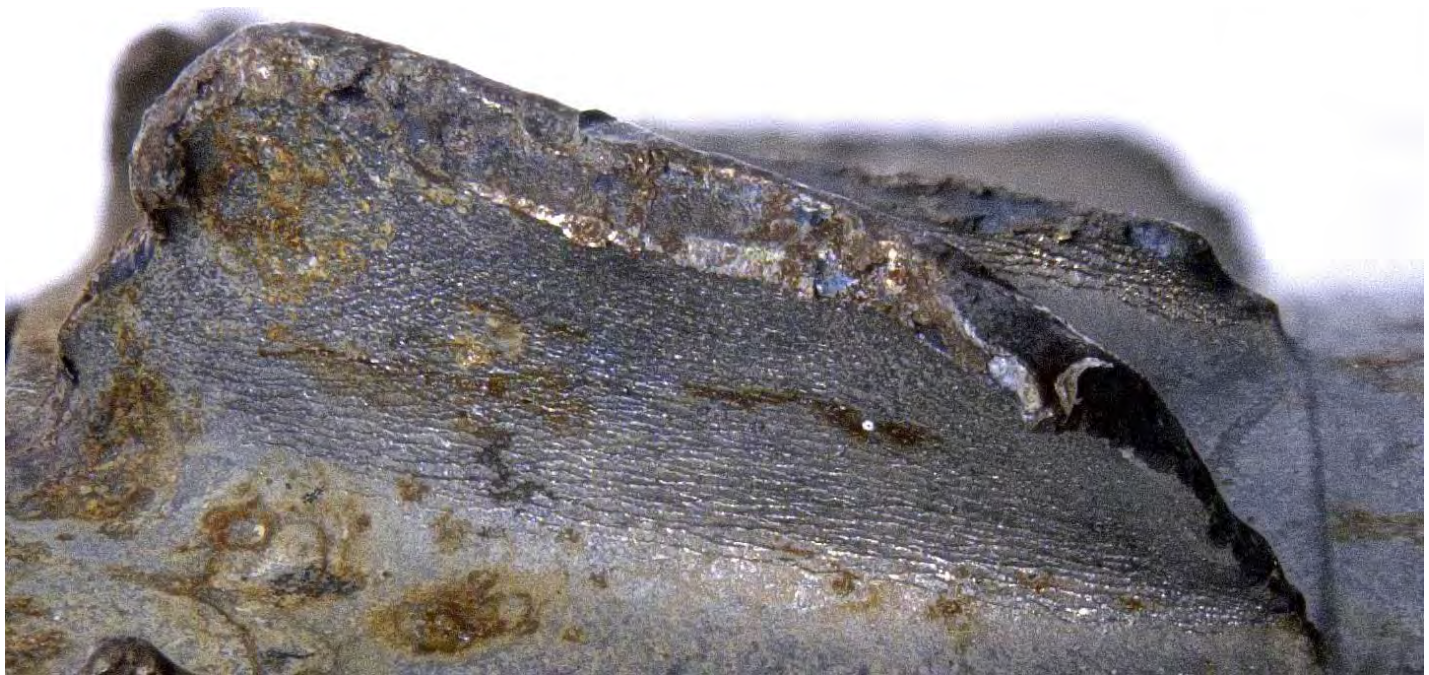
Figure 87. Detailed views of the fracture surface (top) and suction side surface (bottom) of stage 6 compressor blade 24 (see Figures 62 and 63). There were no fatigue progression features on this fracture surface. This blade is shown in more detail in Figures 89 and 90.
