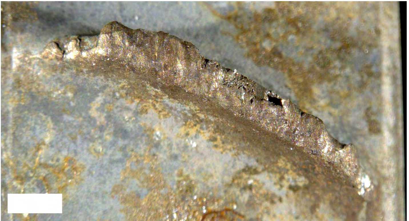
Figure 58. Detailed views of two stage 5 blade fracture surfaces. No fatigue fracture features were present on either of the fracture surfaces.
