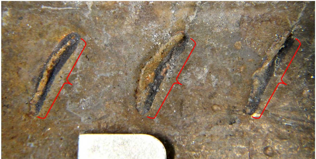
Figure 104. Detailed views of three representative stage 3 (top) and stage 4 (bottom) compressor vane fracture surfaces (red braces), which were completely smeared.
