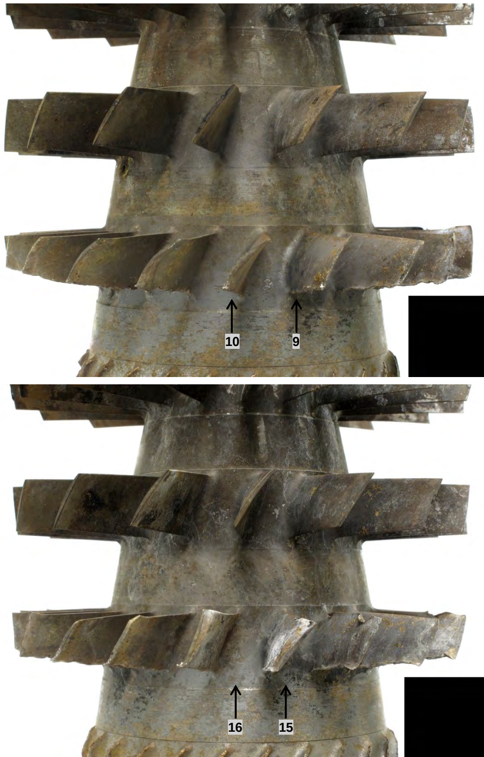
Figure 5. Detailed radial views of the stage 2-3 compressor wheel. Each image shows the wheel rotated approximately 90° from the previous. The black annotations indicate the blade numbering scheme used throughout this report.
