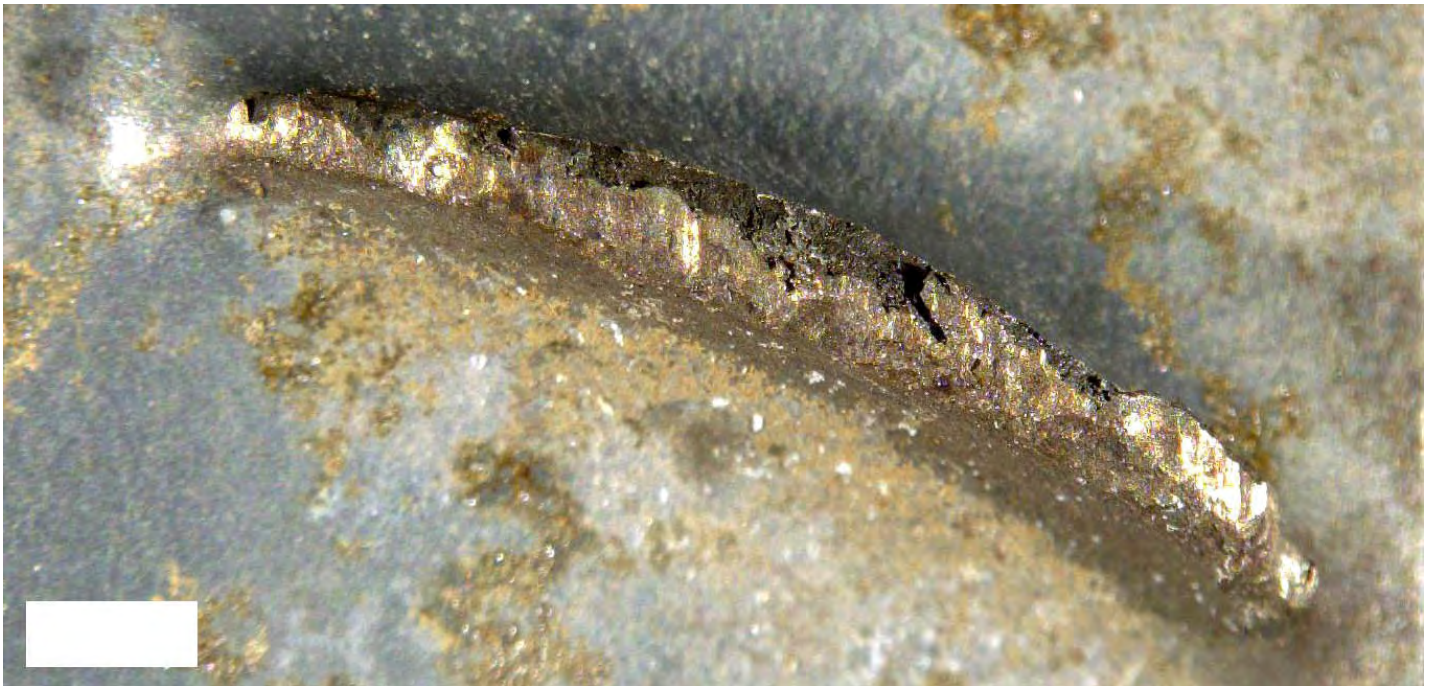
Figure 38. Detailed views of two stage 4 blade fracture surfaces. No fatigue fracture features were present on either of the fracture surfaces.
