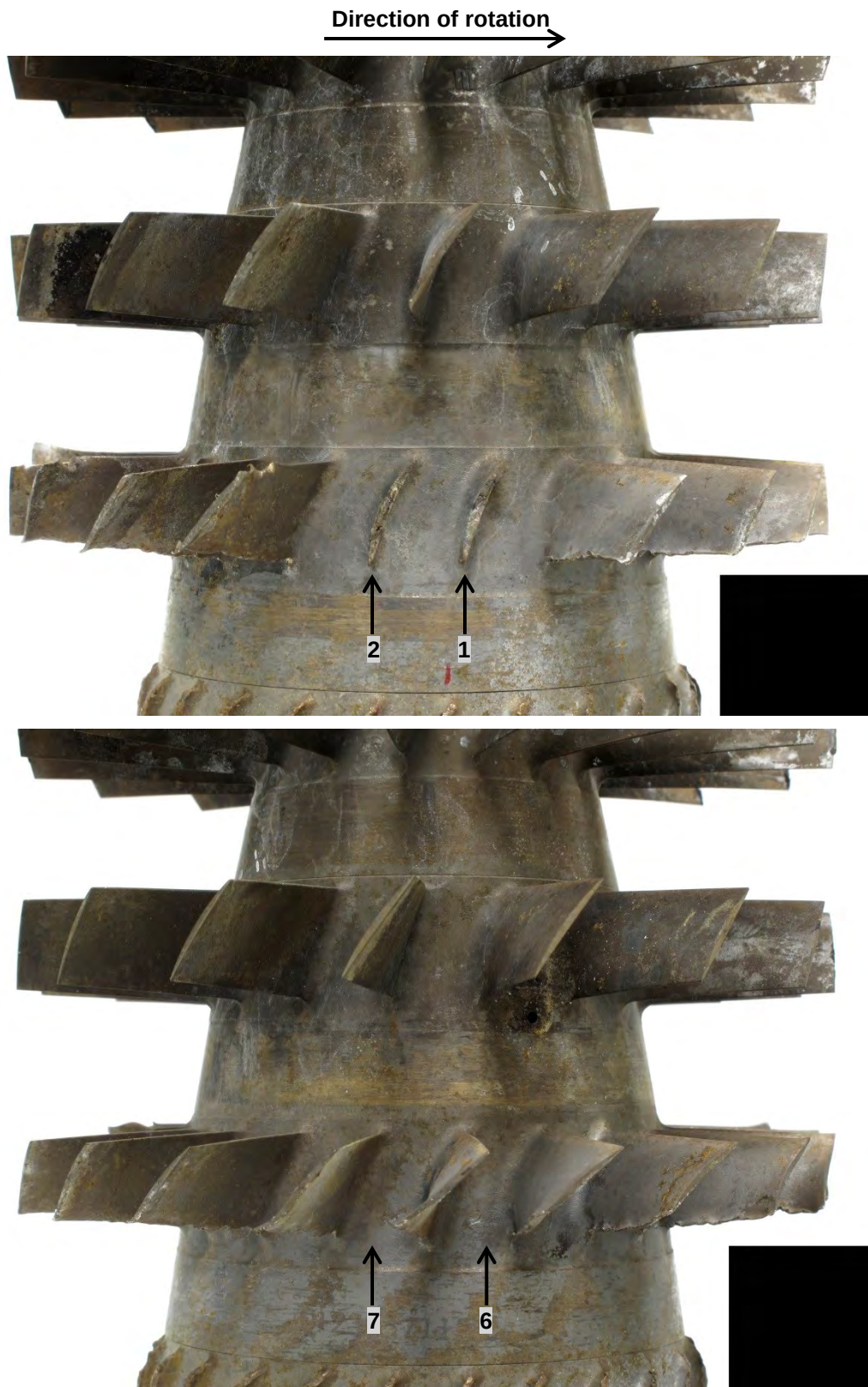
Figure 4. Detailed radial views of the stage 2-3 compressor wheel. Each image shows the wheel rotated approximately 90° from the previous. The black annotations indicate the blade numbering scheme used throughout this report.
