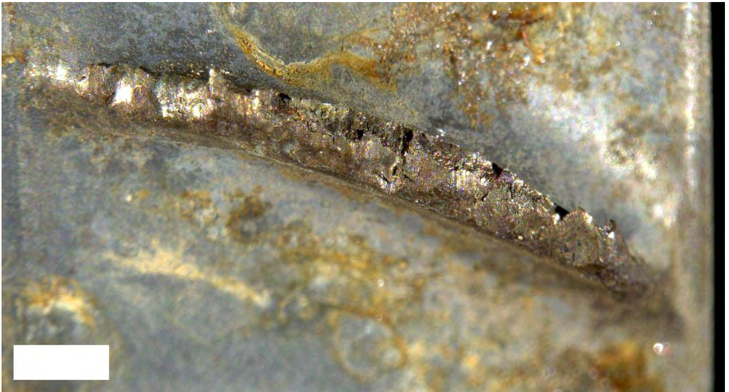
Figure 59. Detailed views of two stage 5 blade fracture surfaces. No fatigue fracture features were present on either of the fracture surfaces.
