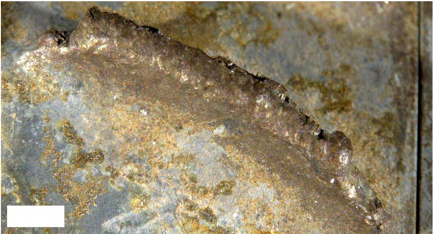
Figure 51. Detailed views of two stage 5 blade fracture surfaces. No fatigue fracture features were present on either of the fracture surfaces.
