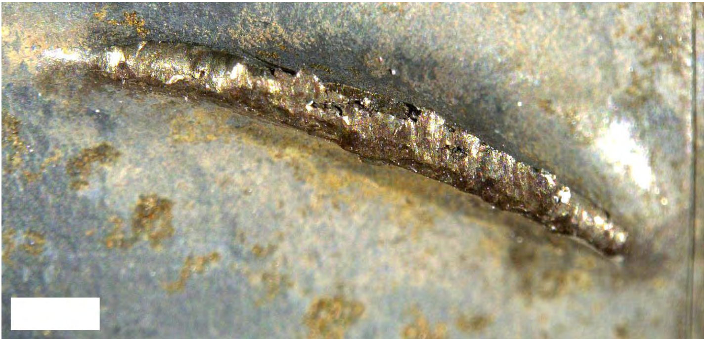
Figure 36. Detailed views of two stage 4 blade fracture surfaces. No fatigue fracture features were present on either of the fracture surfaces.
