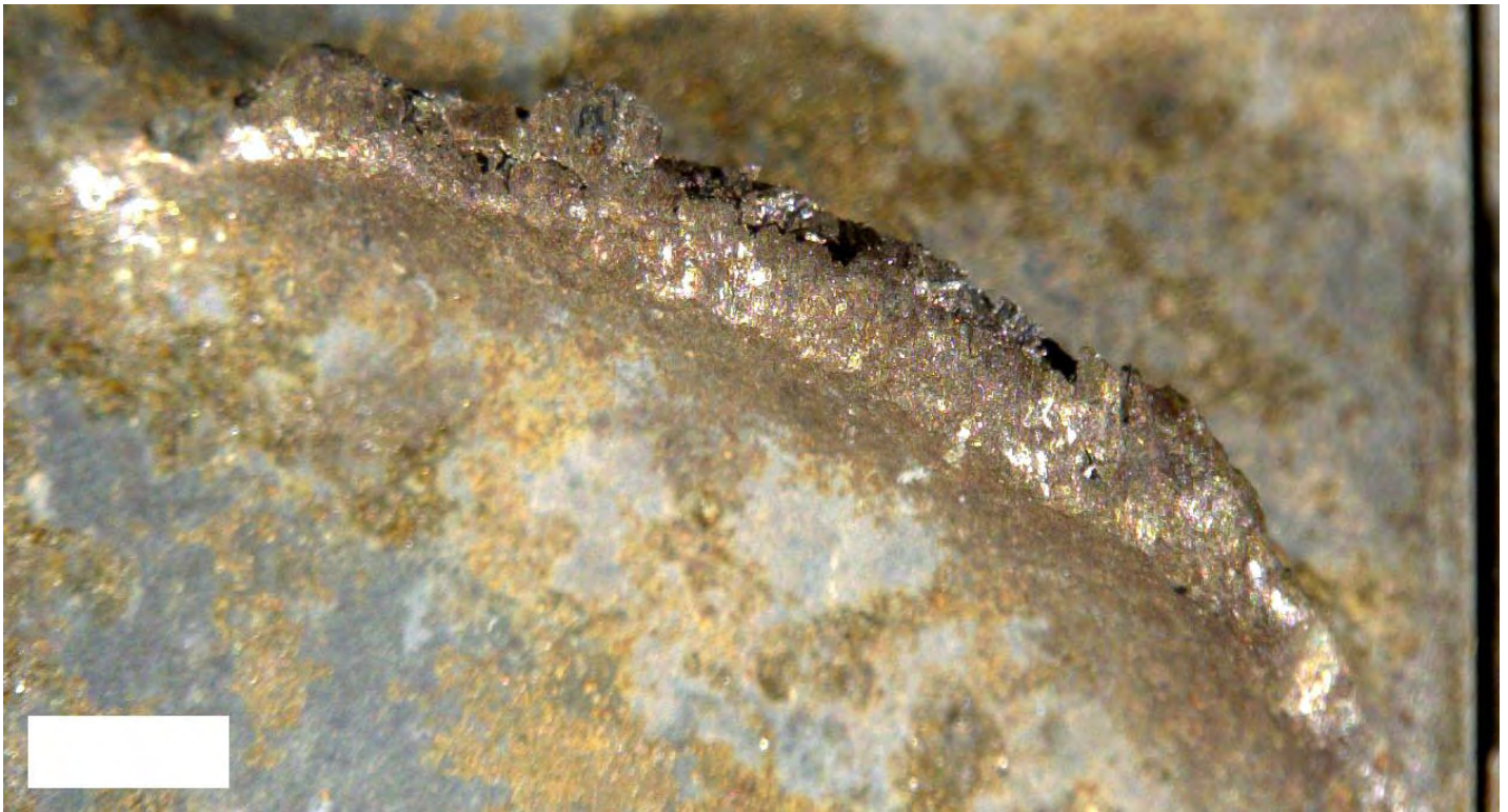
Figure 49. Detailed views of two stage 5 blade fracture surfaces. No fatigue fracture features were present on either of the fracture surfaces.
