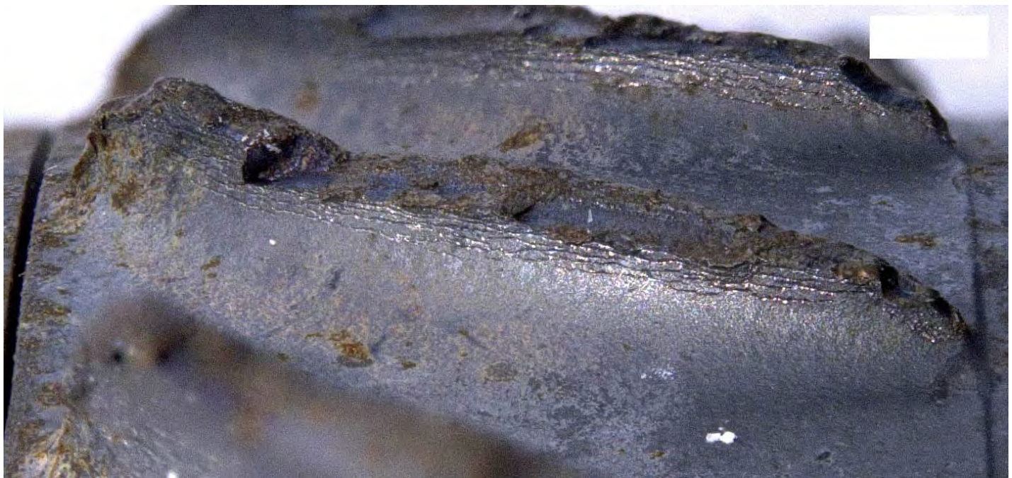
Figure 76. Detailed views of the fracture surface (top) and suction side surface (bottom) of stage 6 compressor blade 13 (see Figures 62 and 63). The red arrows indicate the local direction of fatigue progression. The yellow arrows indicate ratchet marks consistent with fatigue initiation on the suction side surface.
