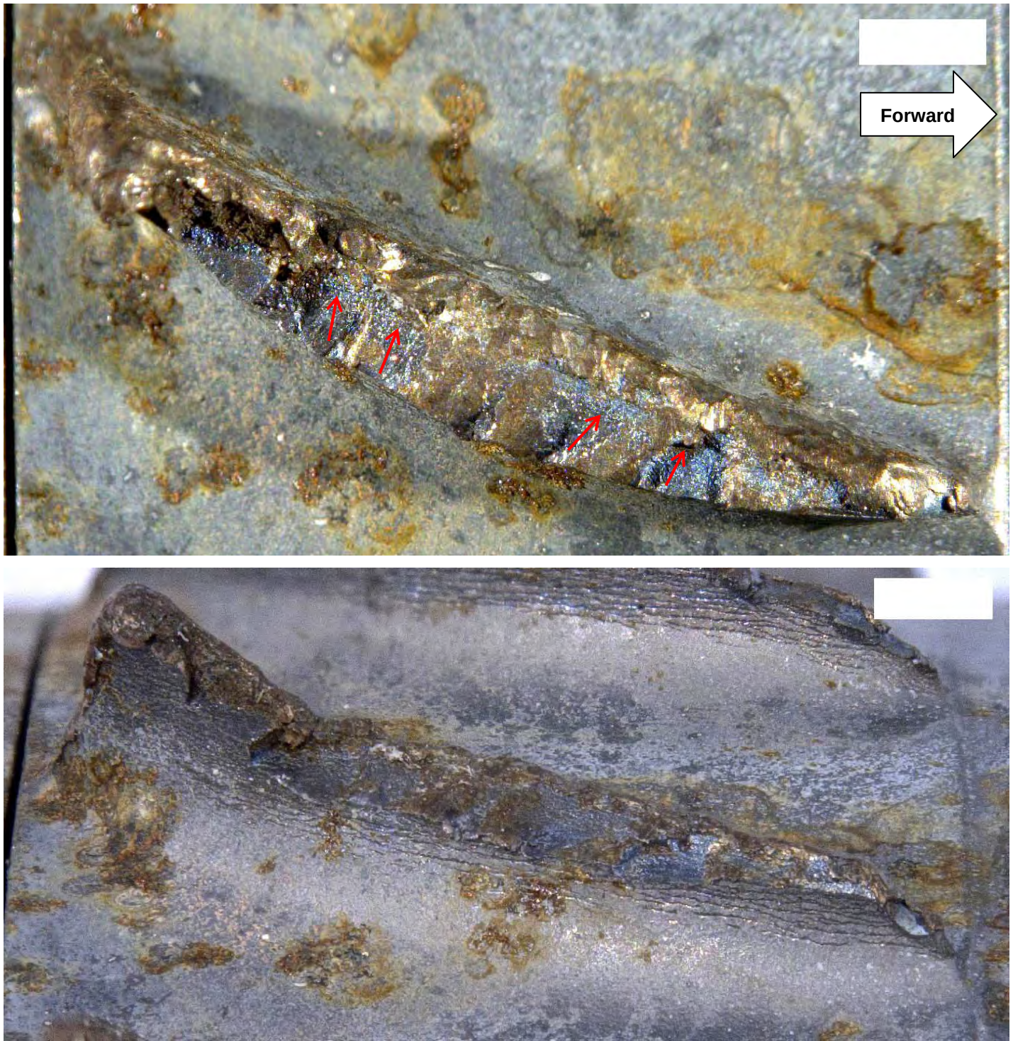
Figure 64. Detailed views of the fracture surface (top) and suction side surface (bottom) of stage 6 compressor blade 1 (see Figures 62 and 63). The red arrows indicate the local direction of fatigue progression.
