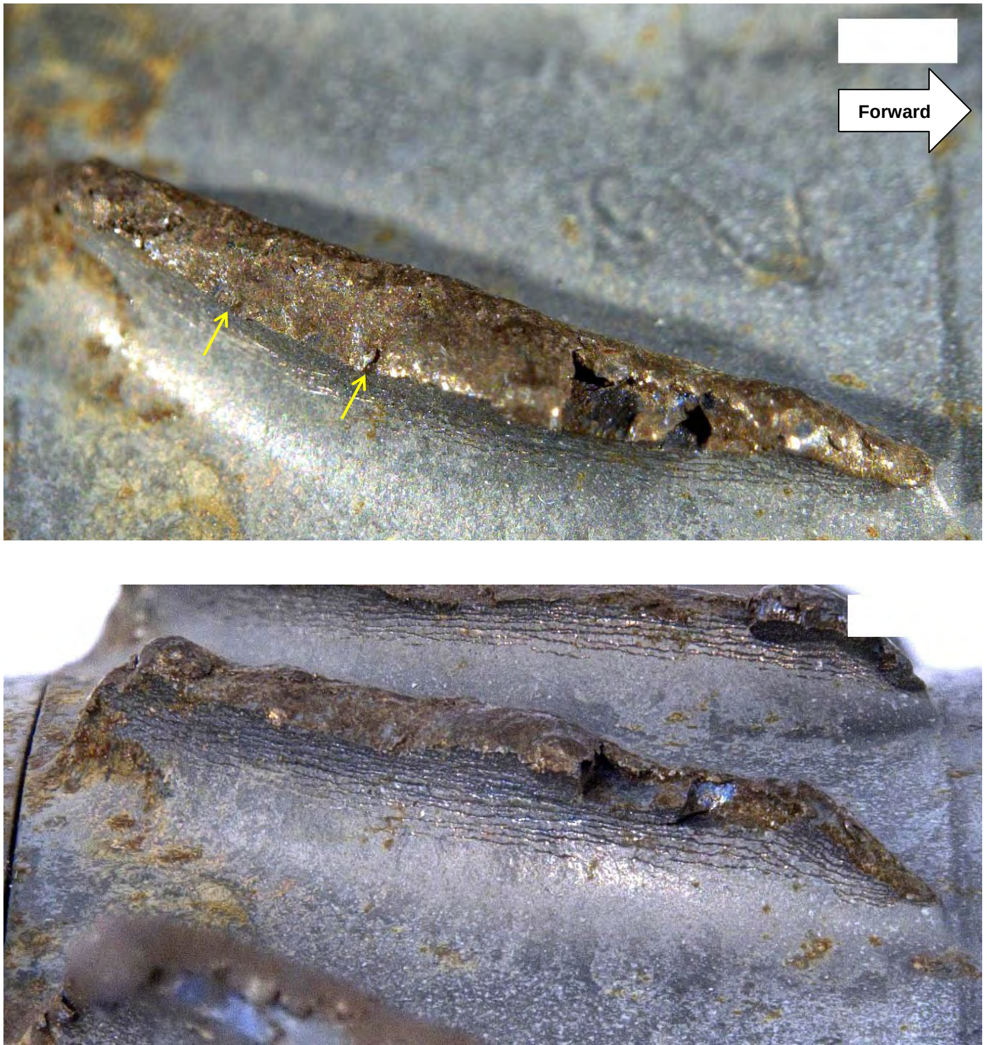
Figure 66. Detailed views of the fracture surface (top) and suction side surface (bottom) of stage 6 compressor blade 3 (see Figures 62 and 63). The yellow arrows indicate ratchet marks consistent with fatigue initiation on the suction side surface.
