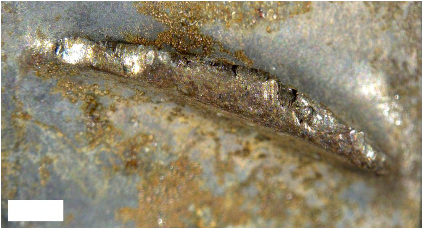
Figure 57. Detailed views of two stage 5 blade fracture surfaces. No fatigue fracture features were present on either of the fracture surfaces.
