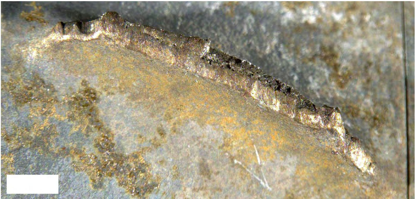
Figure 40. Detailed views of two stage 4 blade fracture surfaces. No fatigue fracture features were present on either of the fracture surfaces.
