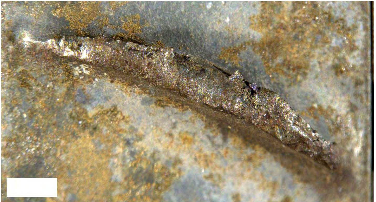
Figure 50. Detailed views of two stage 5 blade fracture surfaces. No fatigue fracture features were present on either of the fracture surfaces.
