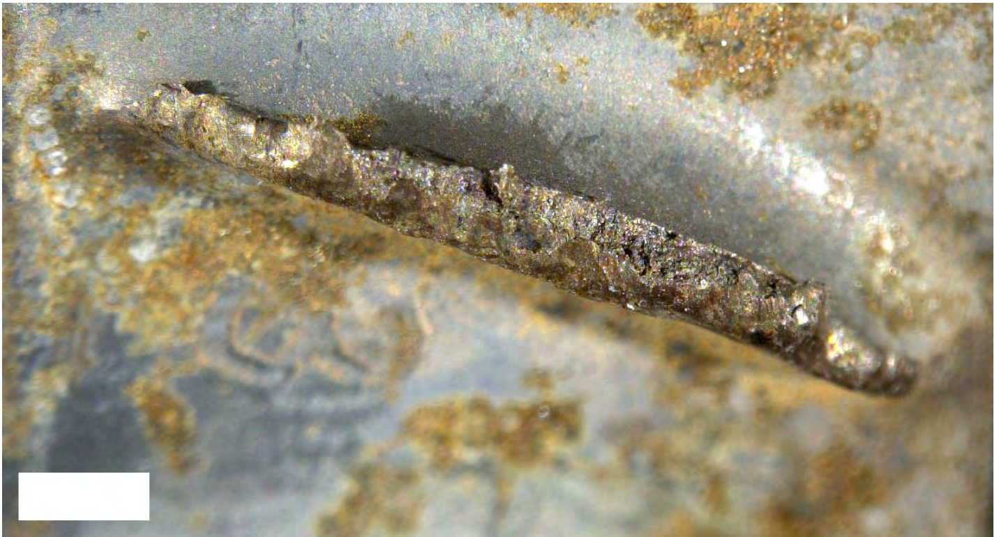
Figure 53. Detailed views of two stage 5 blade fracture surfaces. No fatigue fracture features were present on either of the fracture surfaces.
