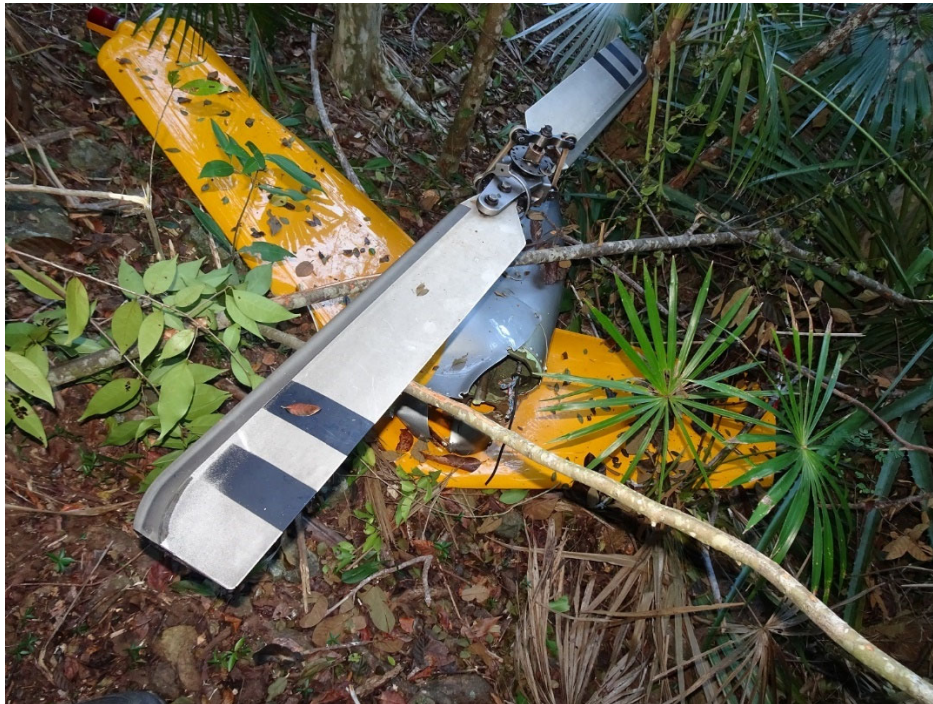
Figure 3. The tail rotor, tail rotor gearbox, and vertical stabilizer at the accident site.
