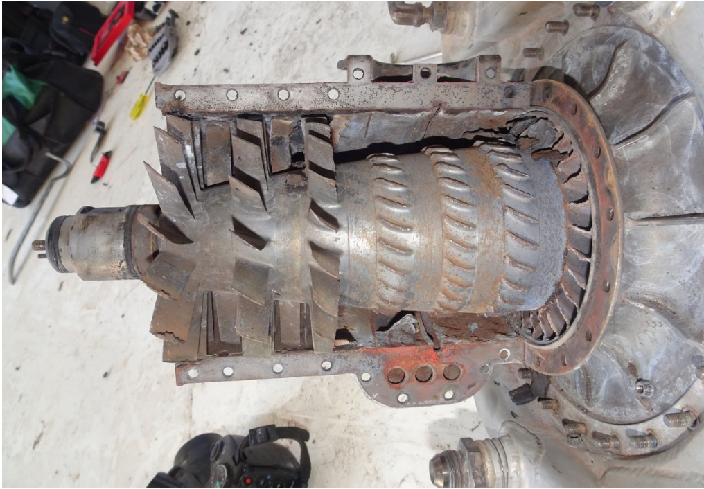
Figure 7. The axial compressor after removal of a case half.
