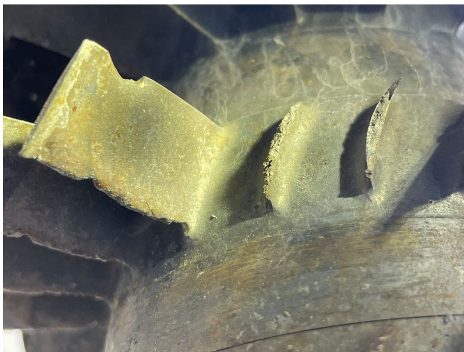
Figure 6. Two fractured stage 3 compressor blades.
