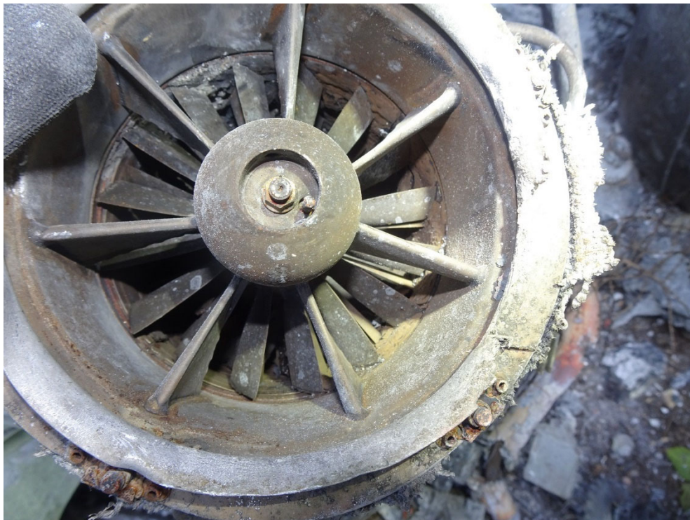
Figure 5. A view of the first stage compressor blades through the engine inlet.
