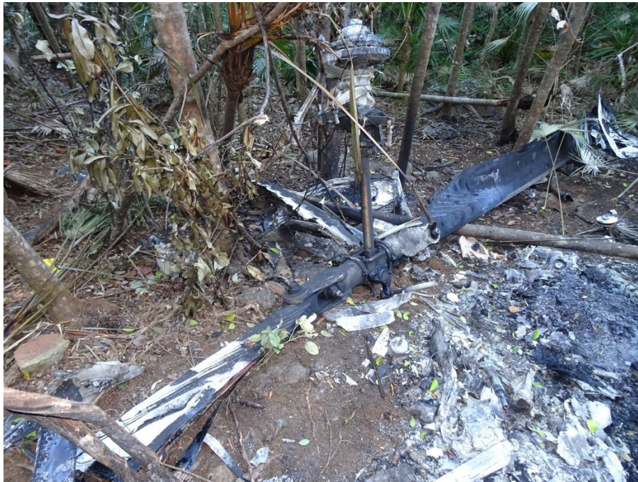
Figure 2. The main rotor, main rotor mast, and a portion of the main rotor gearbox found as an assembly at the accident site.
