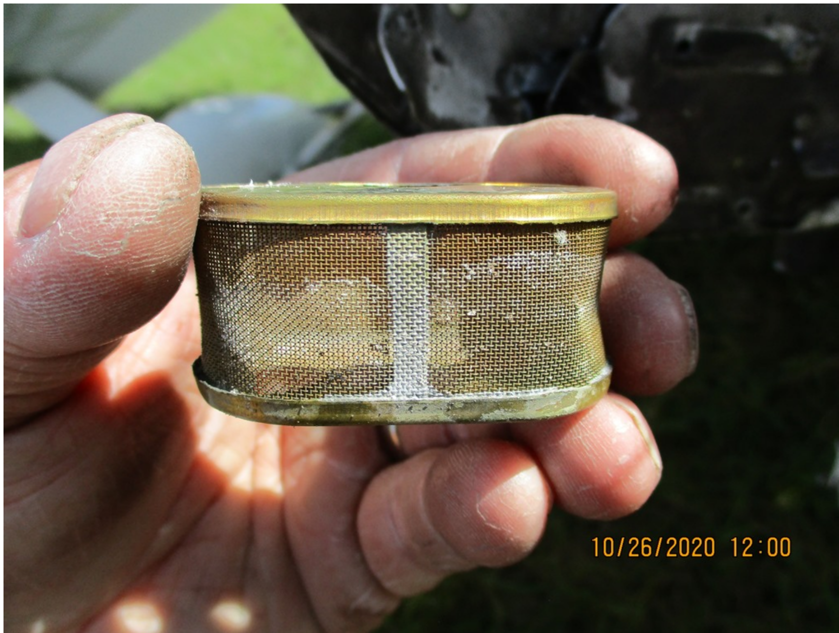
Photo 7 – Airframe Fuel Filter Screen (NTSB)
