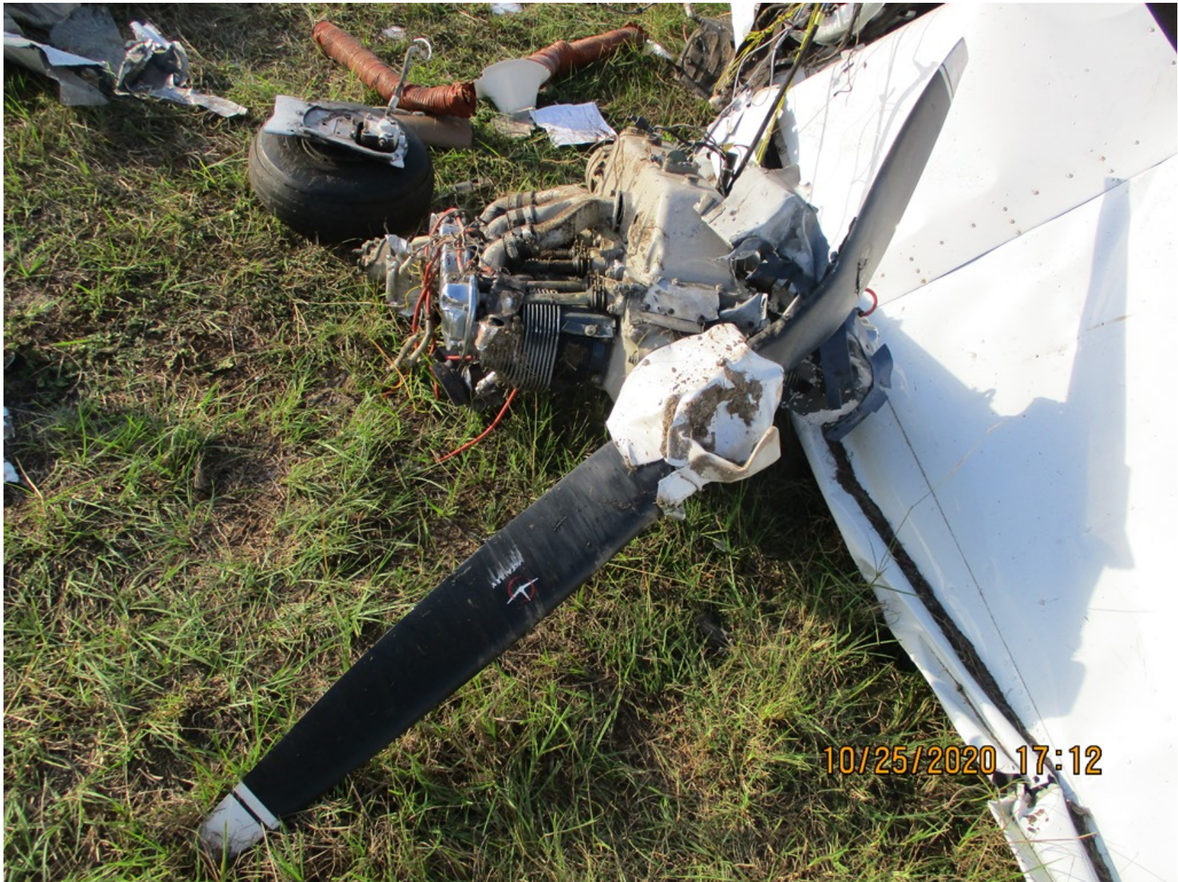
Photo 4 – Engine and Propeller at Accident Site (NTSB)
