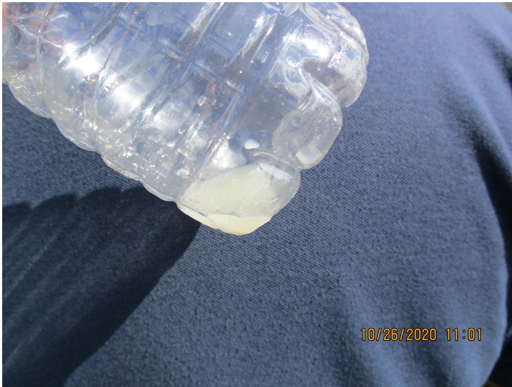
Photo 5 – Cloudy Water Found in Airframe Fuel Filter (NTSB)
