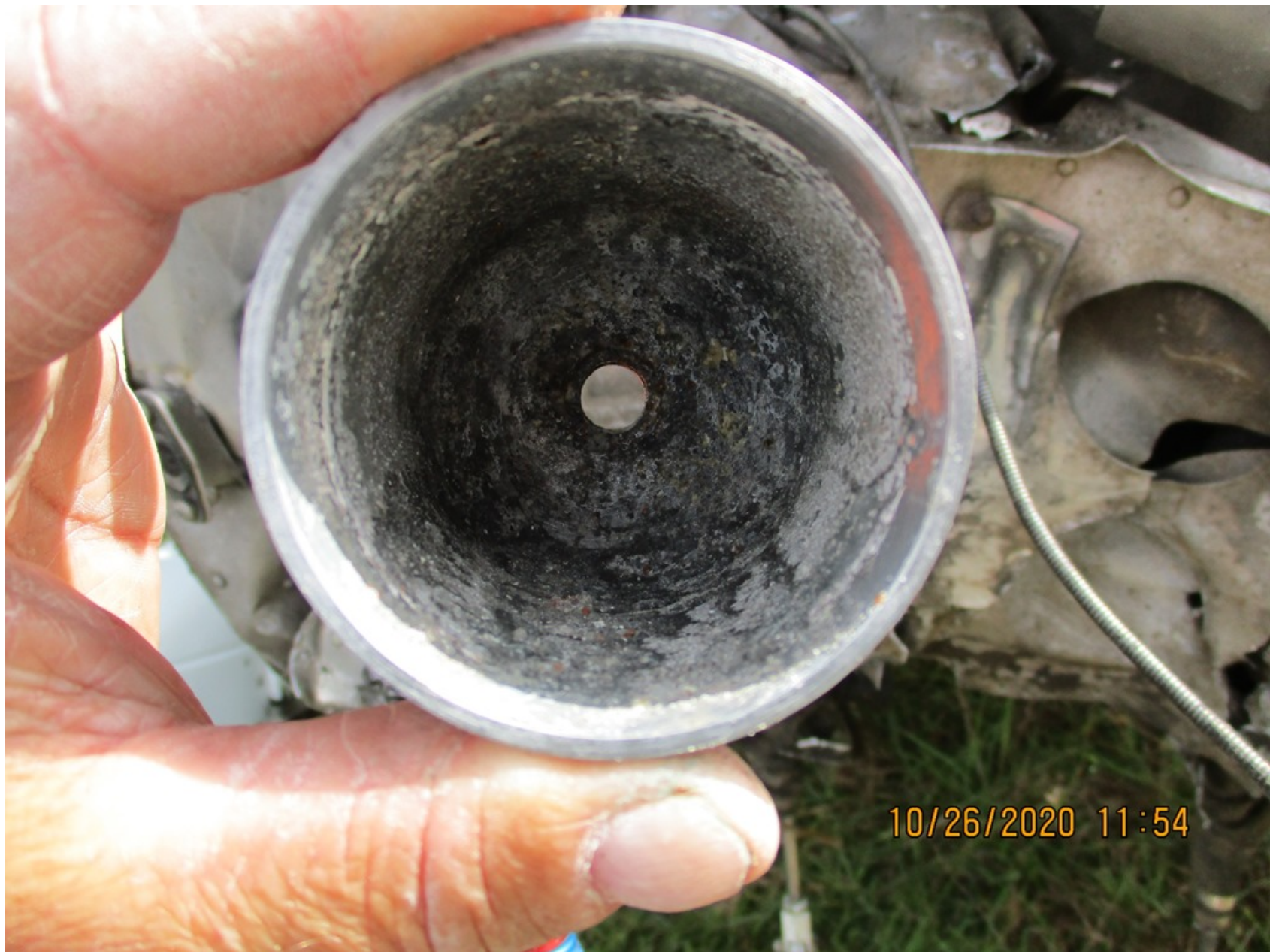
Photo 6 – Airframe Fuel Filter Bowl (NTSB)
