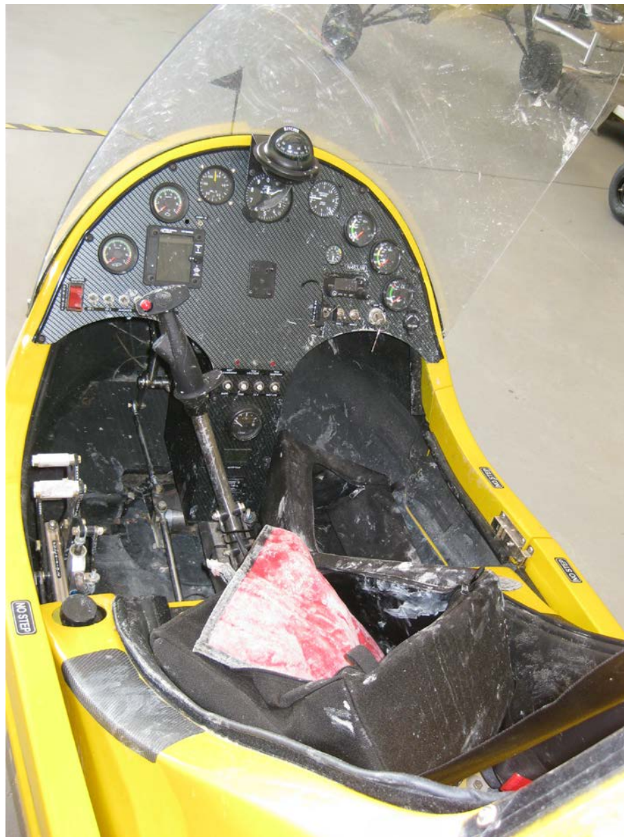
Photo 4 – Photograph of interior of cockpit and fuselage buckling. (Courtesy of FAA)
