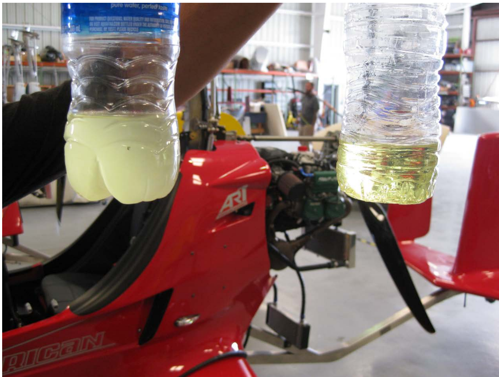
Photo 6 – View of contaminated fuel drained from gyrocopter on left compared to clean fuel on right. (Courtesy of FAA)
