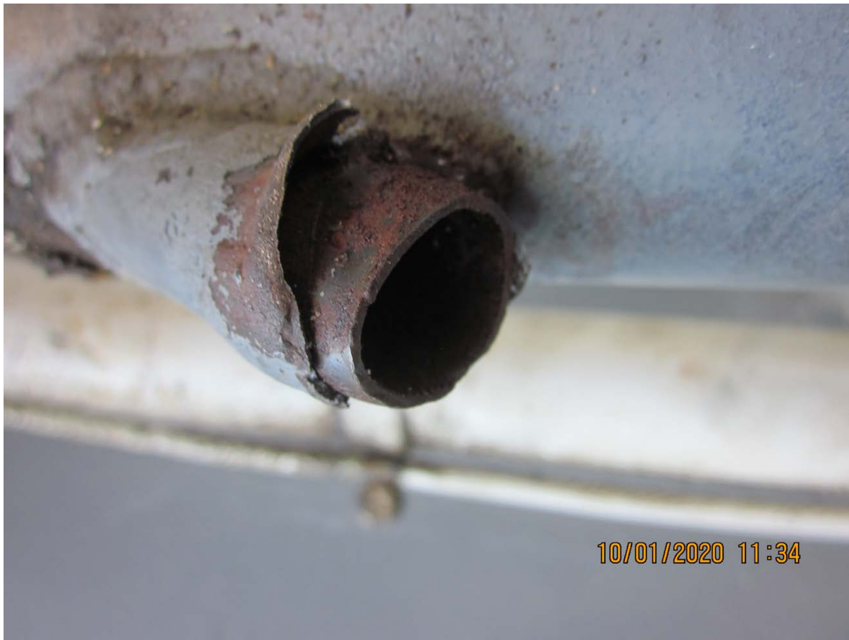
Photo 4 – Closer view of the corrosion visible on the left landing gear airframe cross tube (Photo Courtesy of FAA)
