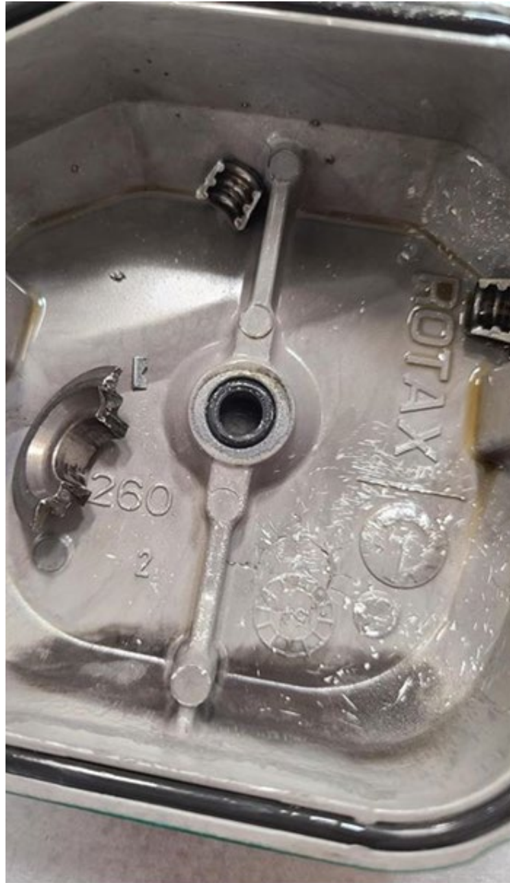
Photo 19 - N639BA Cylinder No. 1 Broken Exhaust Valve Spring Retainer – Courtesy of Icon Aircraft
