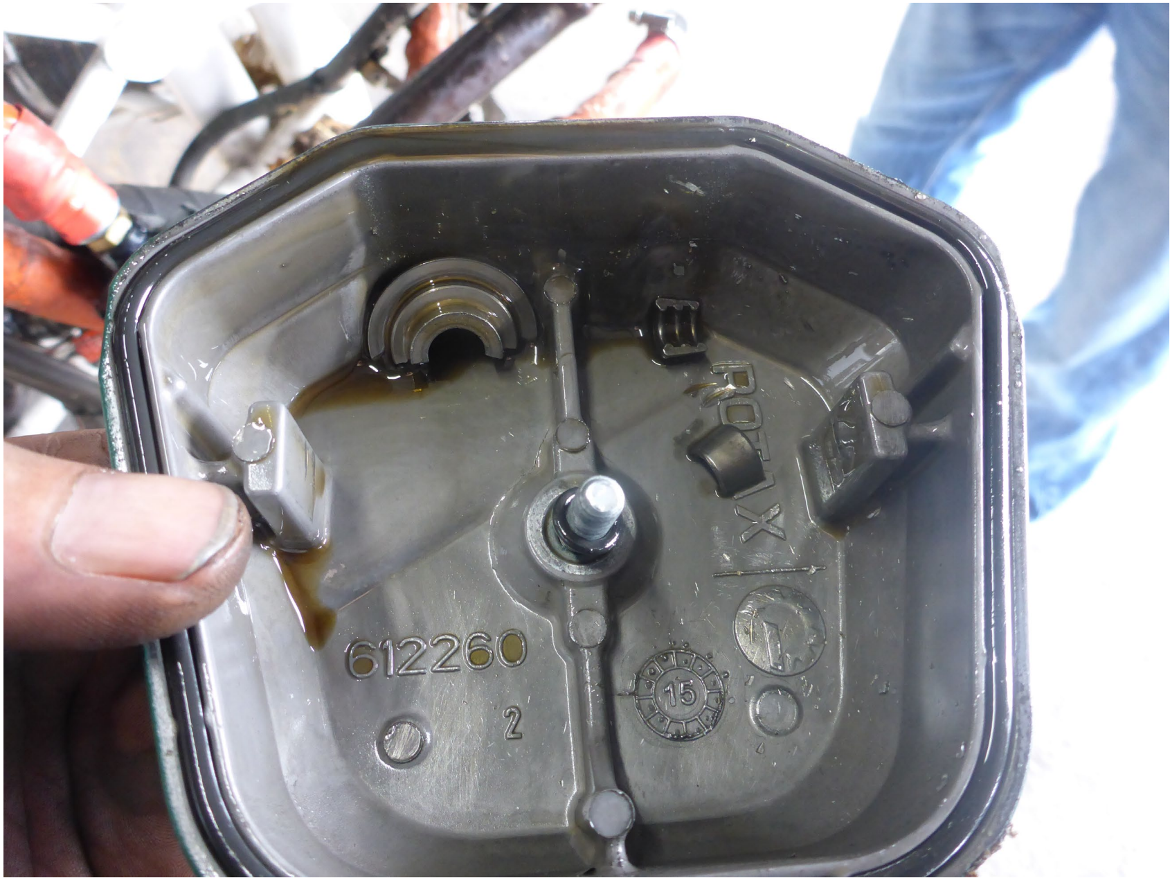
Photo 11 – N562TU Cylinder No. 1 Broken Exhaust Valve Spring Retainer – Courtesy of Rotech Flight Safety
