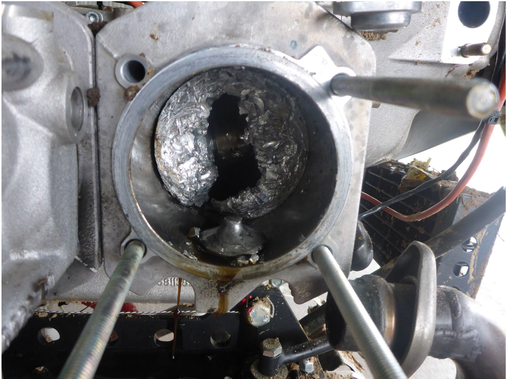
Photo 12 – N562TU No.1 Piston and Exhaust Valve – Courtesy of Rotech Flight Safety
