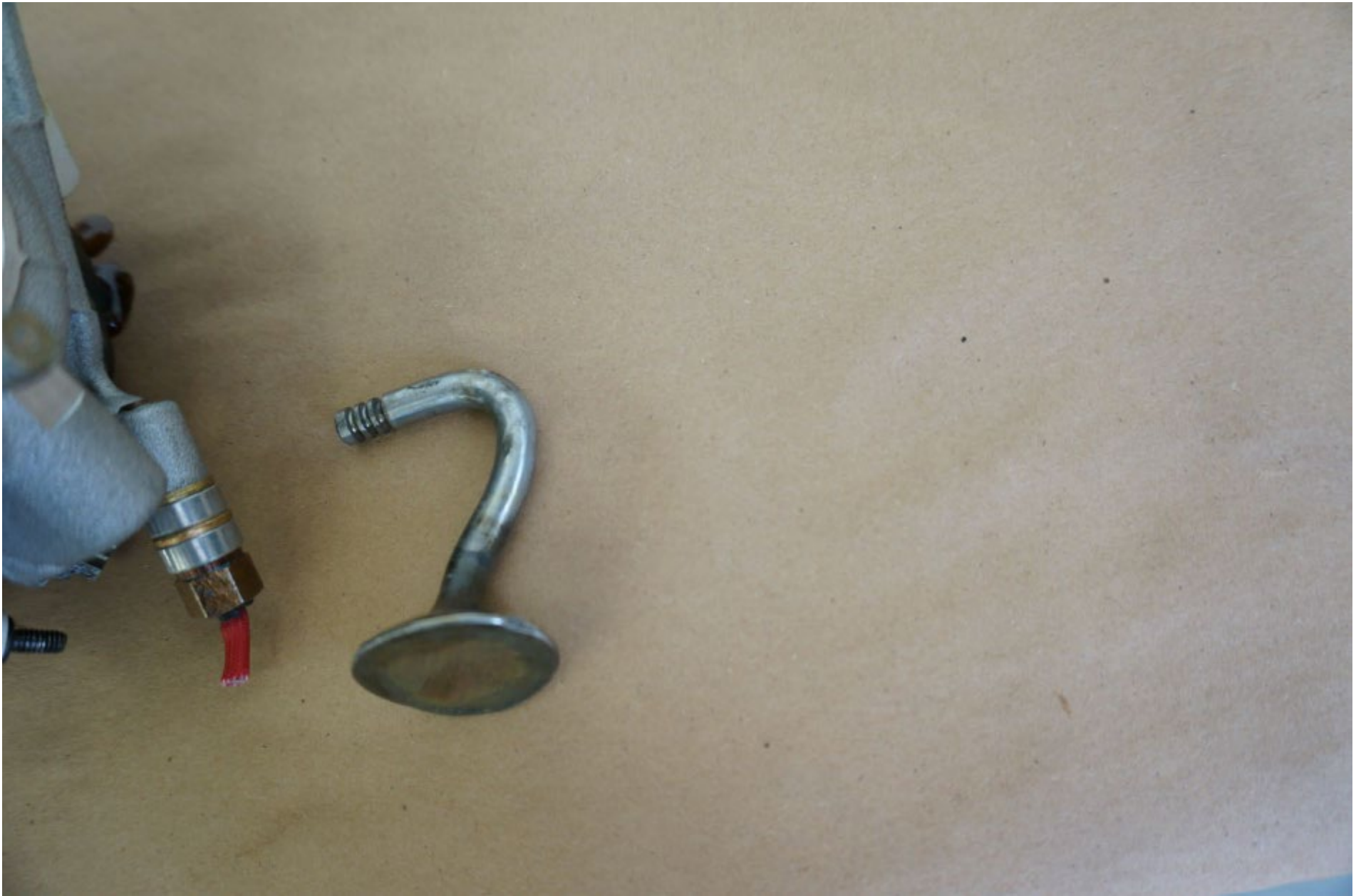
Photo 16 – N561TU No. 1 Exhaust Valve
