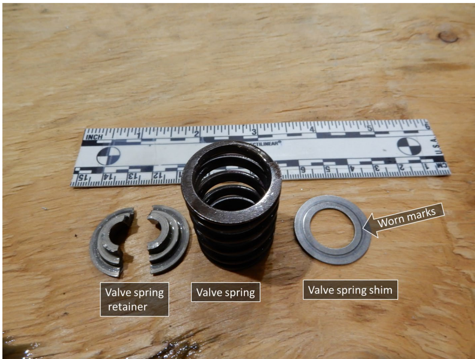
Photo 14 – N204BF – No. 2 Cylinder Intake Valve Spring Retainer, Valve Spring, and Valve Spring Shim
