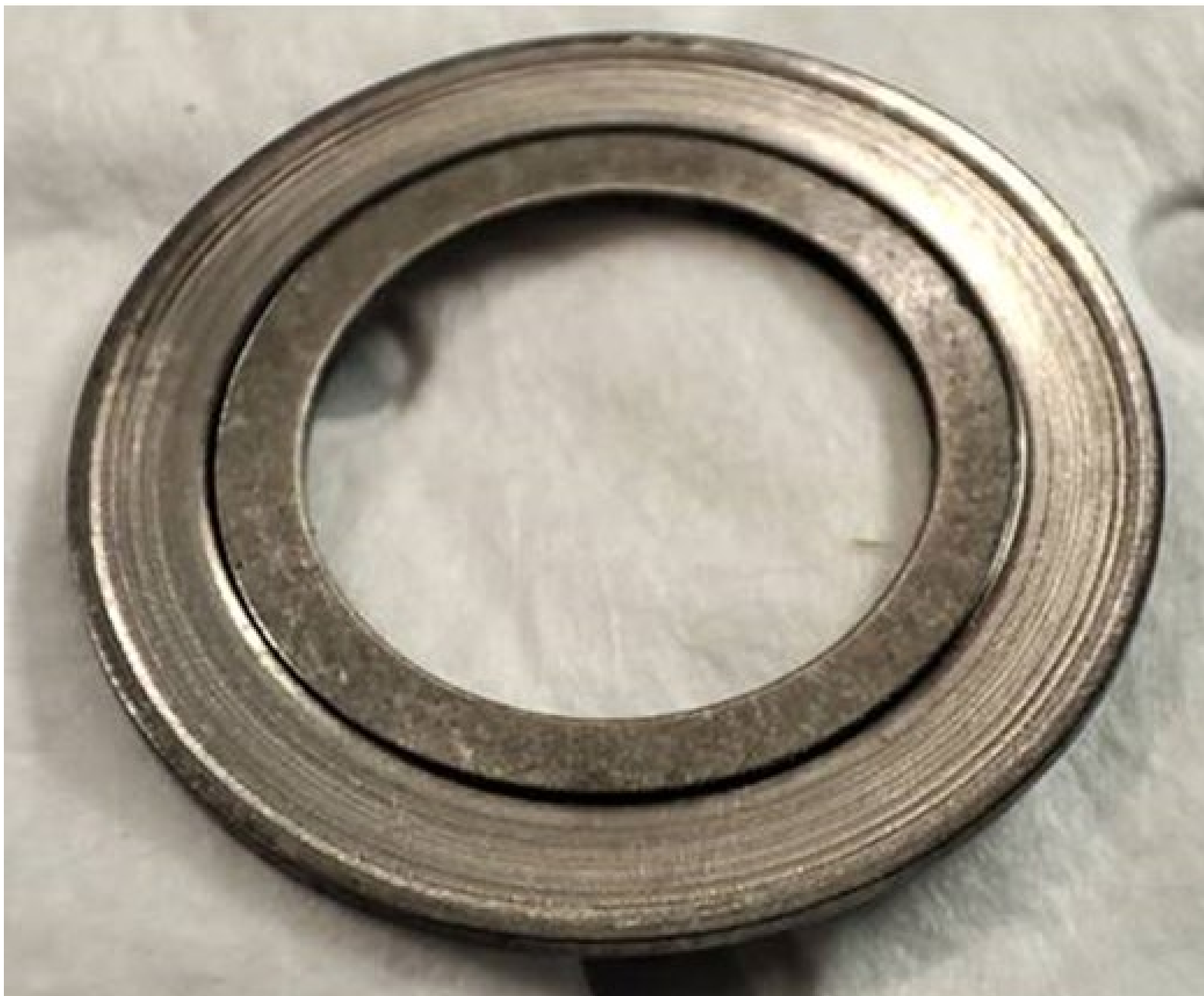
Photo 13 - N562TU No.1 Cylinder Exhaust Valve Spring Shim Wear Marks – Courtesy of BMK
