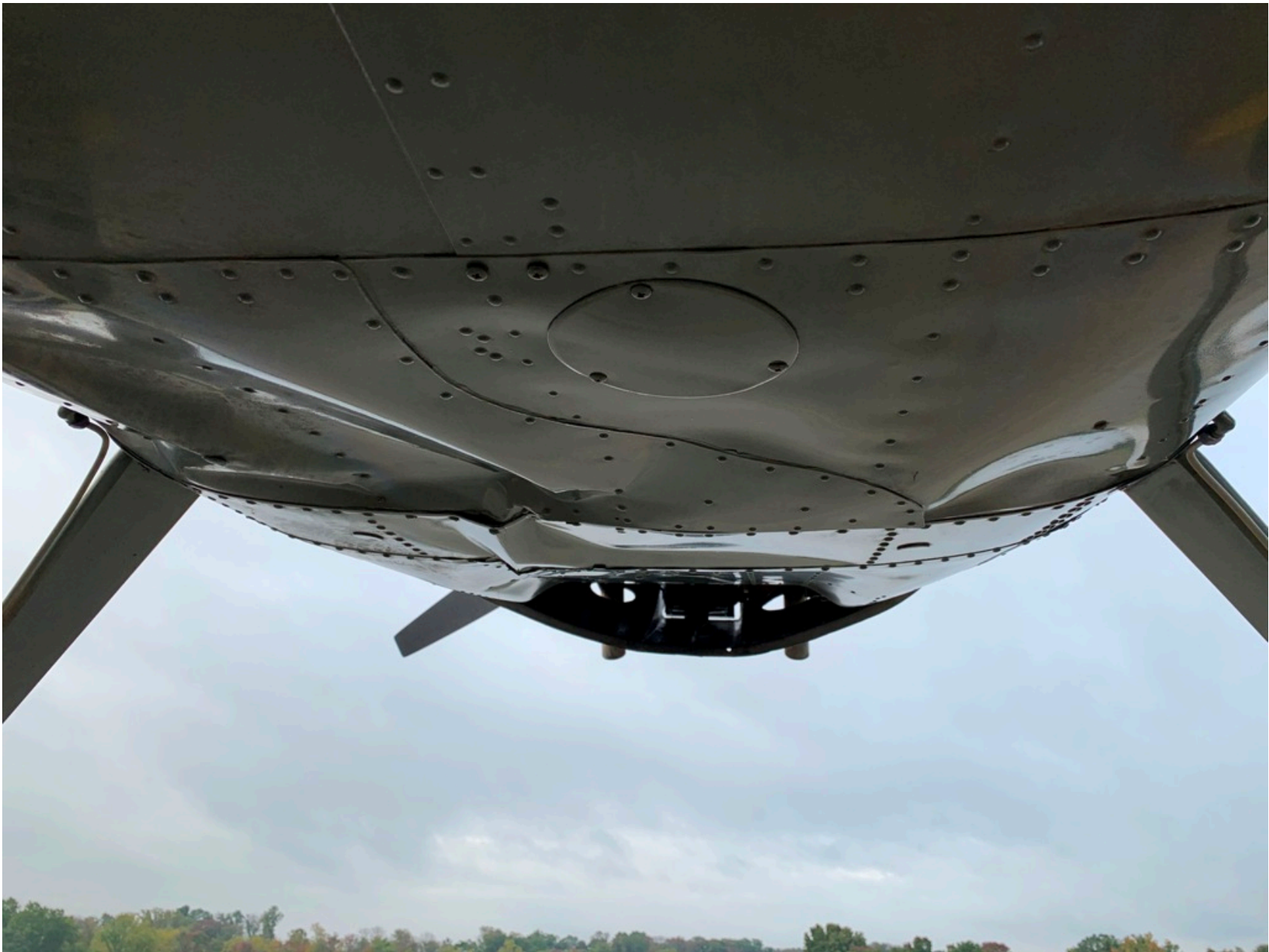
Photo 2 - Digital Photograph Provided by FAA. View of Bottom of Fuselage Taken Behind Main Landing Gear Looking Forward. Note the Structural Damage.
