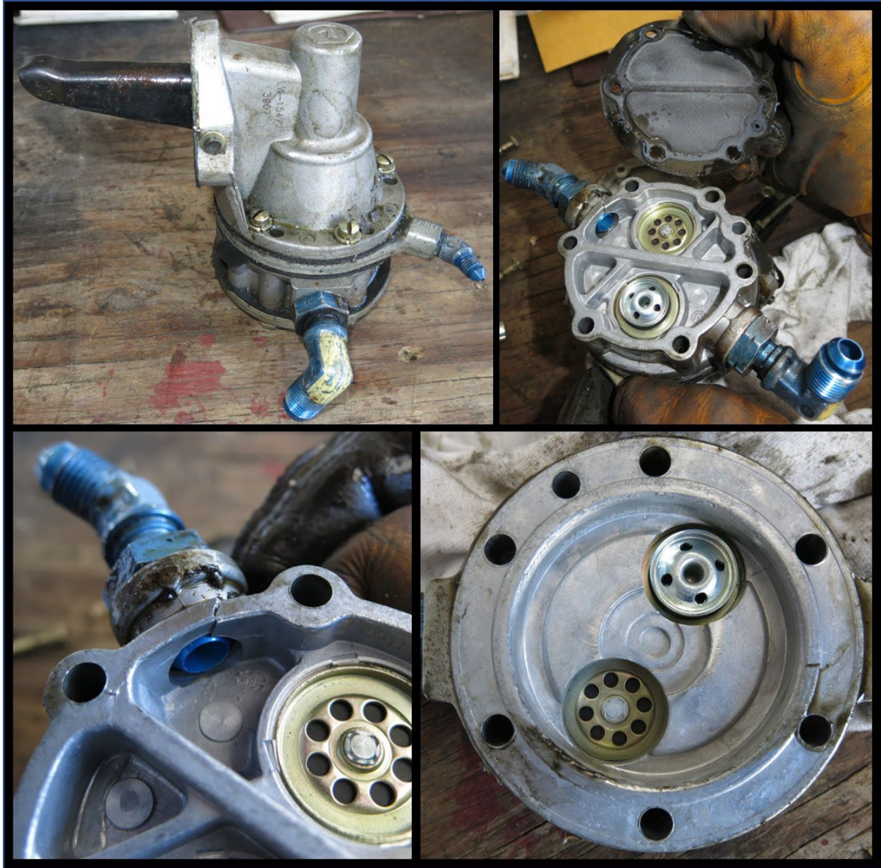
Photograph 5 –Engine driven fuel pump
