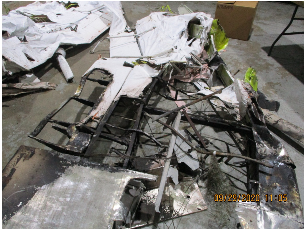
Photo 5: Additional view of fire damaged and impact damaged wing
