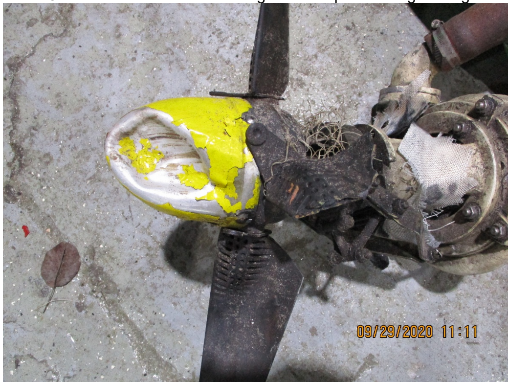
Photo 6: View of impact damaged agriculture fan spraying equipment
