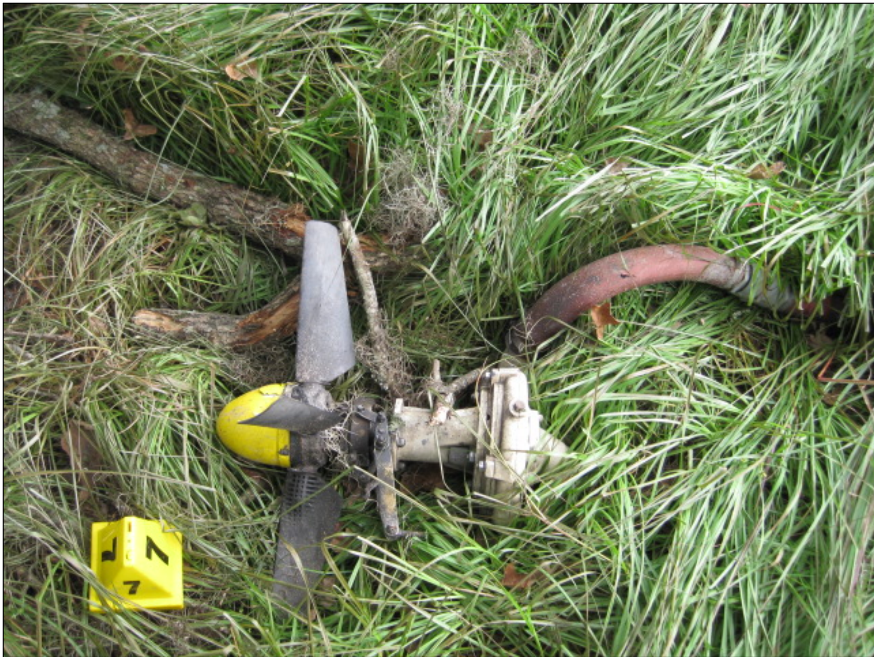
Photo 7 – Separated agriculture spraying fan and piping found near dead tree (Photo Courtesy FAA)
