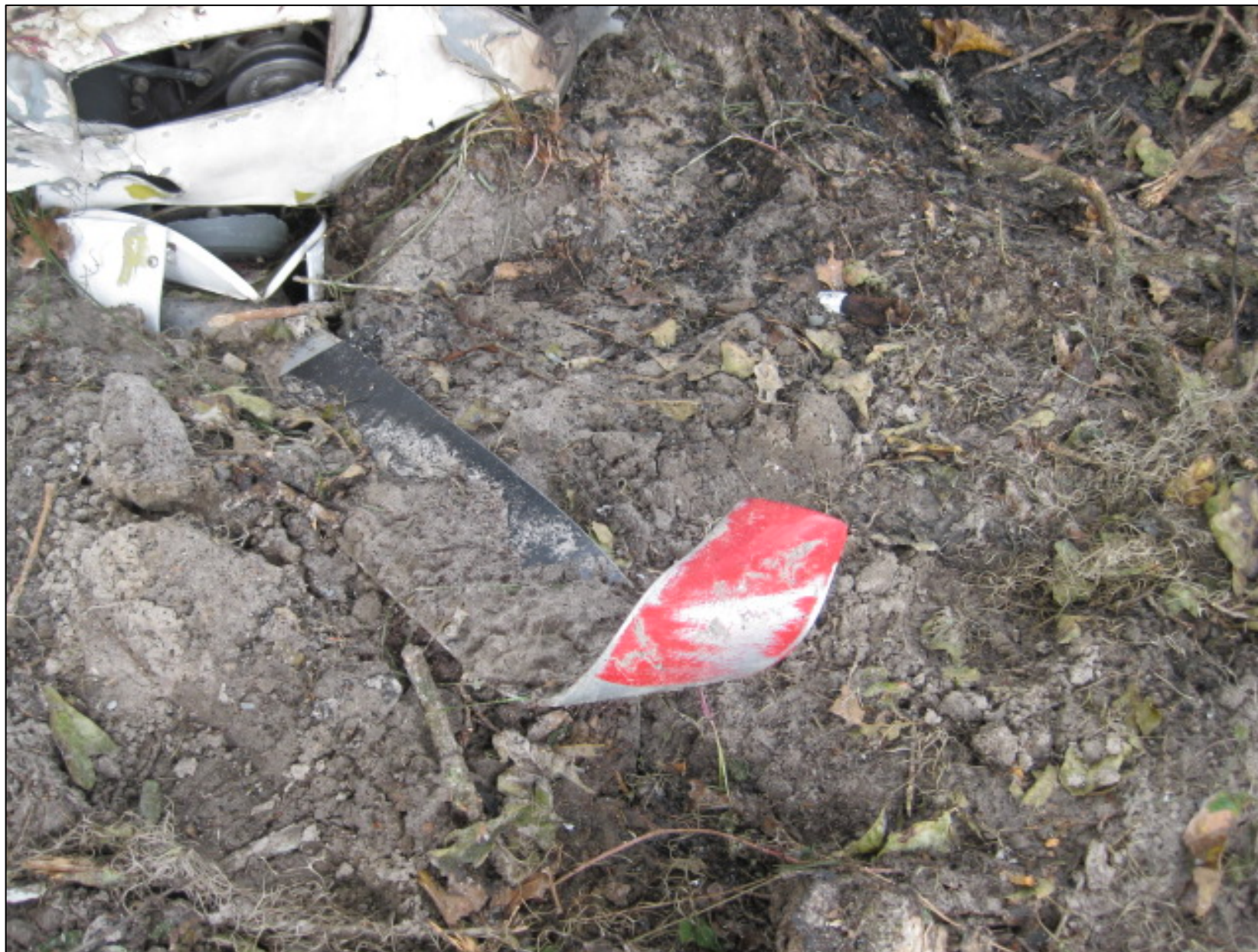
Photo 3 – Curled tip of propeller blade (Photo Courtesy of FAA)
