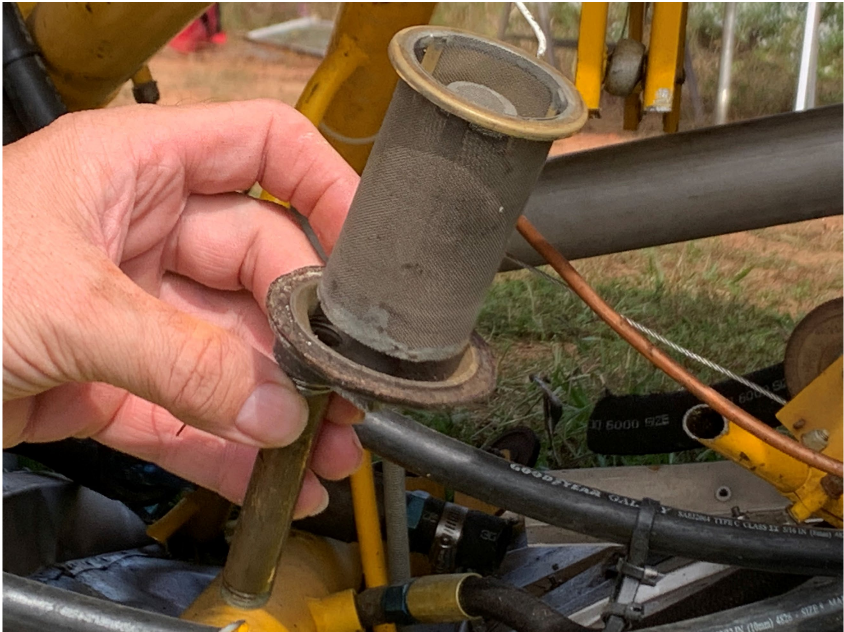
Photo 9 – Fuel Strainer – Courtesy of FAA
