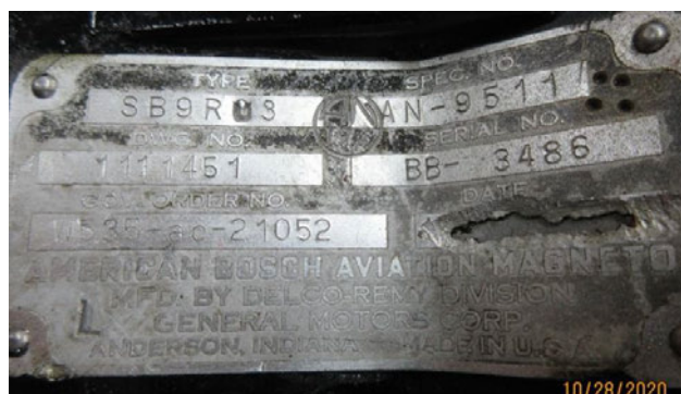
Photo # 4 Data Plate of S/N: BB-3486 SB9RU-3 Covington Aircraft Overhaul
