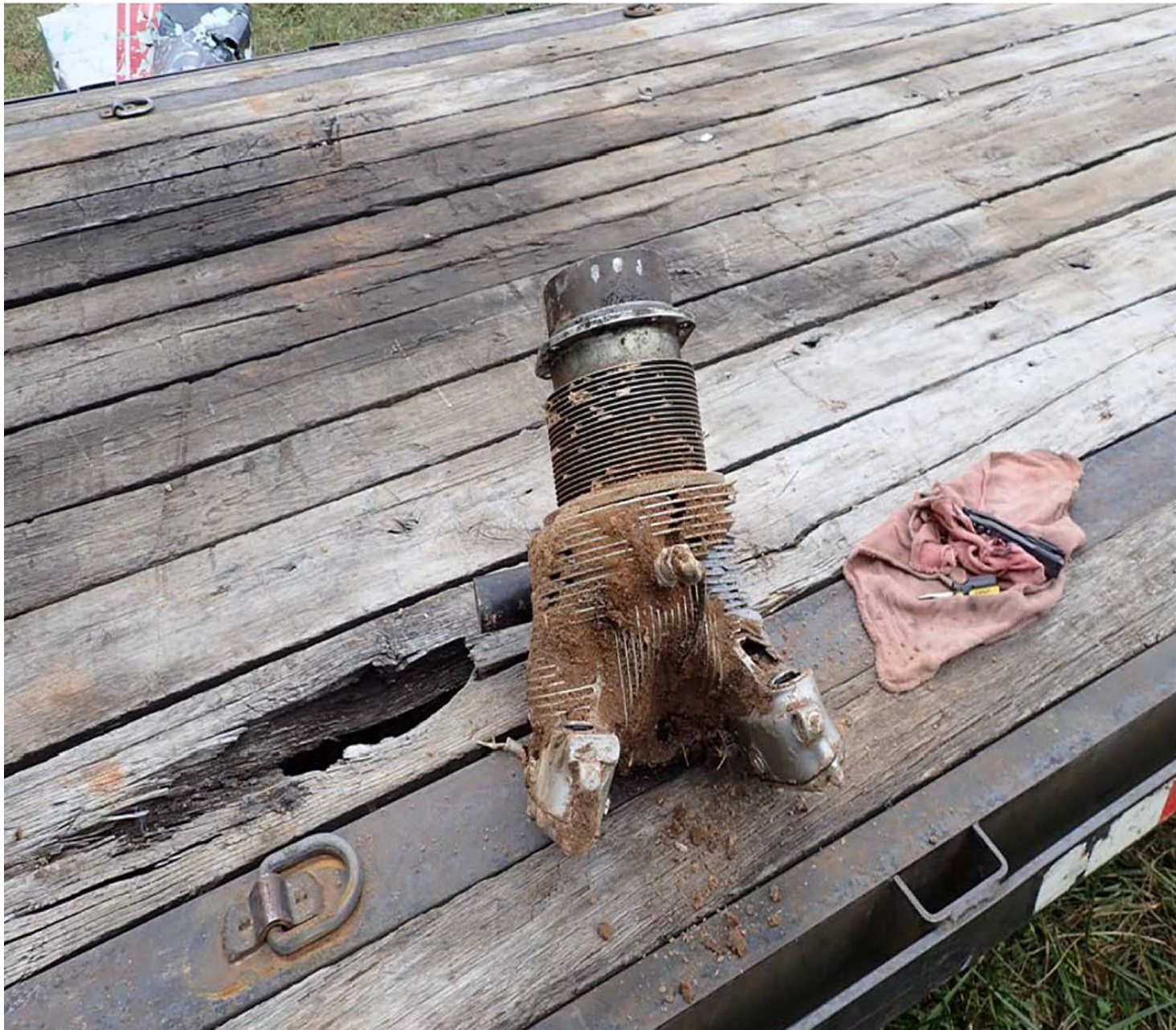
Photo 4 – View of Separated Cylinder after Recovery (FAA)
