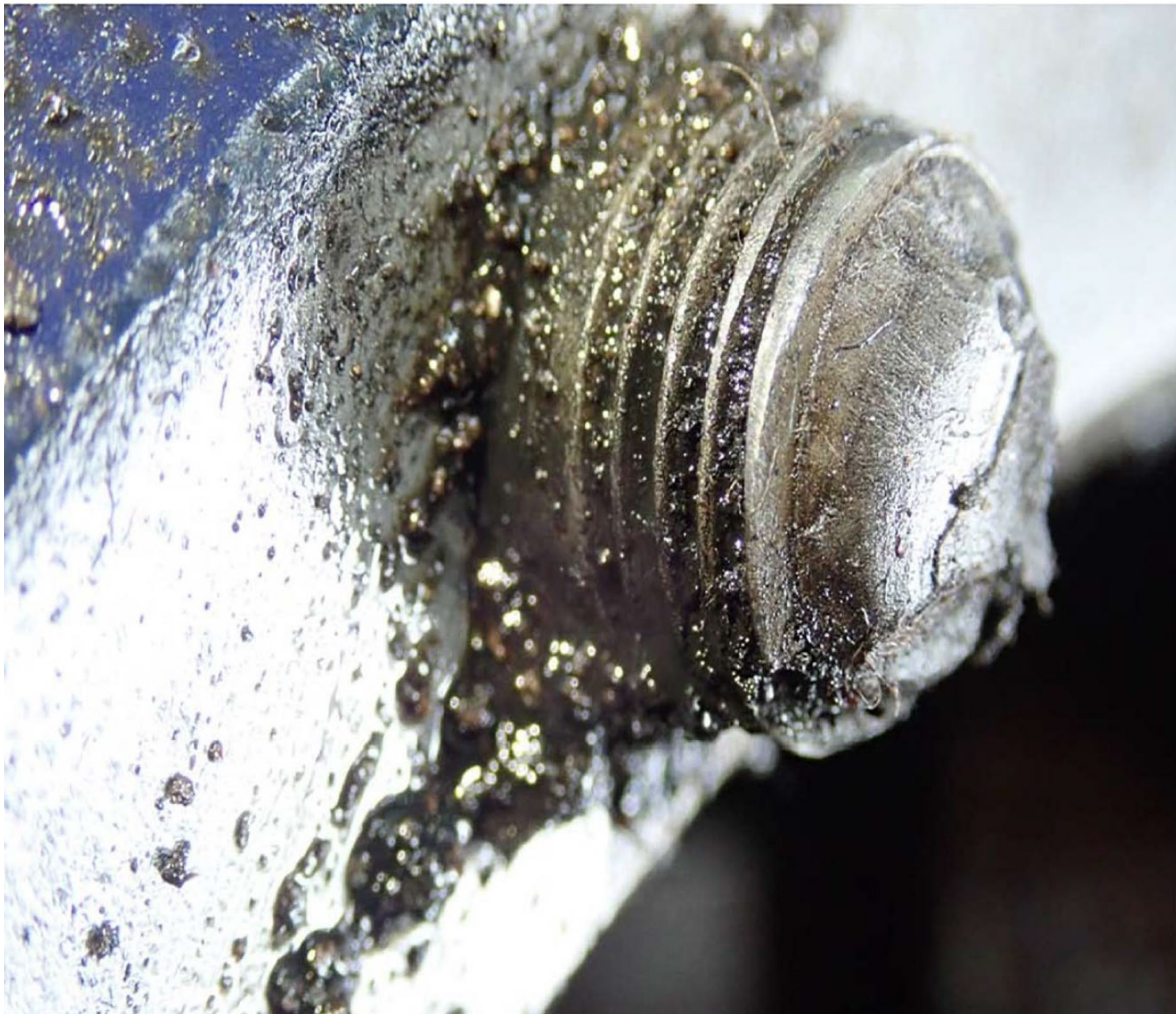
Photo 5 – View of Fractured Cylinder Mount Stud (FAA)
