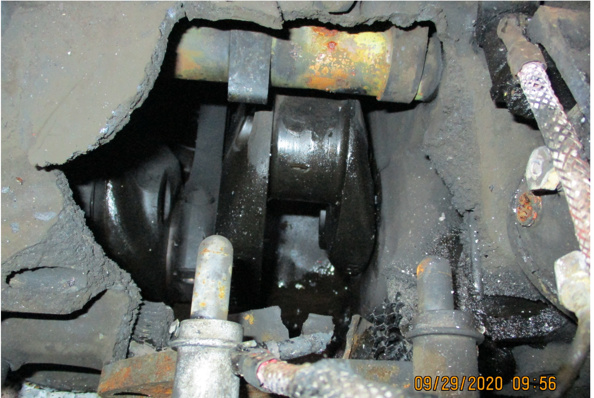
Photo 5 – Hole at #2 cylinder case.
