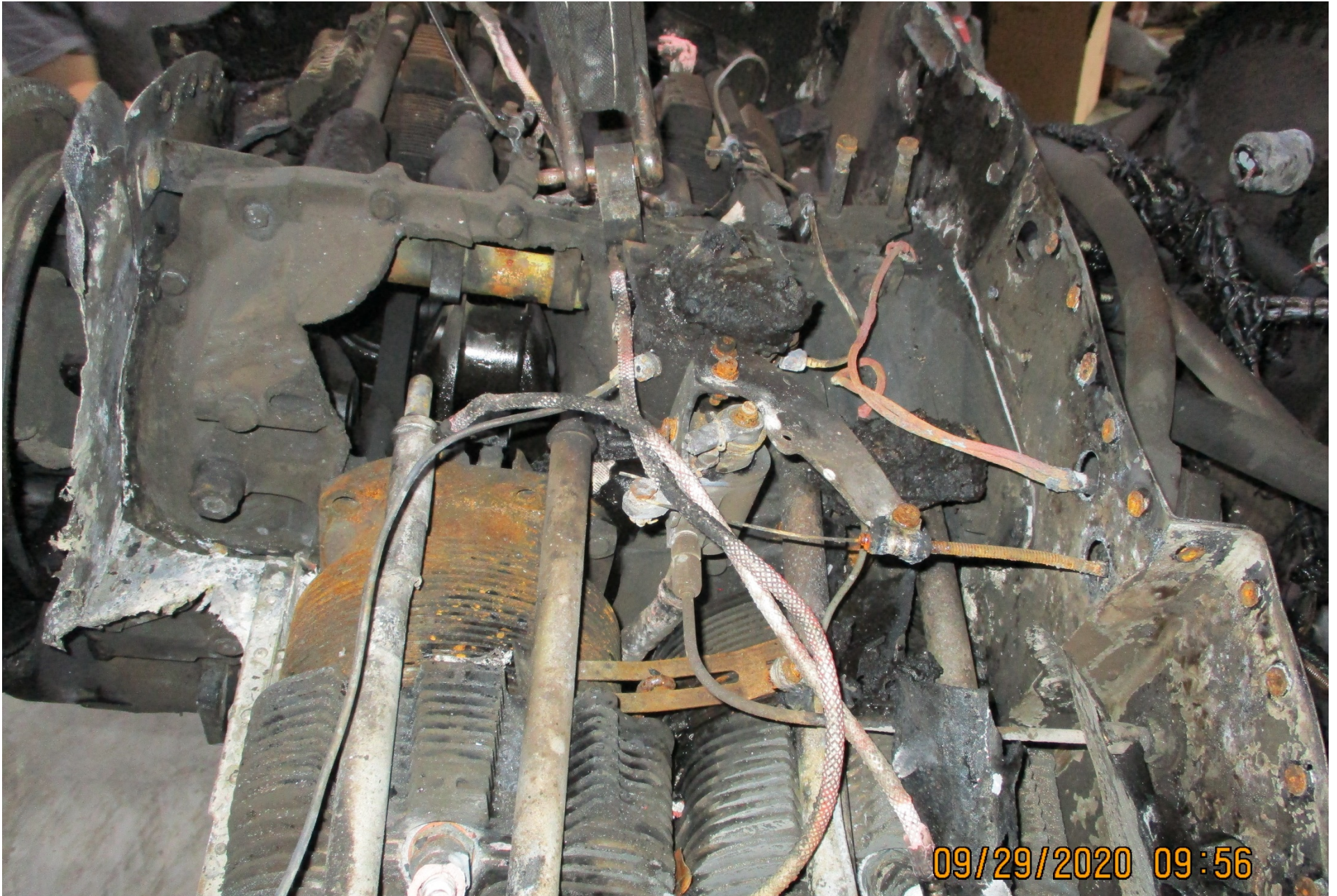
Photo 4 – Engine, hole in case at #2 cylinder
