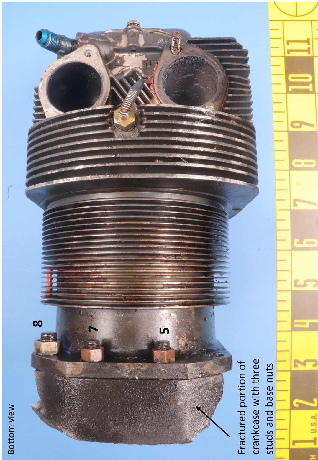
Figure 4 Bottom view of the cylinder shows a fractured portion of the crankcase that remained attached to the cylinder through clamping force provided by the 5:00, 7:00 and 8:00 studs.
