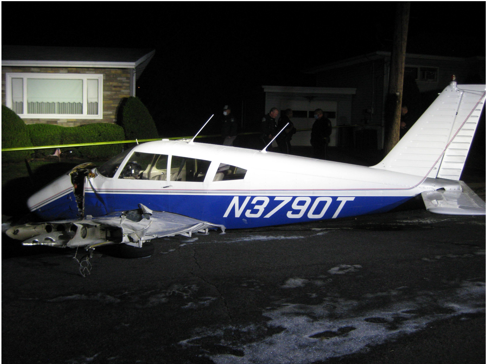
Photo 2 - Digital Photograph Provided by FAA. Left Side View of the Airplane at the Accident Site. Note the Separated Outer Section of the Left Wing.
