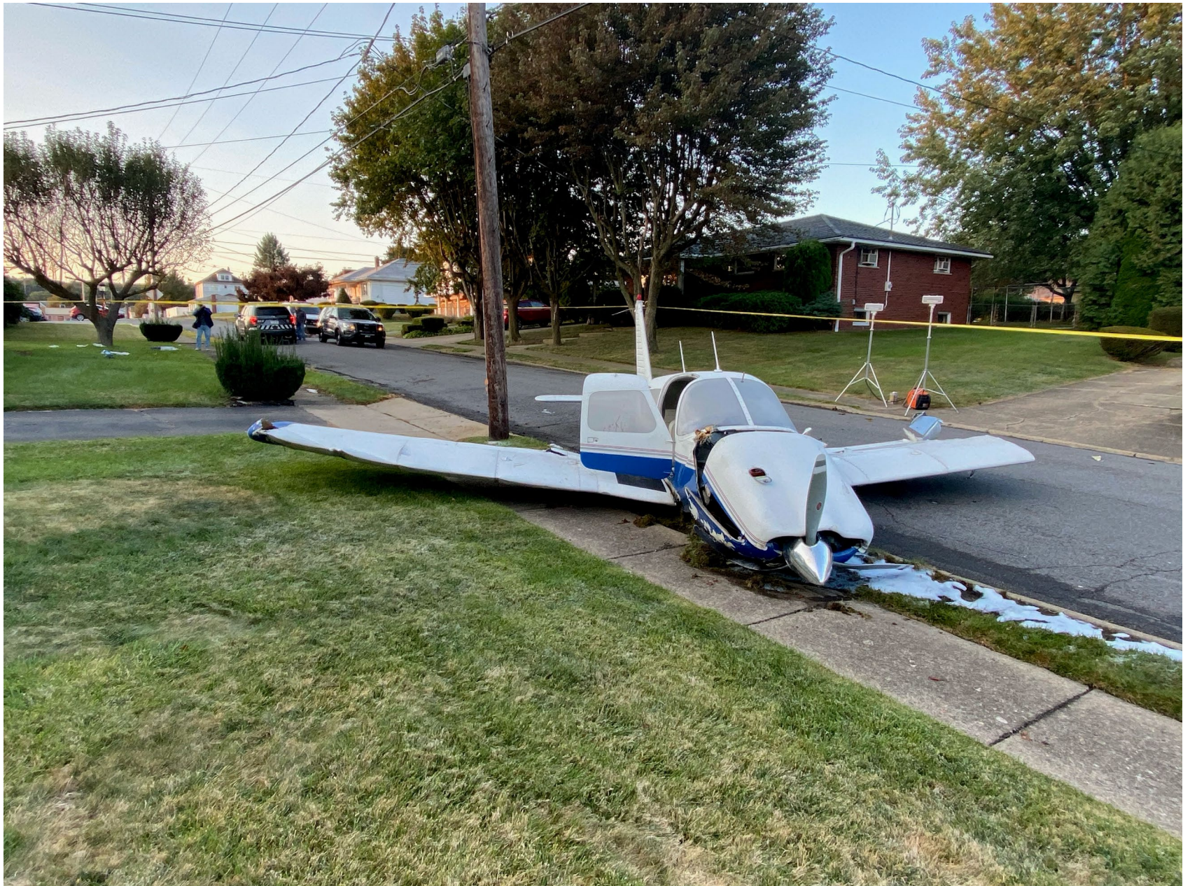
Photo 1 – Digital Photograph Provided by FAA. Right Forward Quartering View of the Airplane at the Accident Site. Note the Separated Outer Section of the Left Wing.
