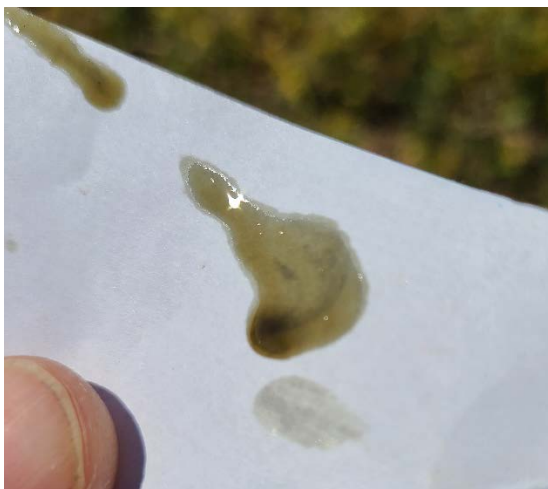
Photo 3: Bits of shiny particles in oil (Photo courtesy of Federal Aviation Administration)
