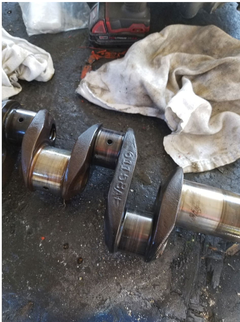
Photo 4 – View of crankshaft showing overheating on journals.
