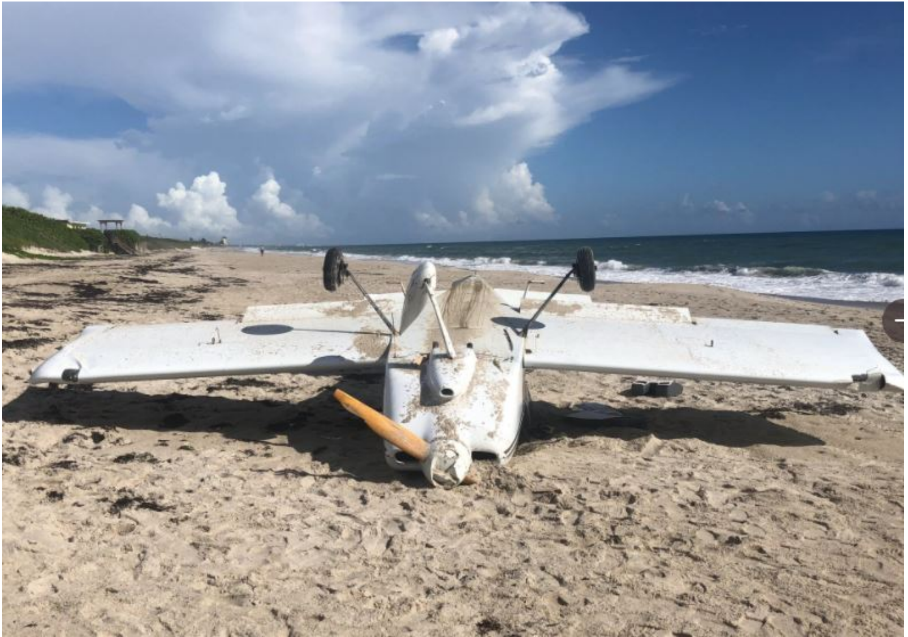
Photo 1 – View of airplane inverted on beach after forced landing (also showing oil streaks on underside)
