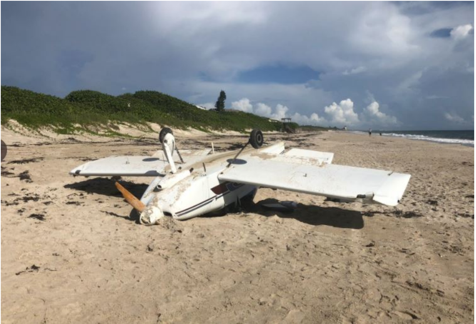
Photo 2 – View of airplane wreckage inverted showing oil streaking
