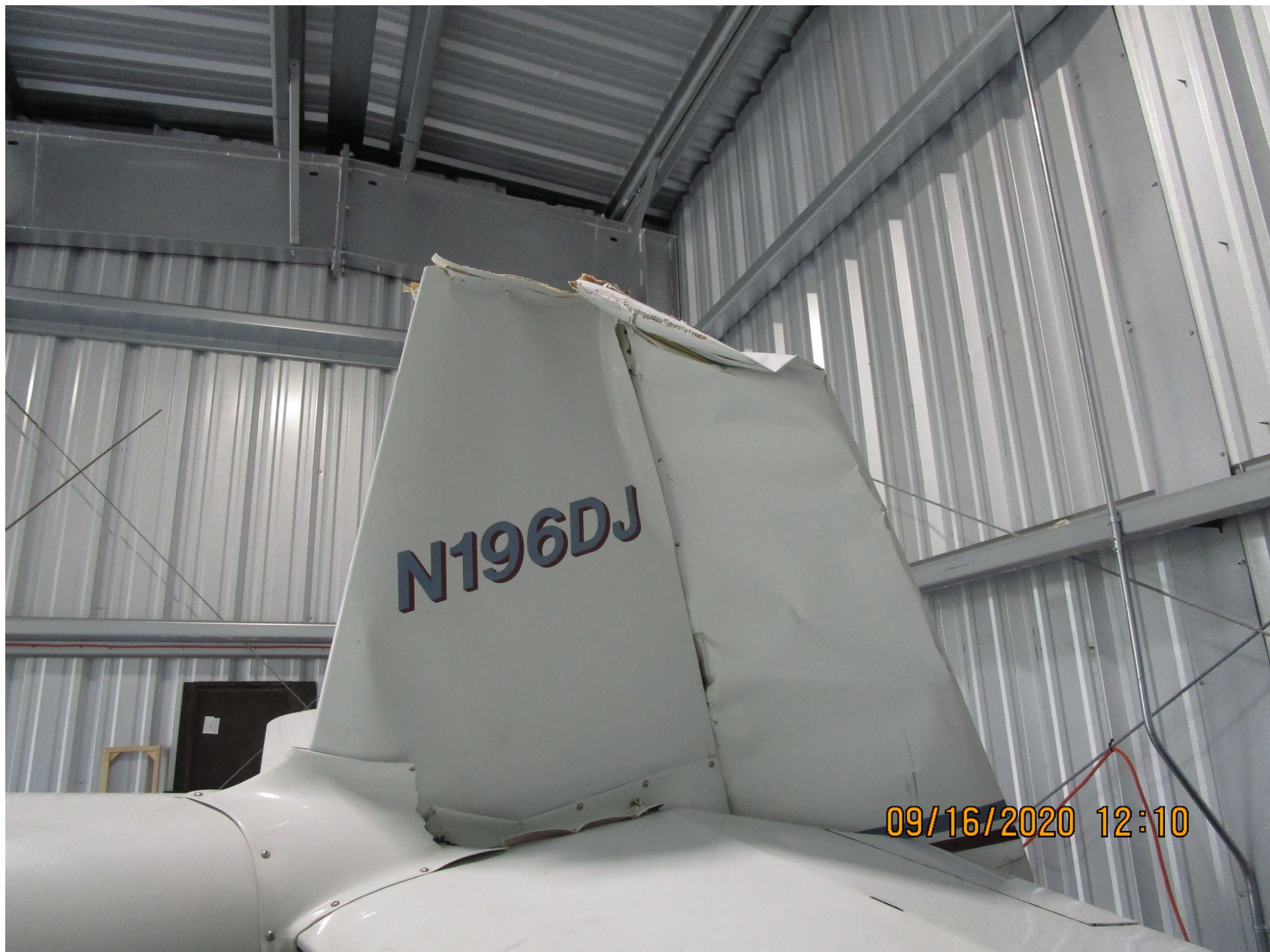
Photo 3 – View of damaged vertical stabilizer and rudder
