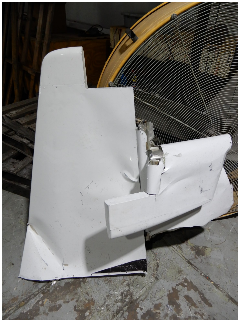
Photo 9 – Vertical Stabilizer and Rudder (NTSB Photo)
