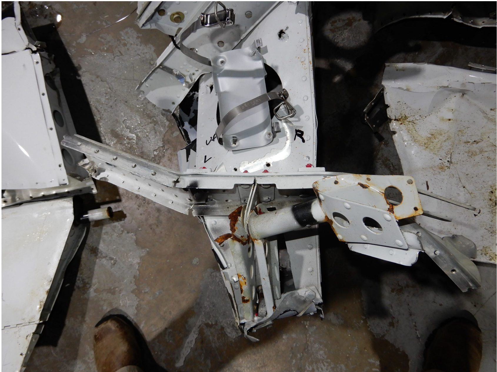
Photo 4 – Empennage Structure (NTSB Photo)
