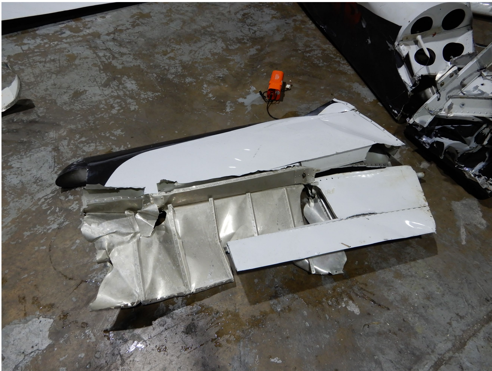
Photo 5 – Left Horizontal Stabilizer and Elevator (NTSB Photo)
