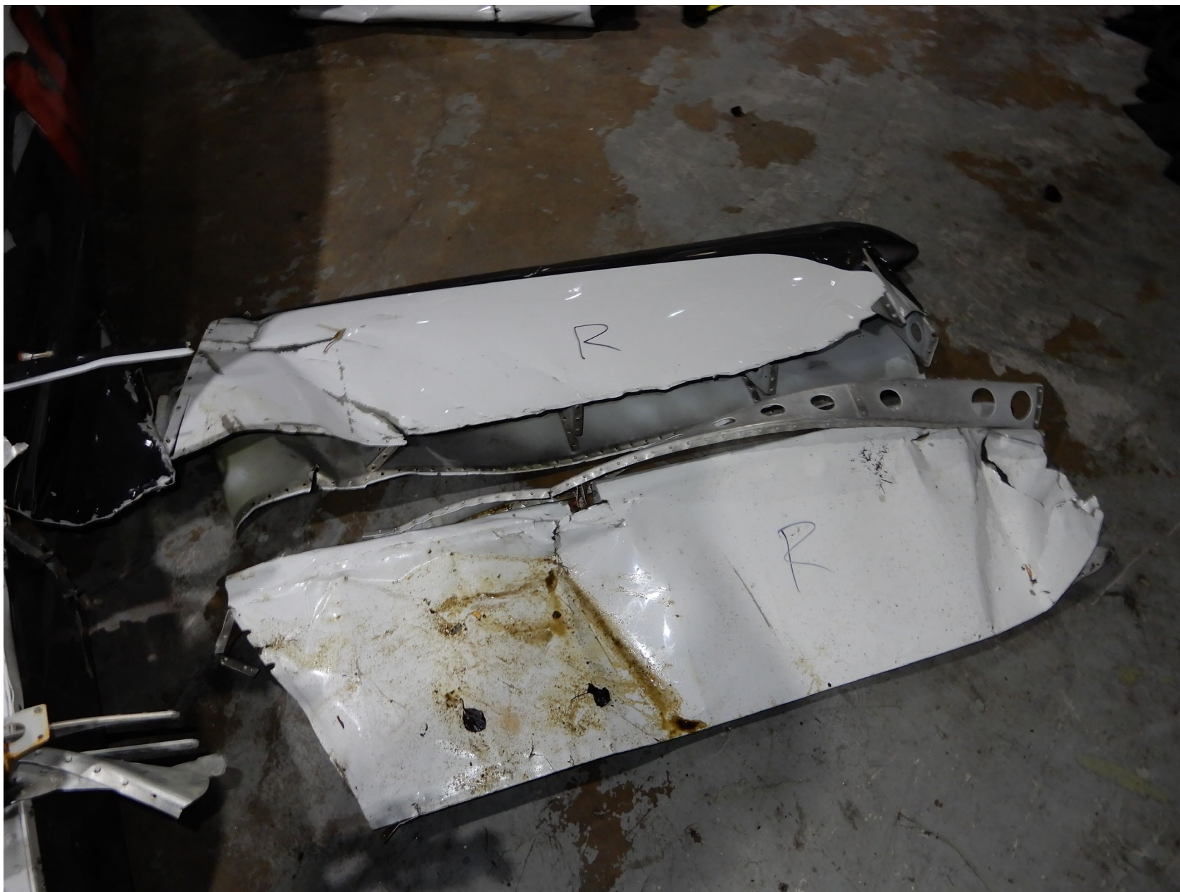
Photo 6 – Right Horizontal Stabilizer and Rudder (NTSB Photo)
