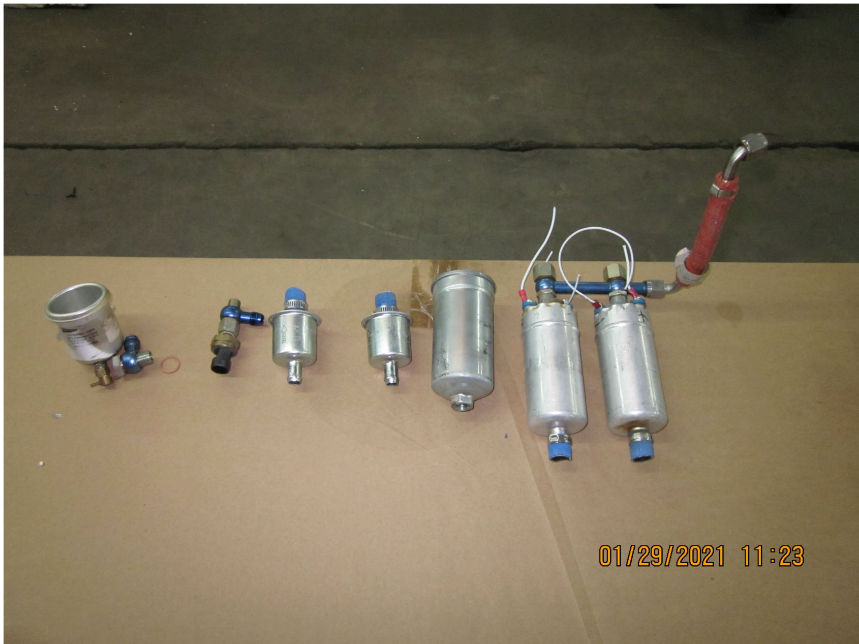
Photo 13 – Fuel Strainers, Filters, and Pumps – Courtesy of UL Power
