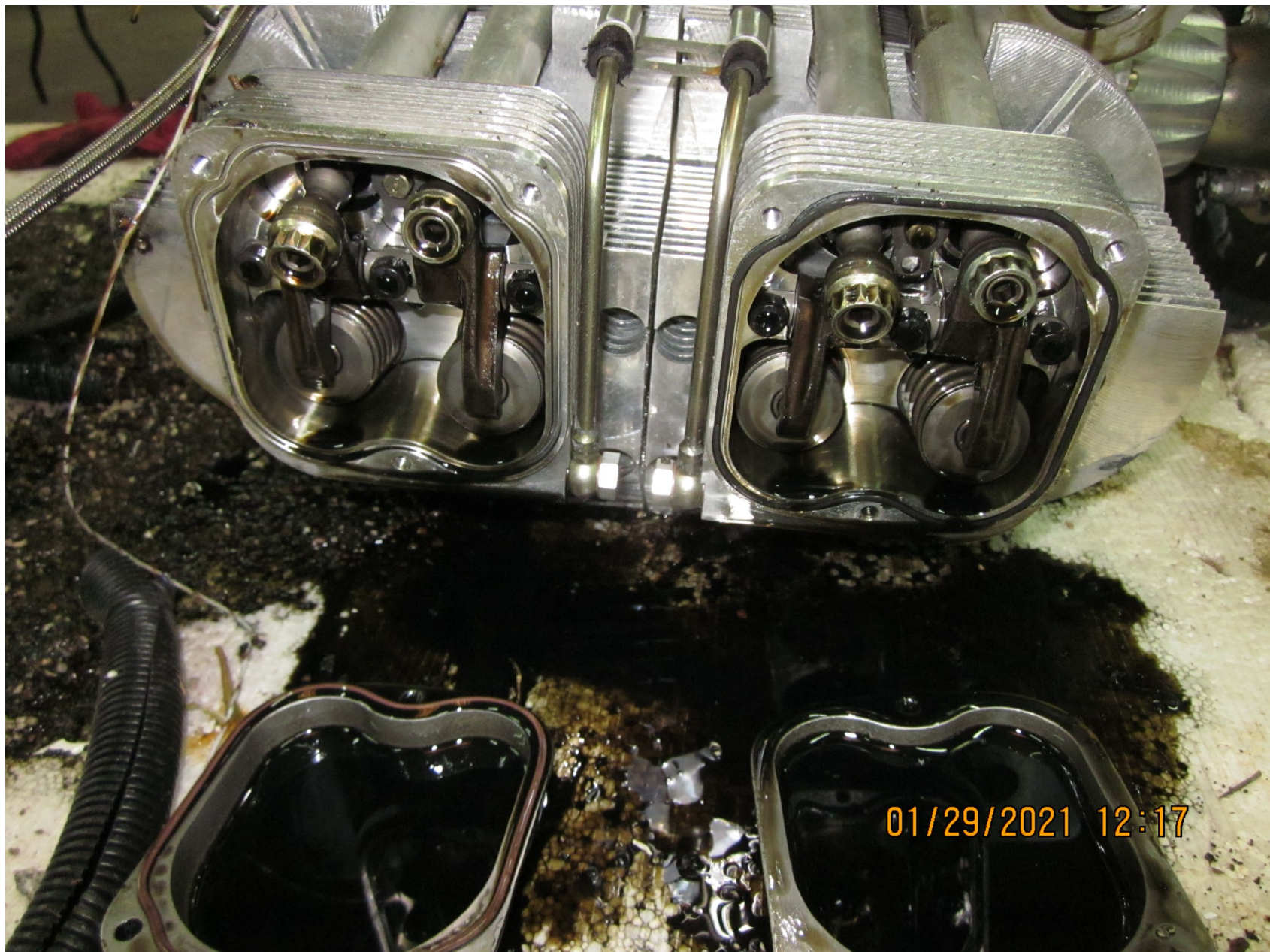
Photo 18 – Interior of Right Side Rocker Boxes – Courtesy of UL Power
