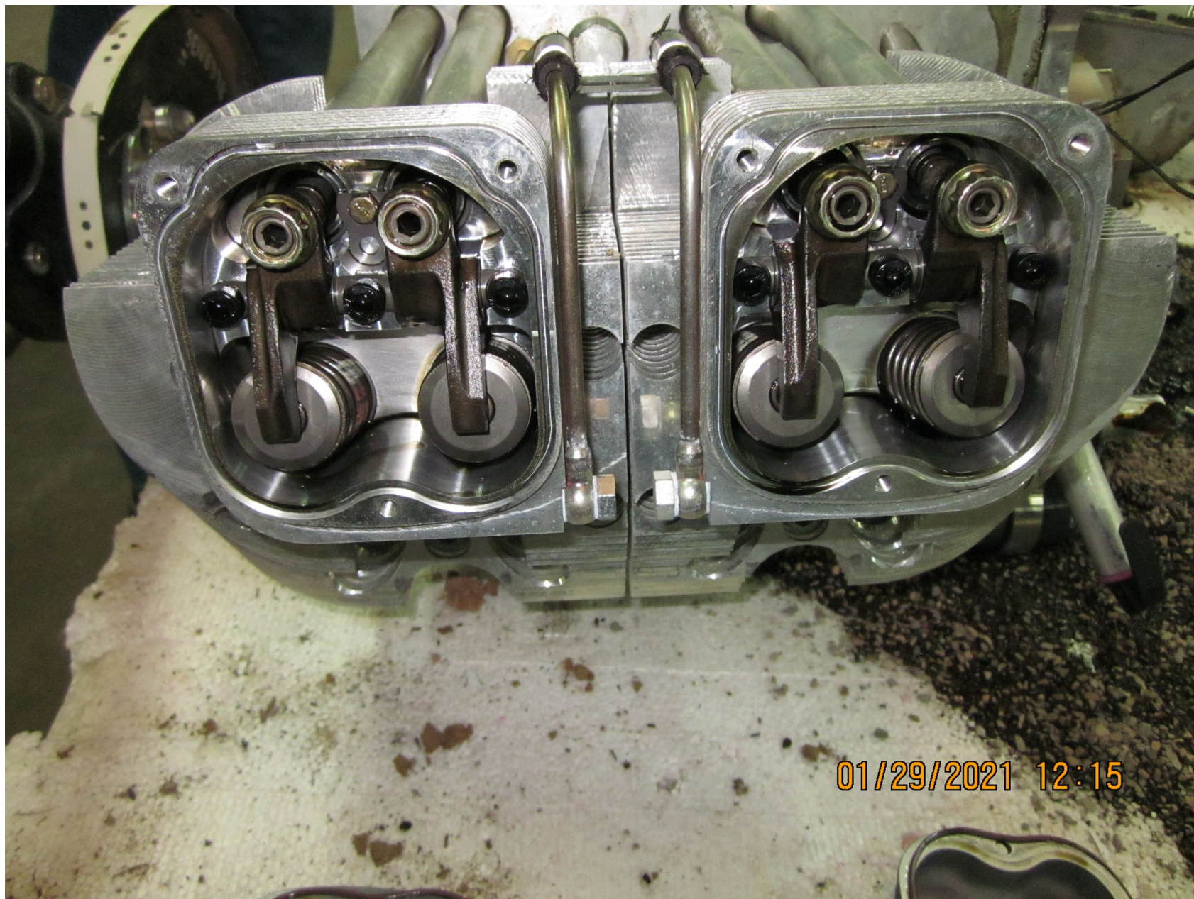
Photo 17 – Interior of Left Side Rocker Boxes – Courtesy of UL Power
