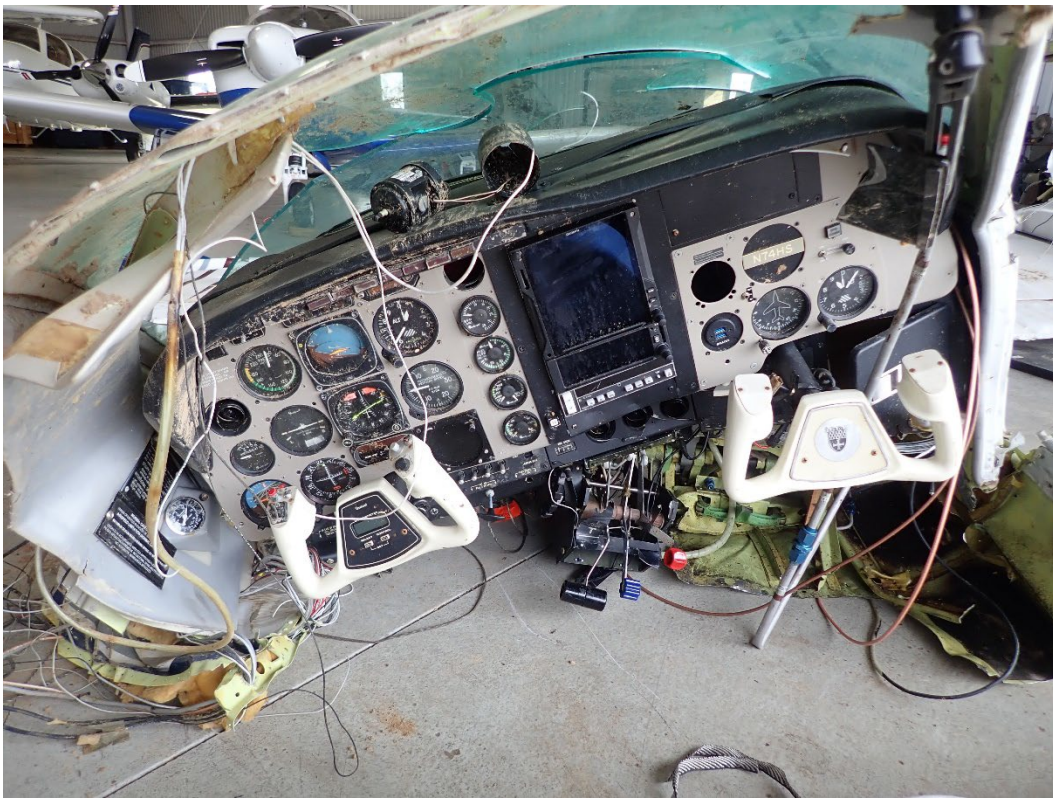
Photograph 11 – Accident airplane – Post-examination of cockpit instrument panel.
