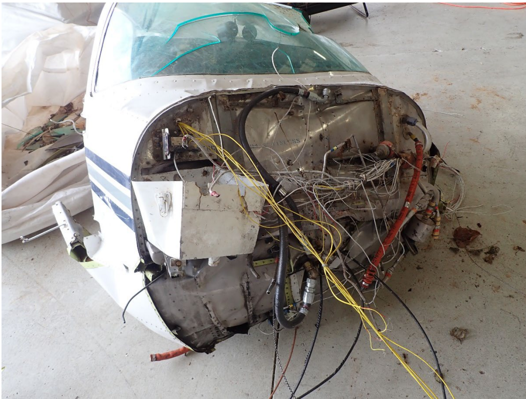
Photograph 5 – Accident airplane – Post-examination of fuselage and firewall.
