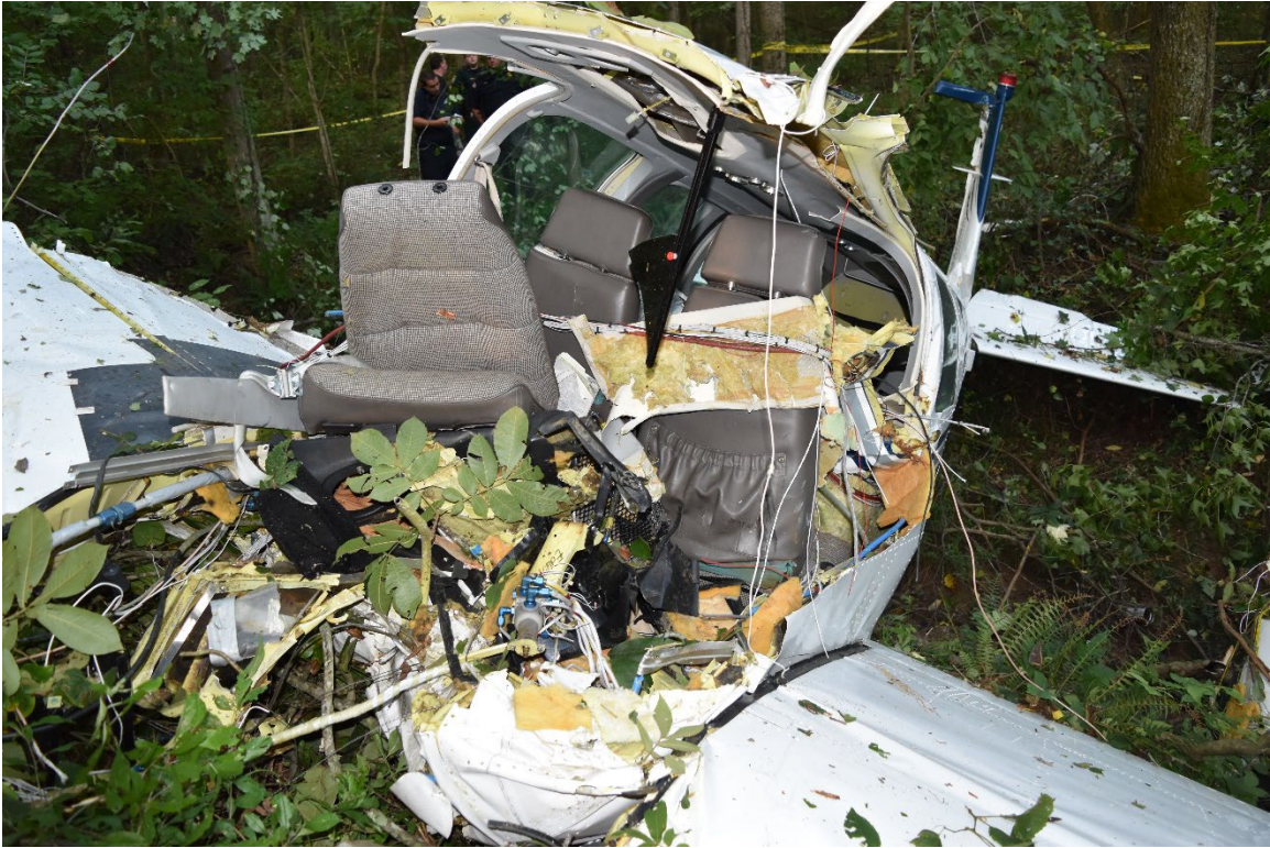
Photograph 2 – Accident Site – Separated aft portion of fuselage.
