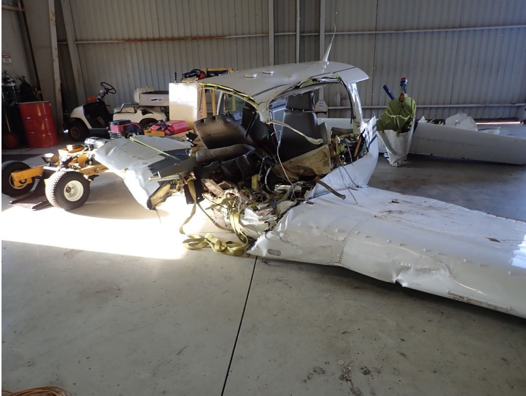
Photograph 4 – Accident airplane – Post-examination of aft fuselage and left wing.
