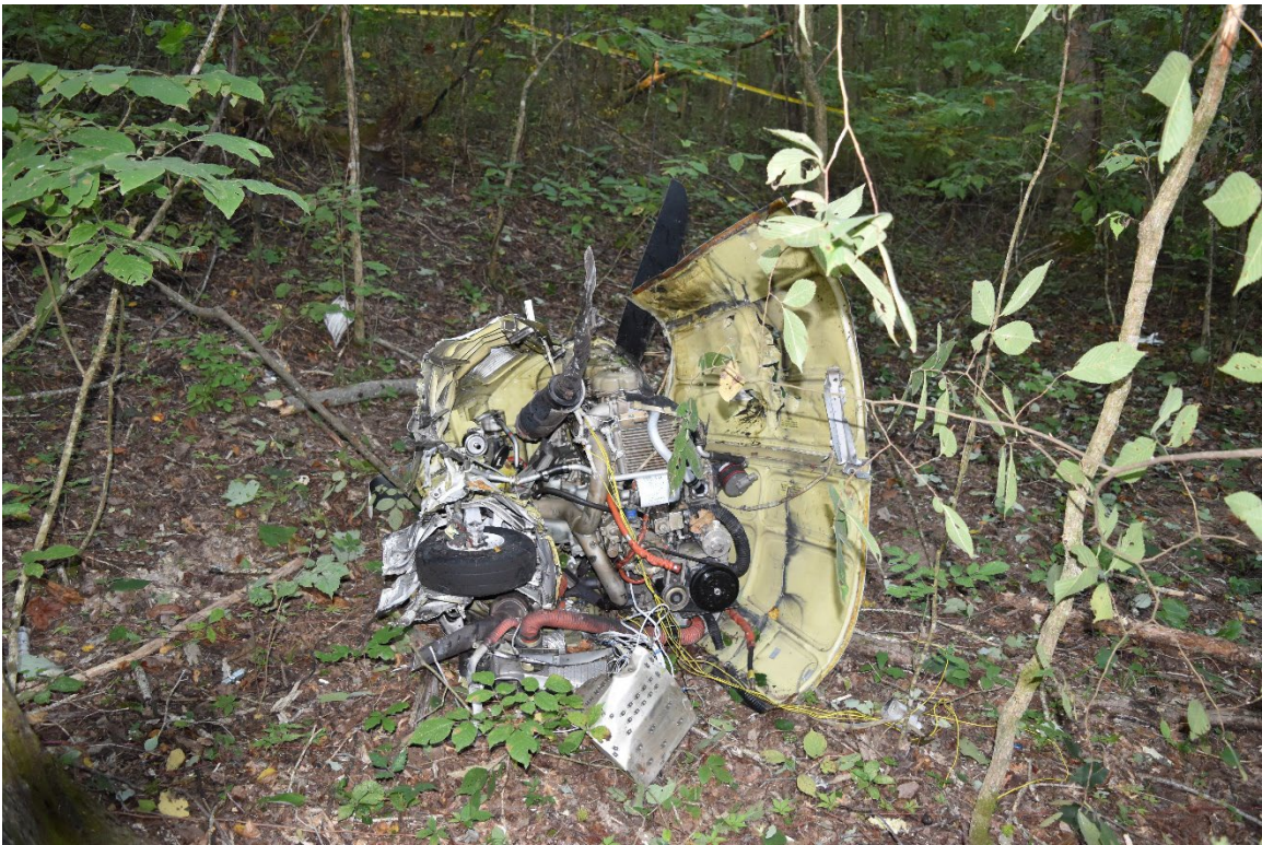
Photograph 3 – Accident Site – Separated engine and landing gear.
