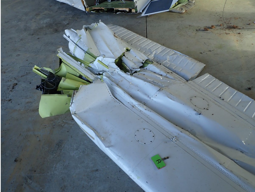
Photograph 6 – Accident airplane – Post-examination of right wing.
