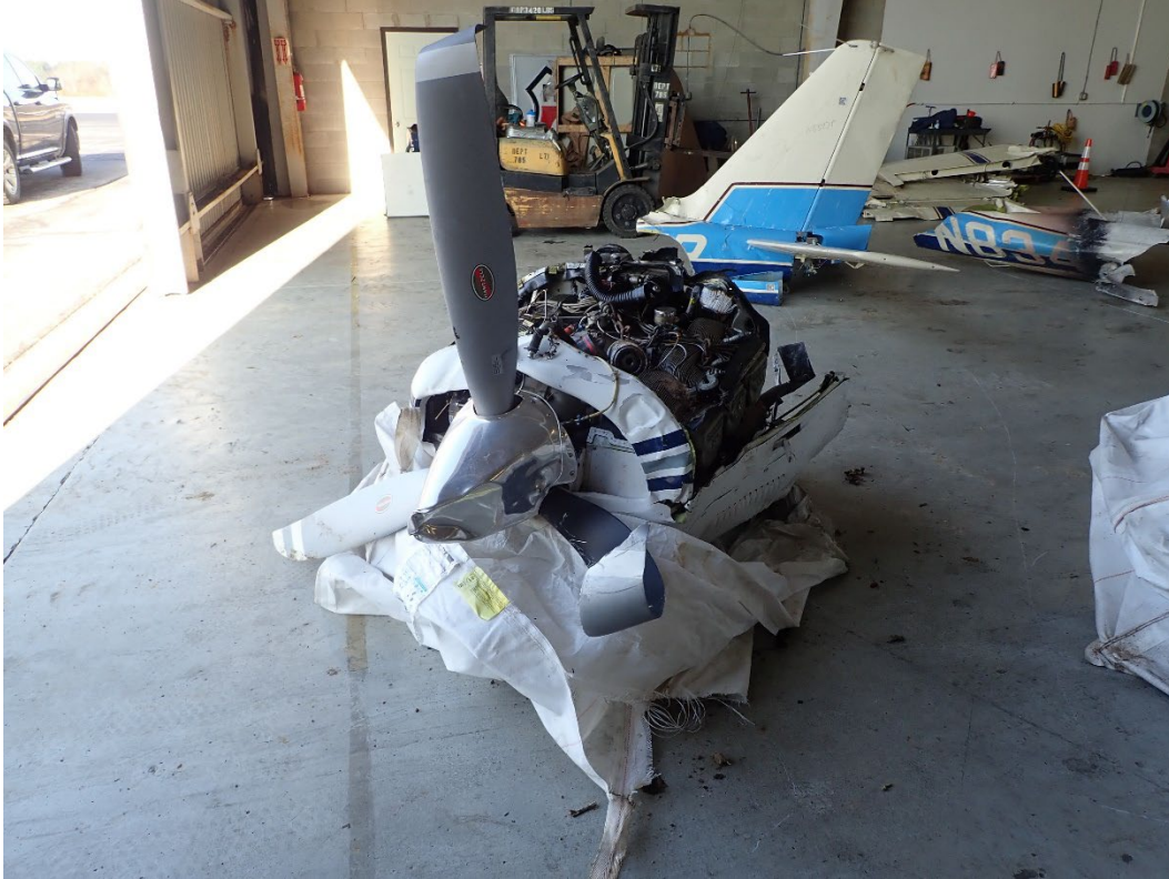
Photograph 10 – Accident airplane – Post-examination of engine and propeller.
