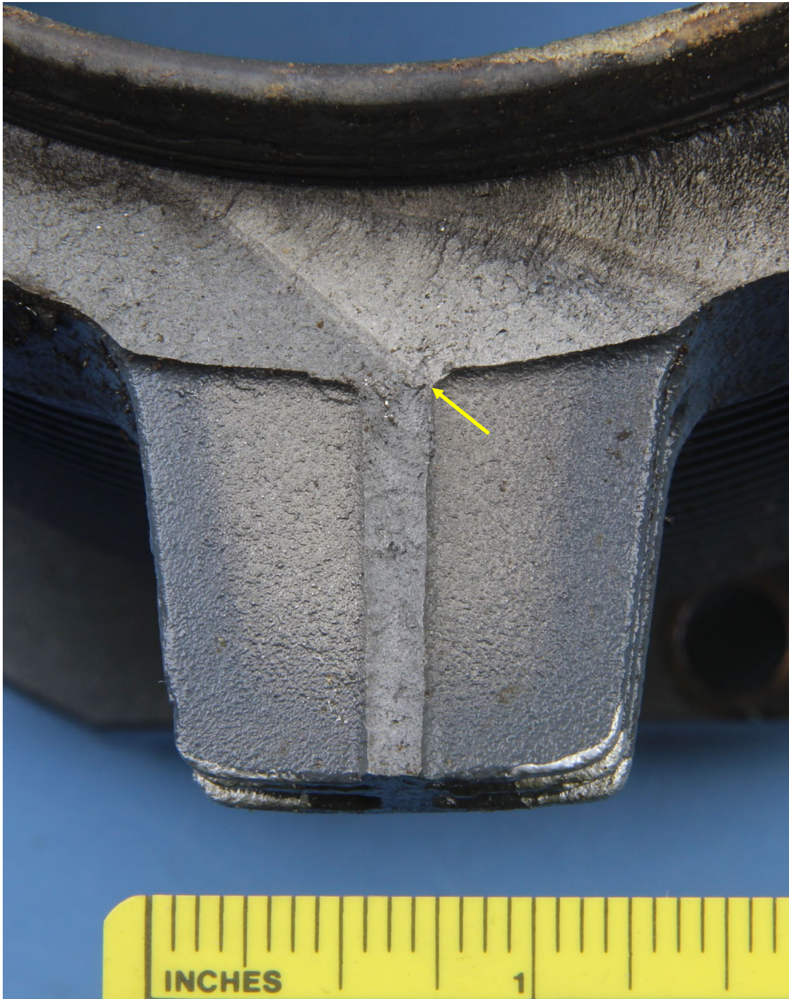
Figure 5: Close-up photo of the fracture surface on the bottom half of the separated cylinder. The yellow arrow points to the location of fatigue cracking initiation at the start of the fillet between the vertical stiffener and the circumferential outer wall of the cylinder.
