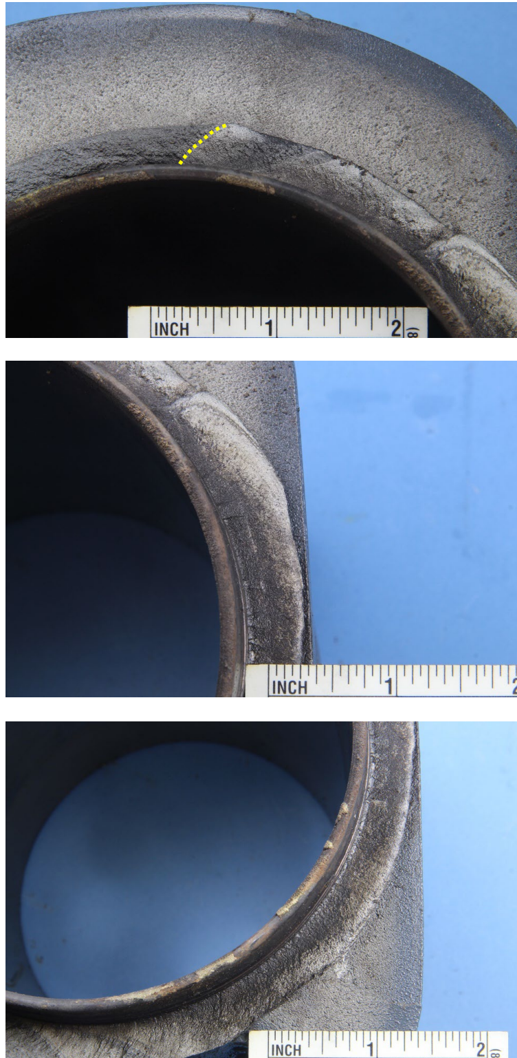
Figure 2: Close-up photos of the fatigue cracking on the fracture surface on the bottom half of the cylinder. The yellow dotted line in the top image indicates the interface where fatigue cracking ended, and overstress began.
