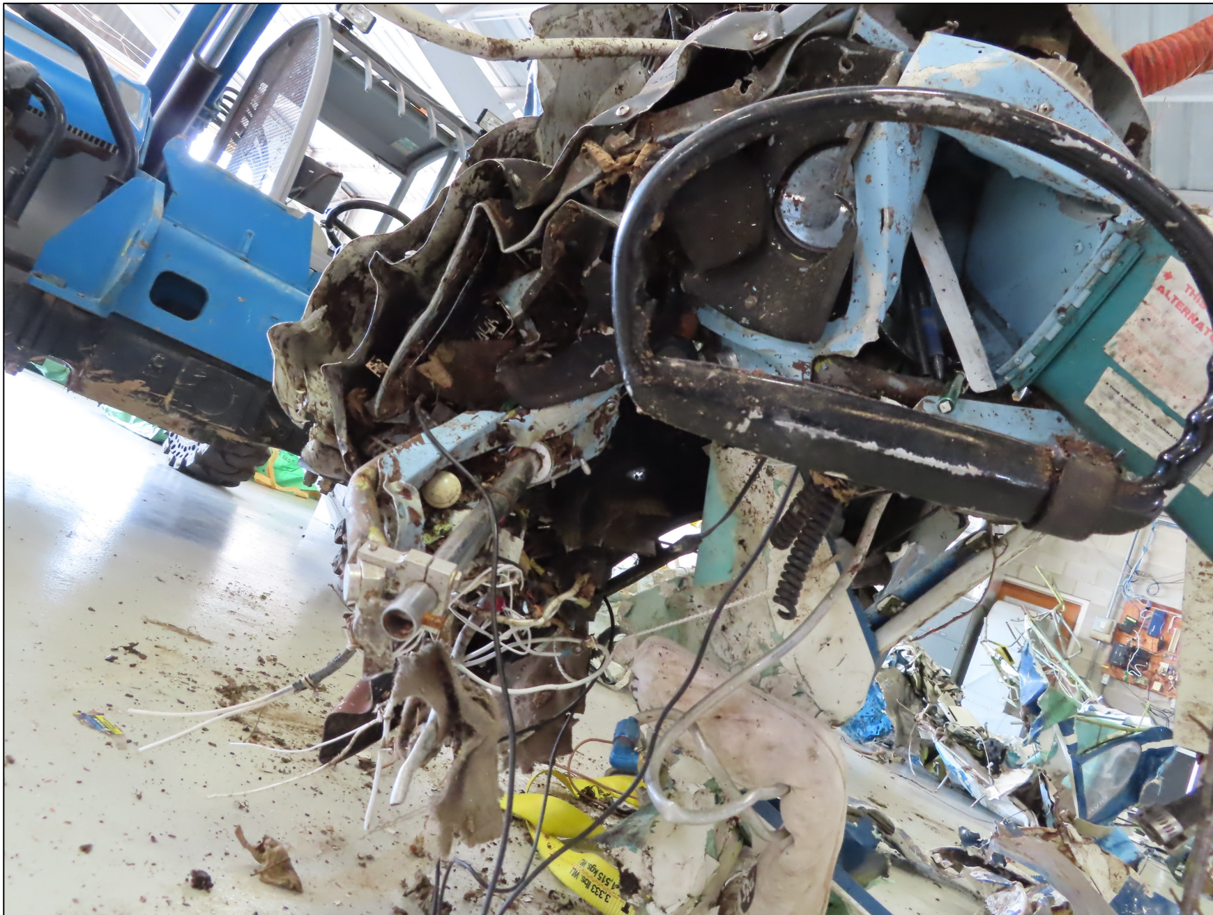
Photo 8 – View of the impact damaged flight controls and cockpit panel
