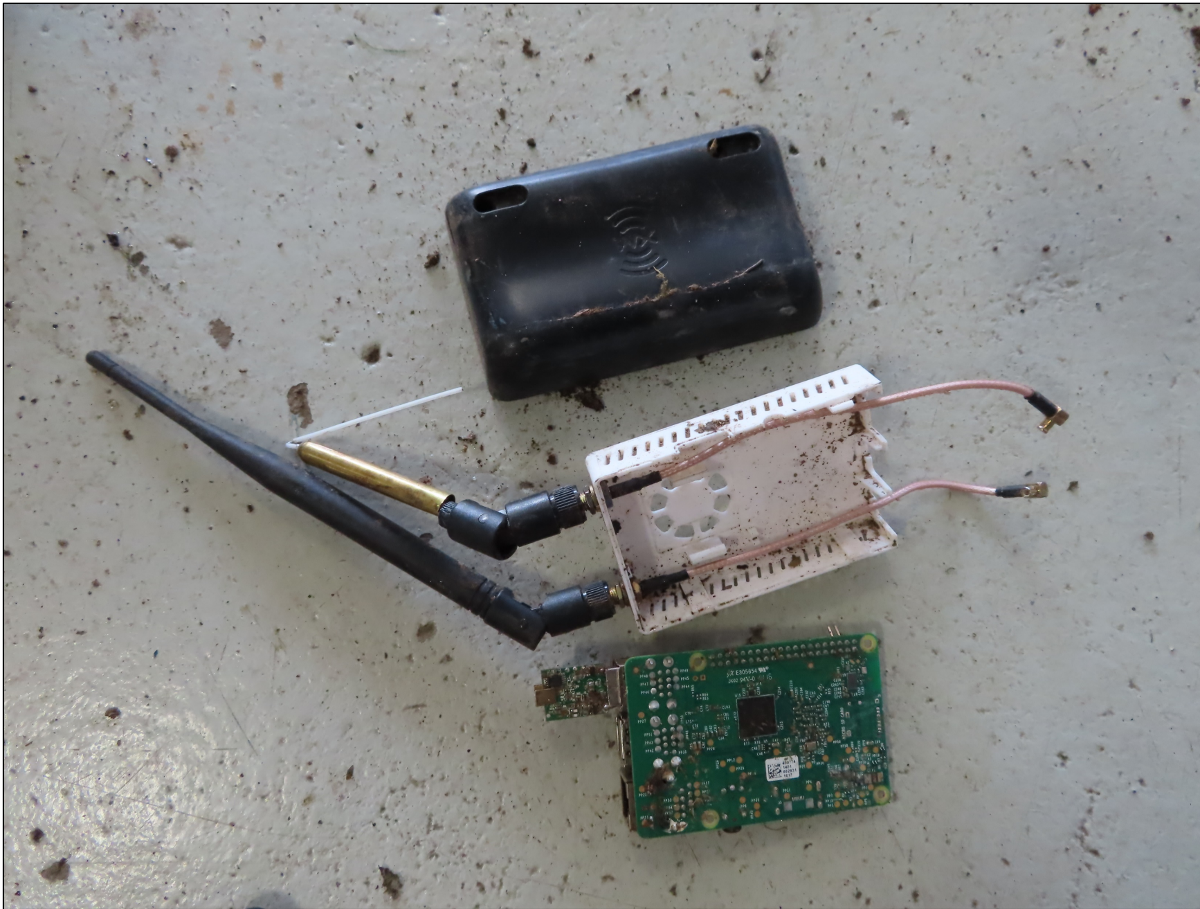
Photo 7 – View of the ADS-B Equipment located within the wreckage
