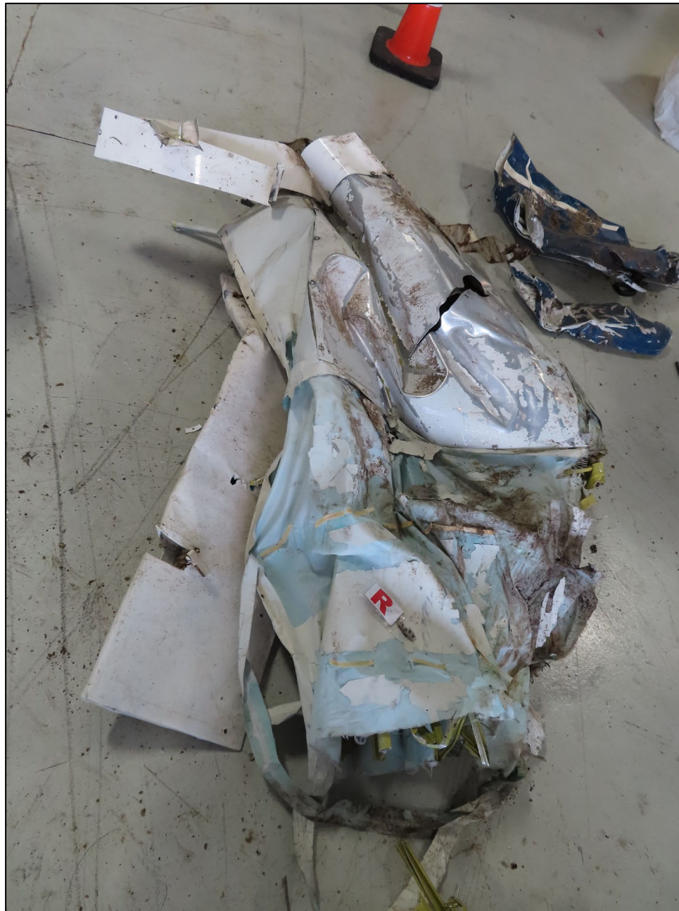
Photo 6 – View of the fragmented and impact damaged right wing
