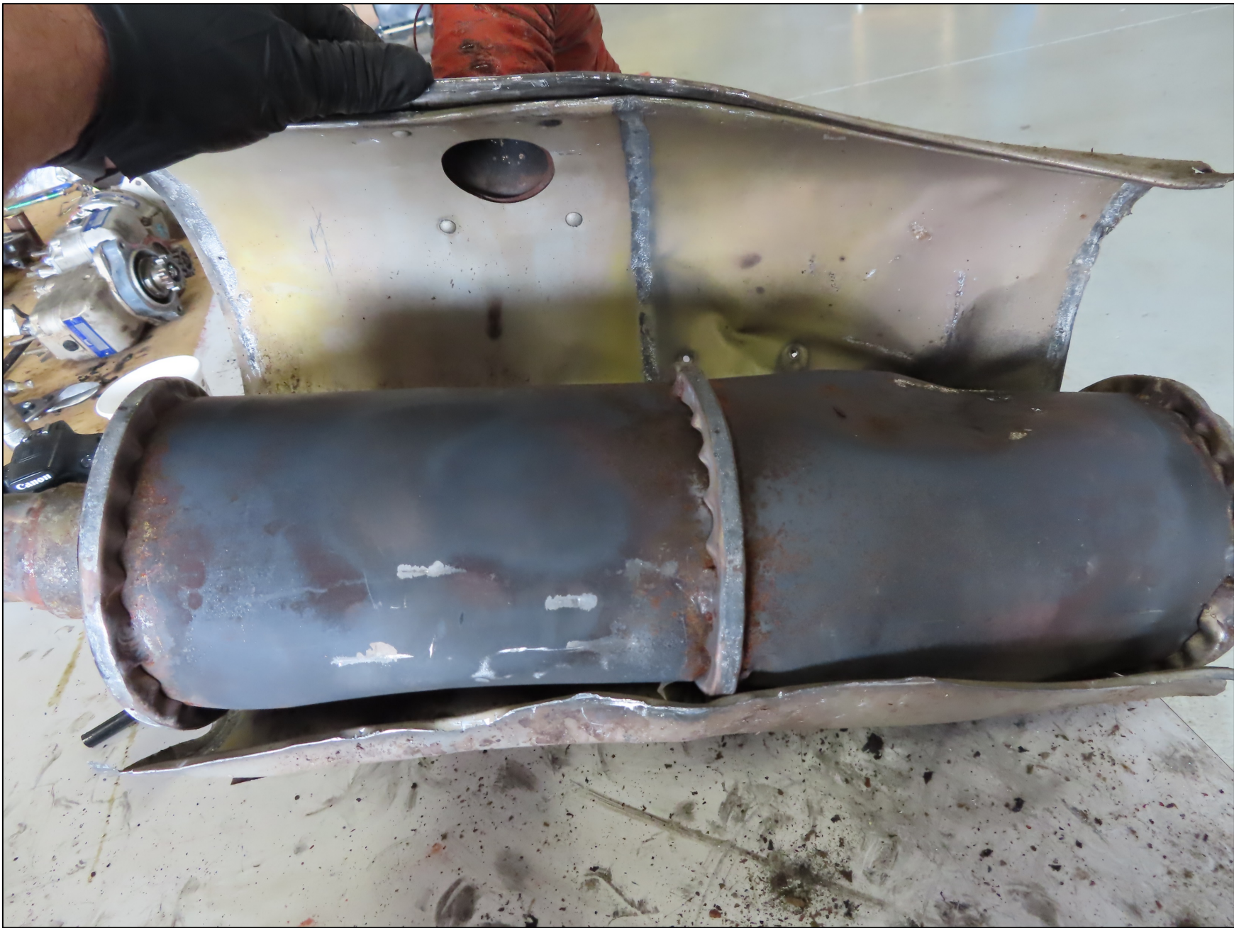
Photo 14 – View of the exhaust partially disassembled postaccident
