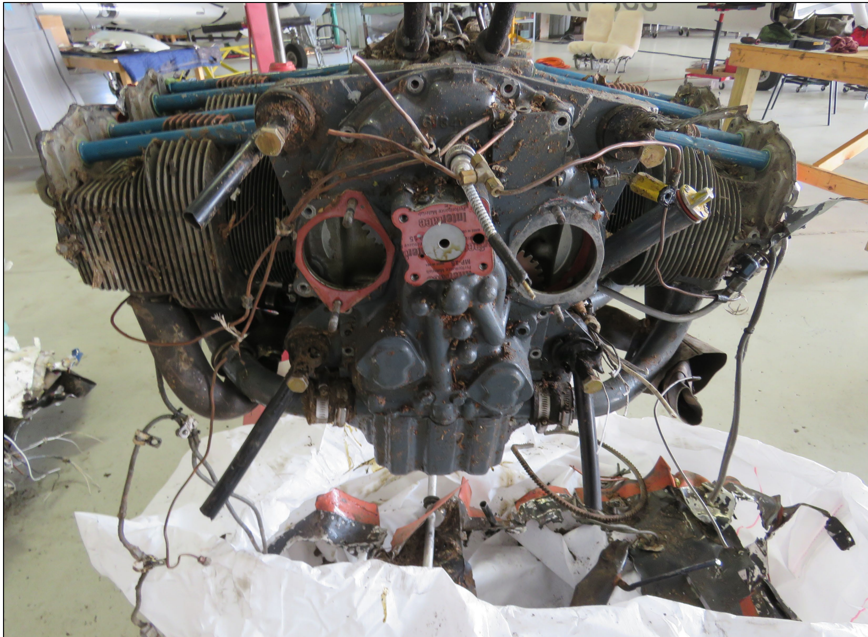
Photo 13 – View of the accessory section of the engine
