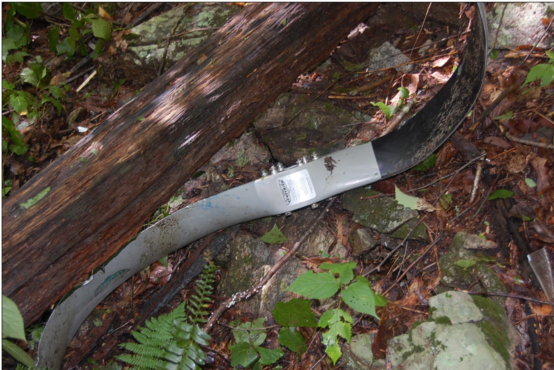
Photo 3 – View of the propeller at the accident site, separated from the engine (Photo Courtesy FAA)
