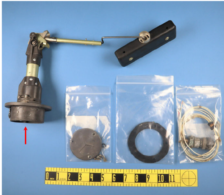
Figure 1.) As-received parts with red arrow pointing to the fuel transmitter assembly with float.
