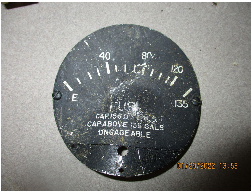
Figure 1: FAA Digital Photograph. View of the Separated Fuel Quantity Gauge Faceplate. Note the Separated Needle. No needle slap mark was noted.
