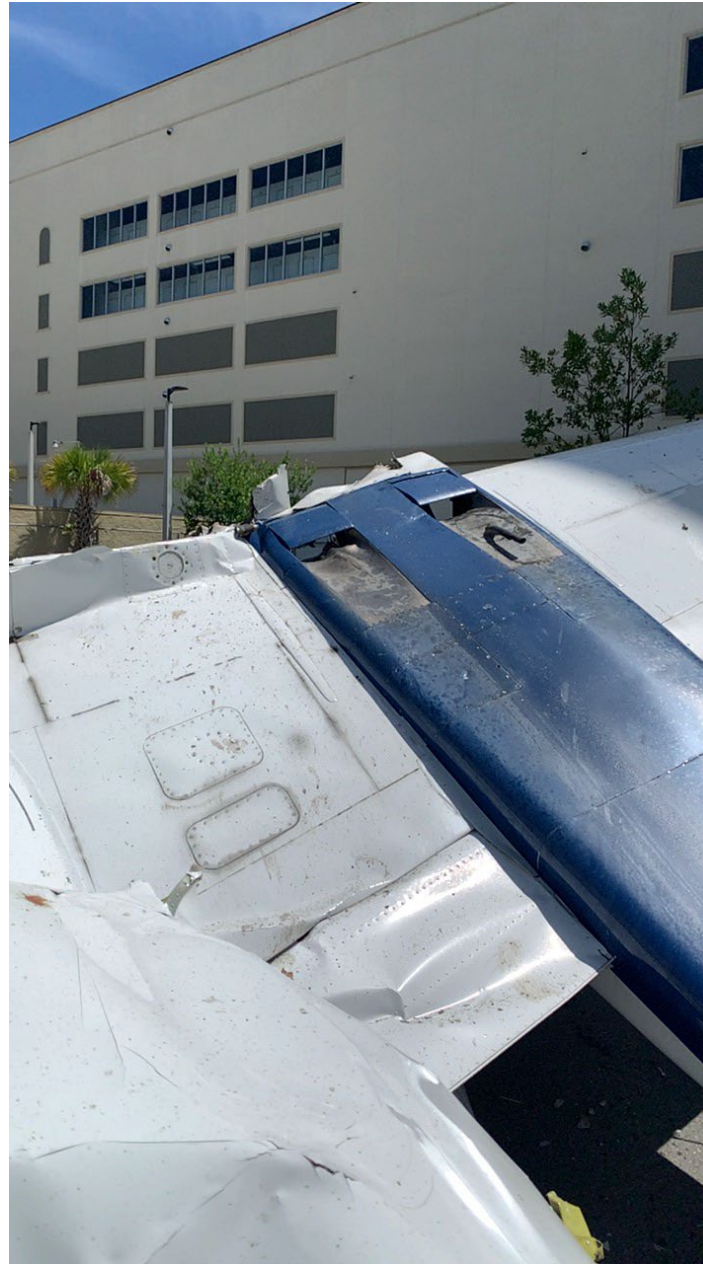
Photo 7 - FAA Digital Photograph. View of The Upper Portion of the Right Wing Showing the Fuel Filler Port. Note no Blue stains Aft of the Cap.
