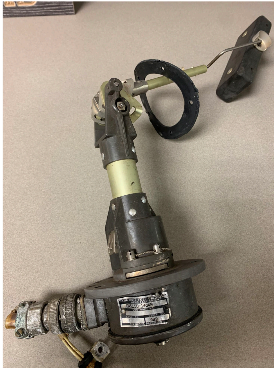
Photo 9 - FAA Digital Photograph. View of The Tank Unit, Part Number EA515B-1404M.
