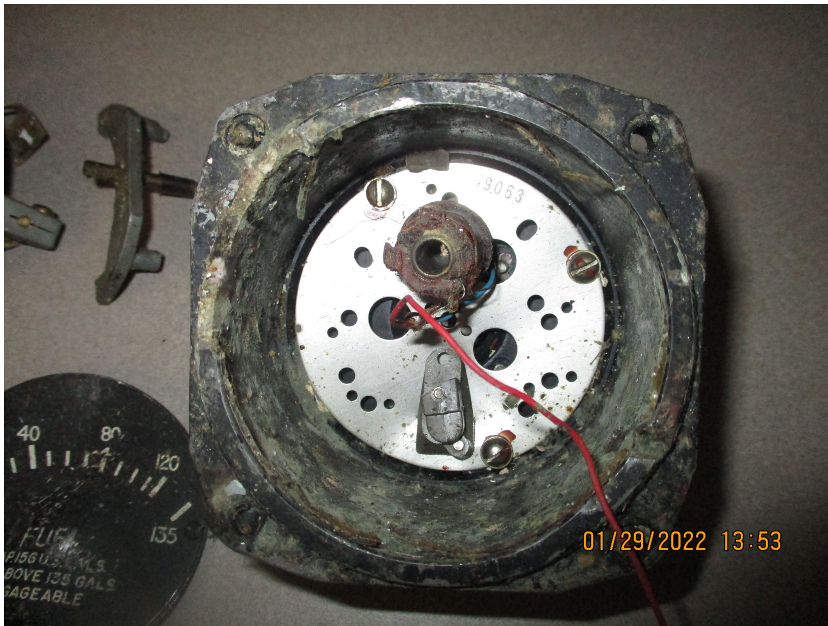
Photo 8 - FAA Digital Photograph. View of The Impact Damaged Fuel Quantity Gauge and Separated Faceplate. Note the Separated Needle.
