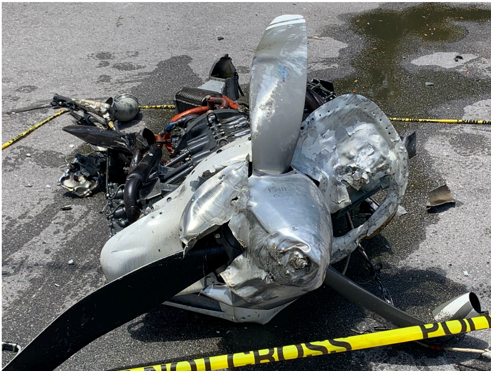
Photo 5 - FAA Digital Photograph. View Depicting the Right Propeller Assembly Attached to the Separated Engine Assembly.
