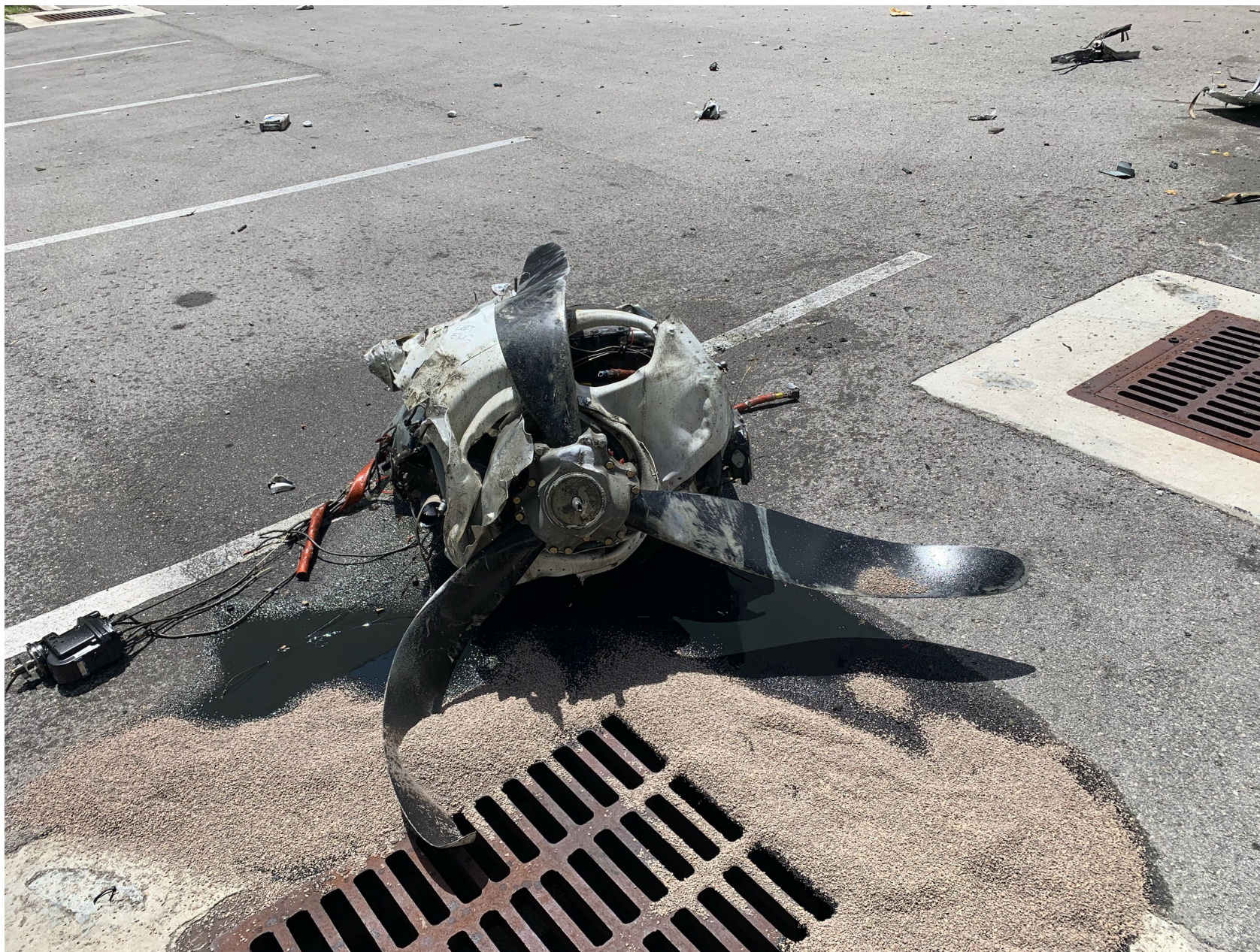
Photo 4 - FAA Digital Photograph. View Depicting the Left Propeller Assembly Attached to the Separated Engine Assembly. Note the Separated Cylinder, Piston, and Spinner.
