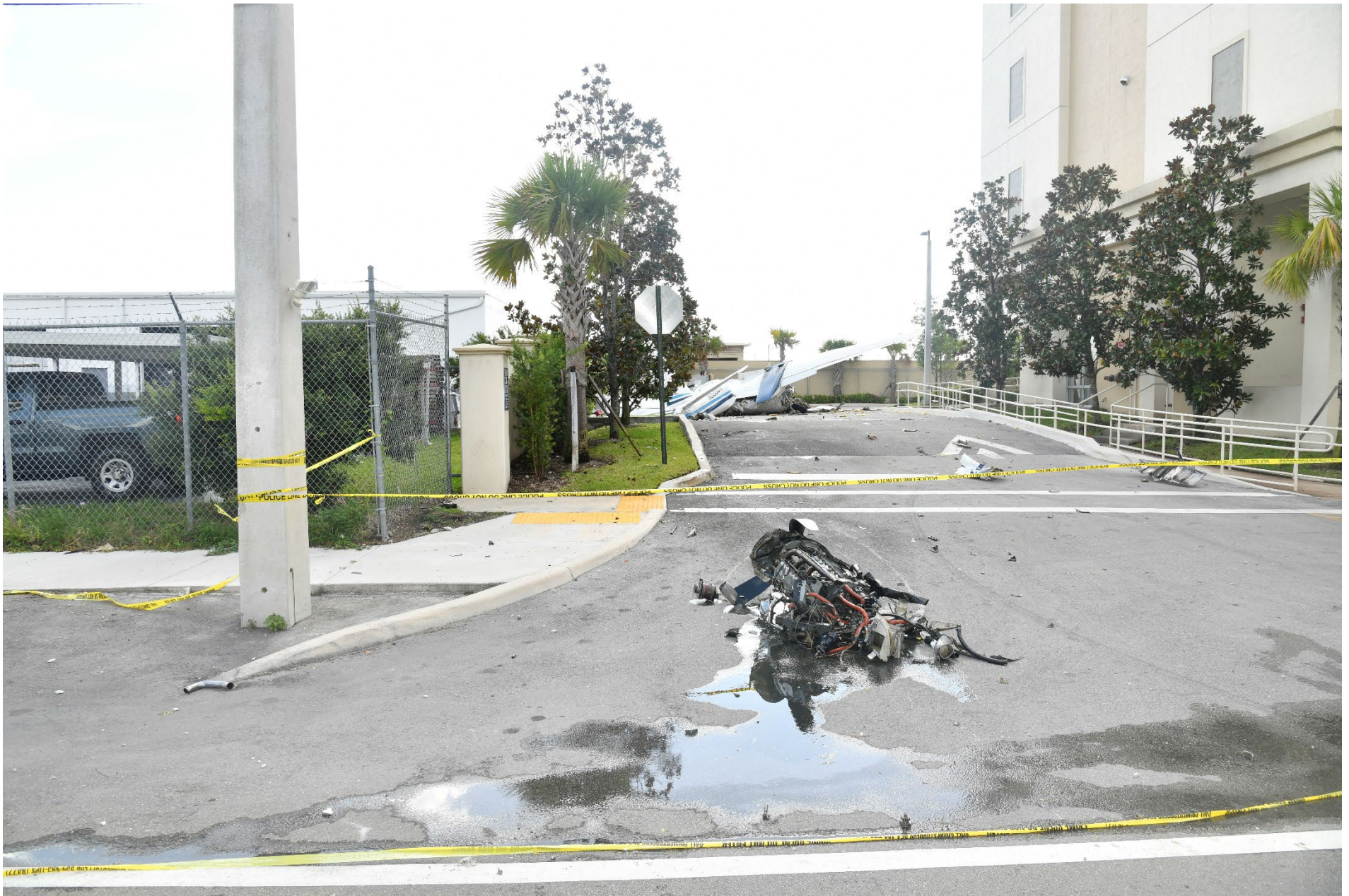
Photo 1 – Broward Sheriff’s Office Digital Photograph. View Depicting the Separated Right Engine with Attached Propeller in the Foreground and Right Rear Quartering View of the Main Wreckage in the Background.
