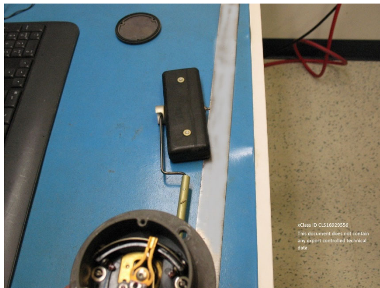
Figure 5: Bent in Float Arm
