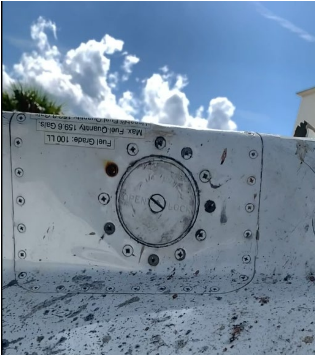
Figure 1: Screenshot From FAA Video Depicting Single Fuel Filler Port with Attached Fuel Cap.
