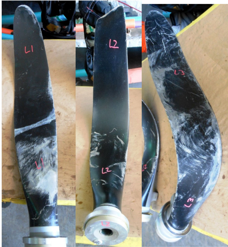
Photo #13 - Left propeller face side of blades
