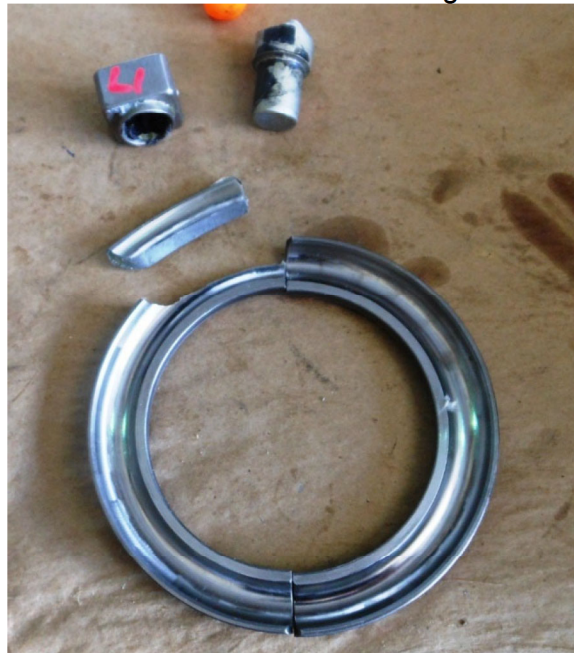
Photo #12 - L1 hub-side blade bearing race fracture
