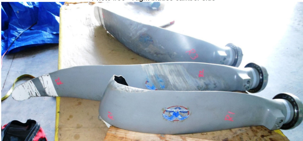
Photo #33 - Right blades camber side
