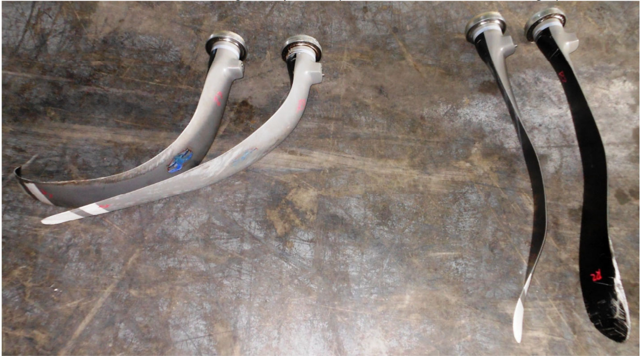
Photo #1 - Blade damage comparison (L2-R3 on left and L1-R2 on right)
