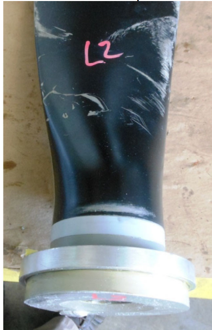
Photo #14 - L2 blade shank impact mark on face side
