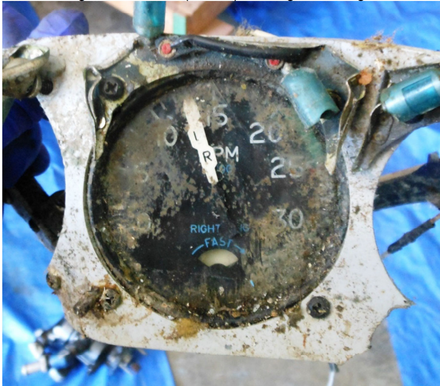
Photo #2 - Engine tachometer (electric) showing left and right ~1300 RPM
