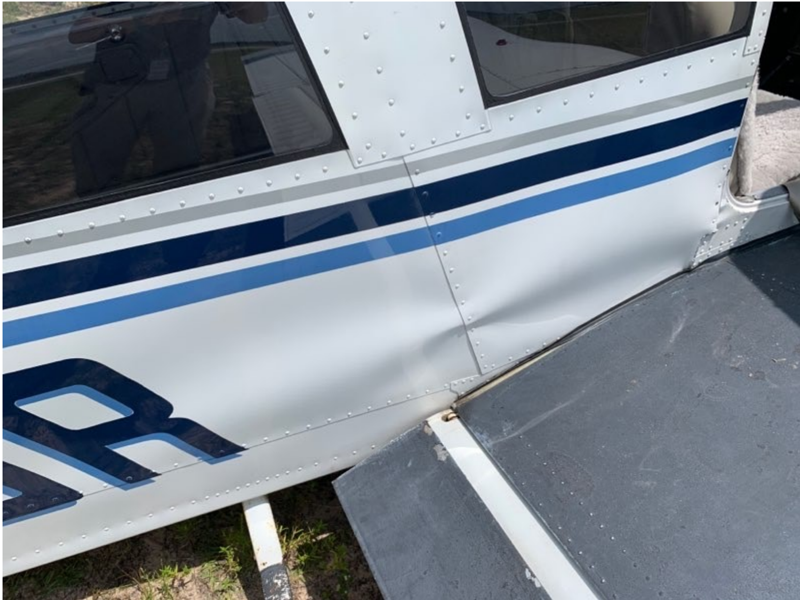
Photo 2 – View of fuselage damage. (Courtesy of Airport Manager)
