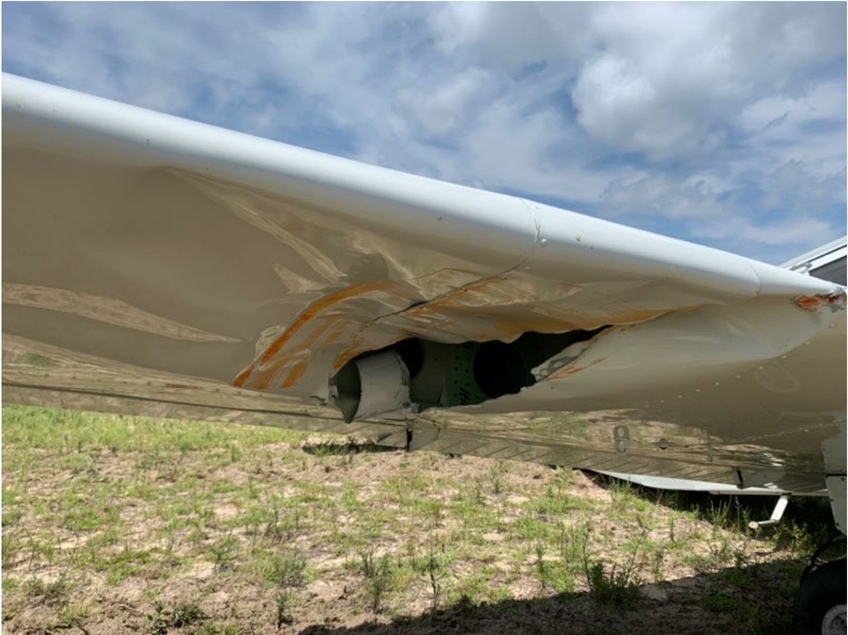
Photo 1 – View of right wing damage. (Courtesy of Airport Manager)
